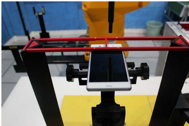
**Picture 2: EUT Positioning for RF**
