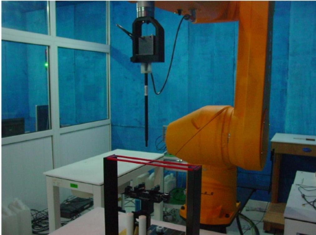
**Picture A1: HAC RF System Layout**
