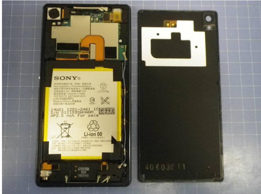
Mobile Phone Disassembly and Inbuilt Battery
