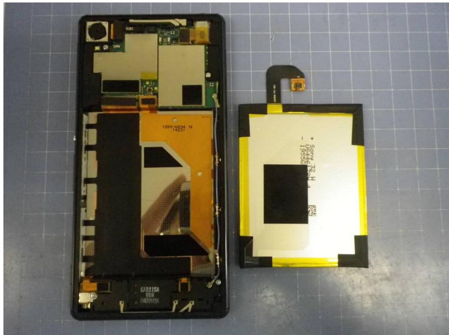
Mobile Phone Disassembly and Inbuilt Battery
