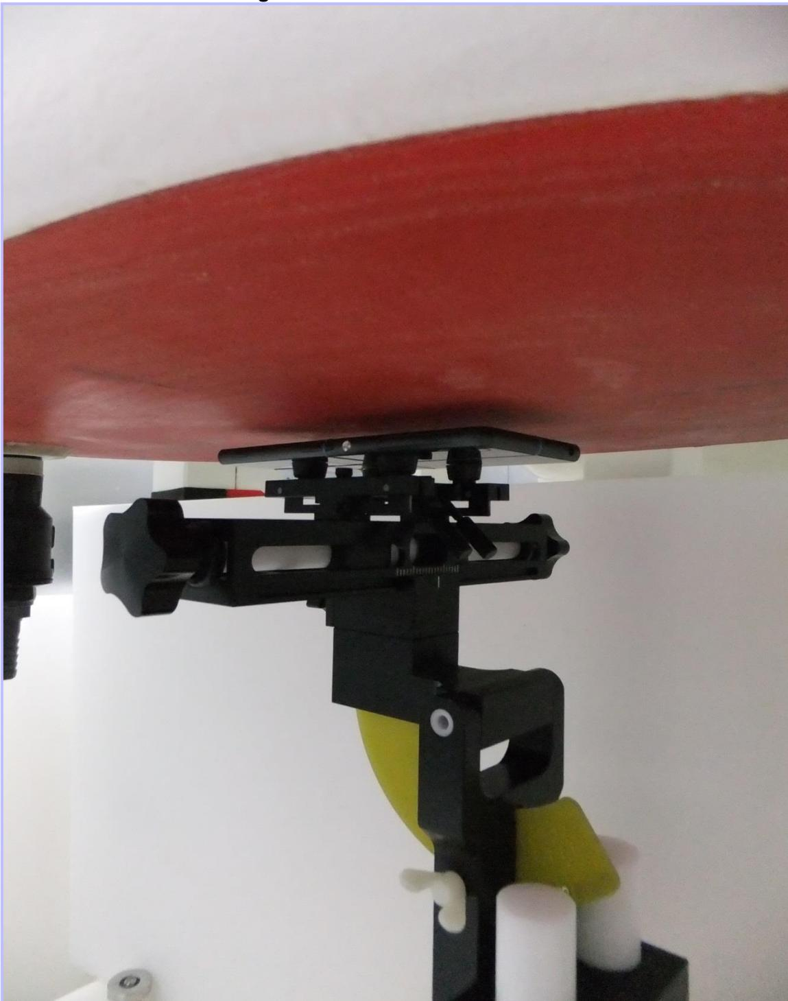
**003: Left Hand Side of the EUT Facing Phantom at 10mm**
