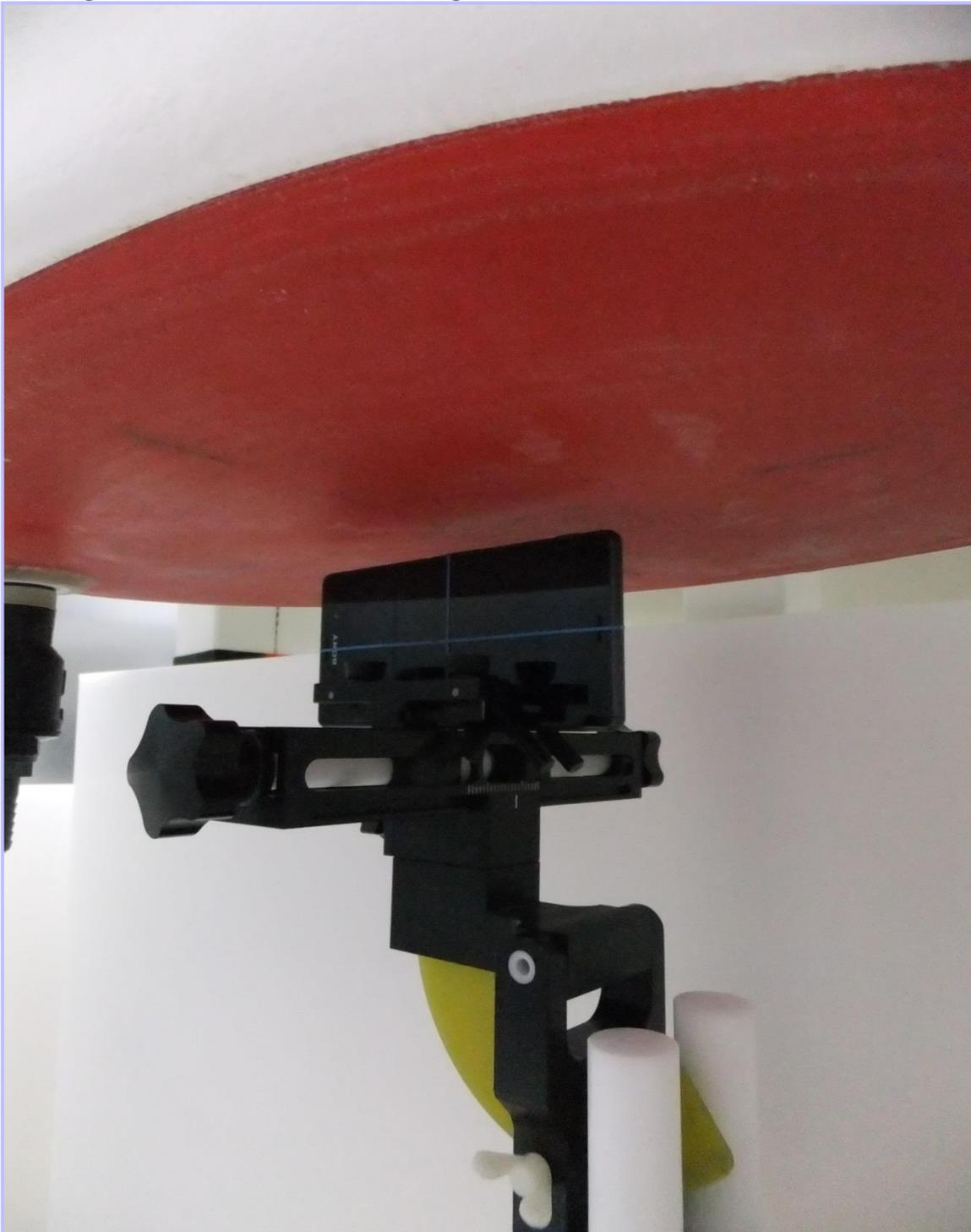
**005: Bottom of the EUT Facing Phantom at 10mm**
