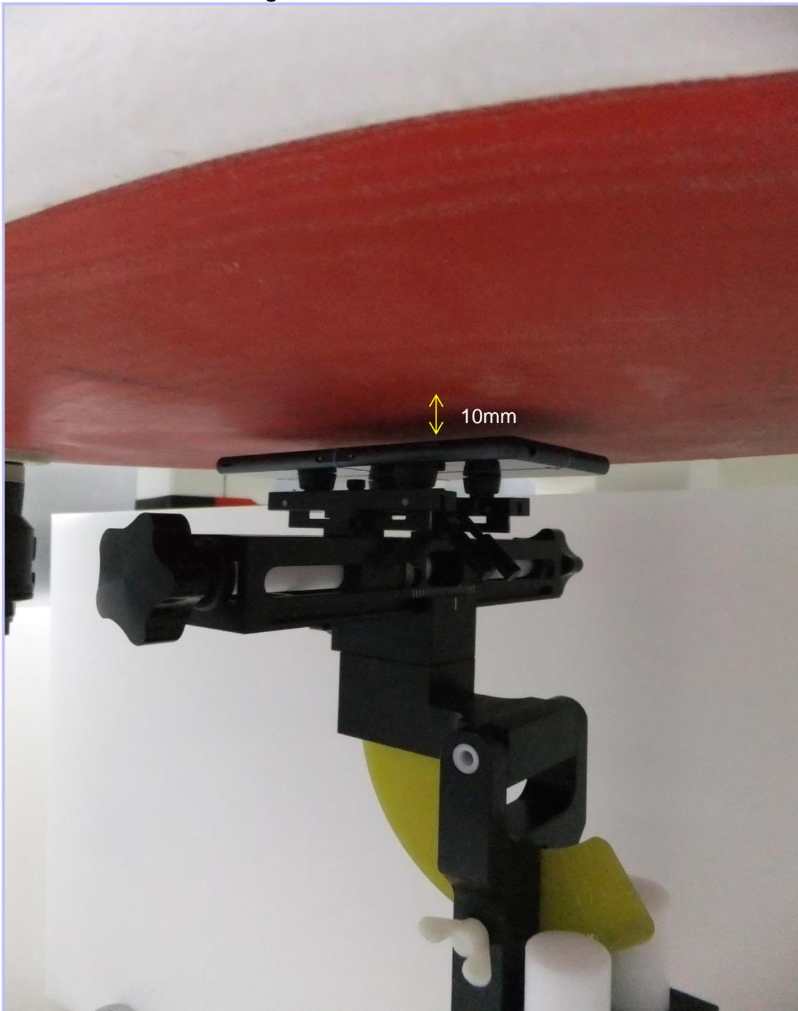
**002: Back of the EUT Facing Phantom at 10mm**
