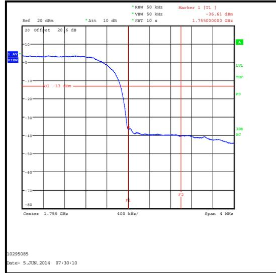
**Transmitter Radiated Emissions at Band Edges (continued)**
