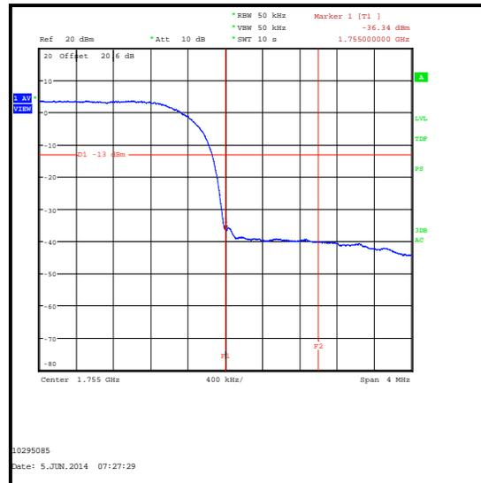
**Transmitter Radiated Emissions at Band Edges (continued)**
