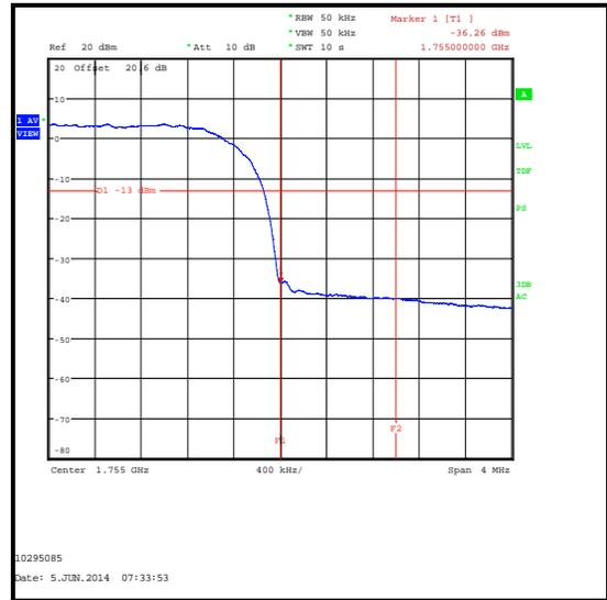
**Transmitter Radiated Emissions at Band Edges (continued)**
