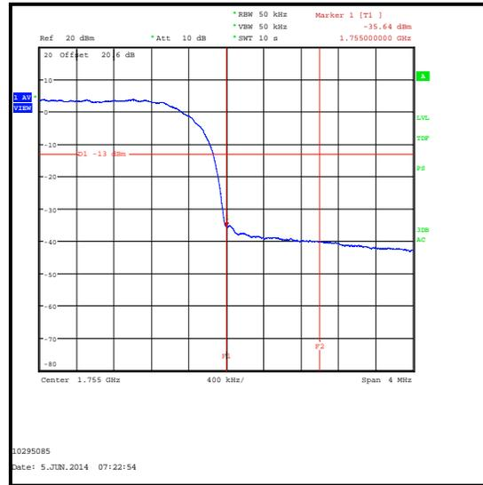
**Transmitter Radiated Emissions at Band Edges (continued)**
