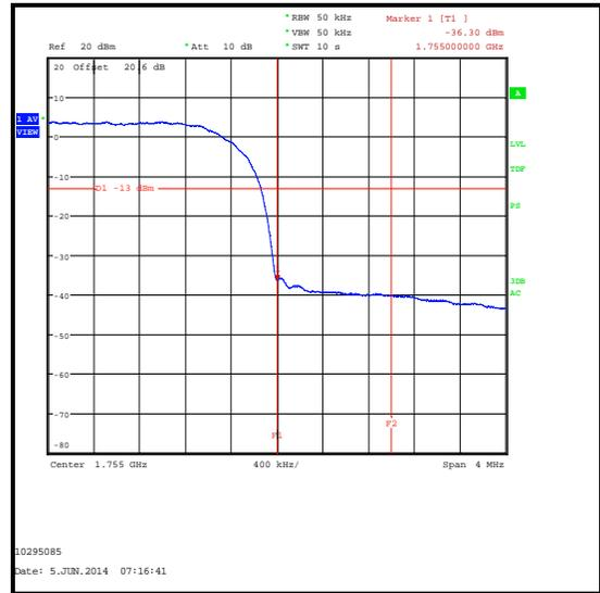
**Transmitter Radiated Emissions at Band Edges (continued)**
