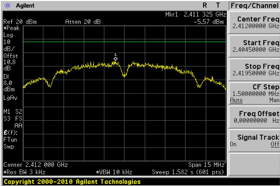
Power Spectral Density Test Plot (CH-Mid)
