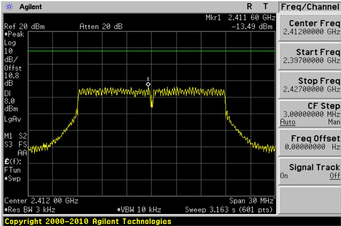
Power Spectral Density Test Plot (CH-Mid)
