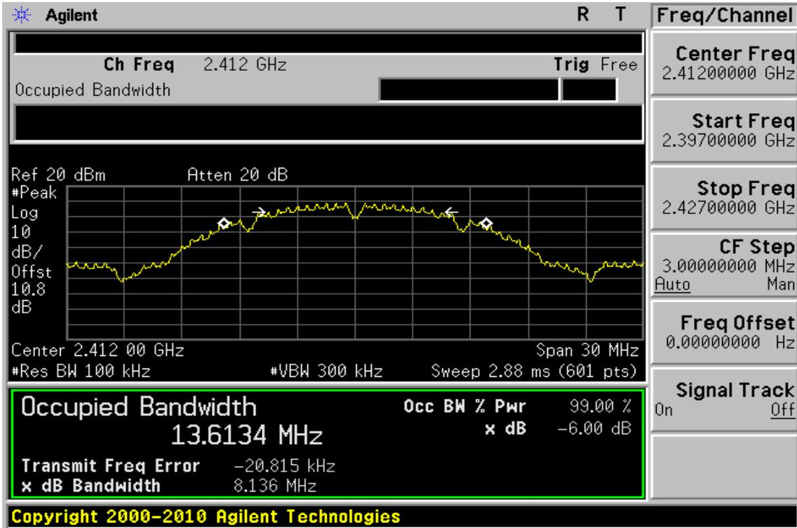
6dB Band Width Test Data CH-Mid
