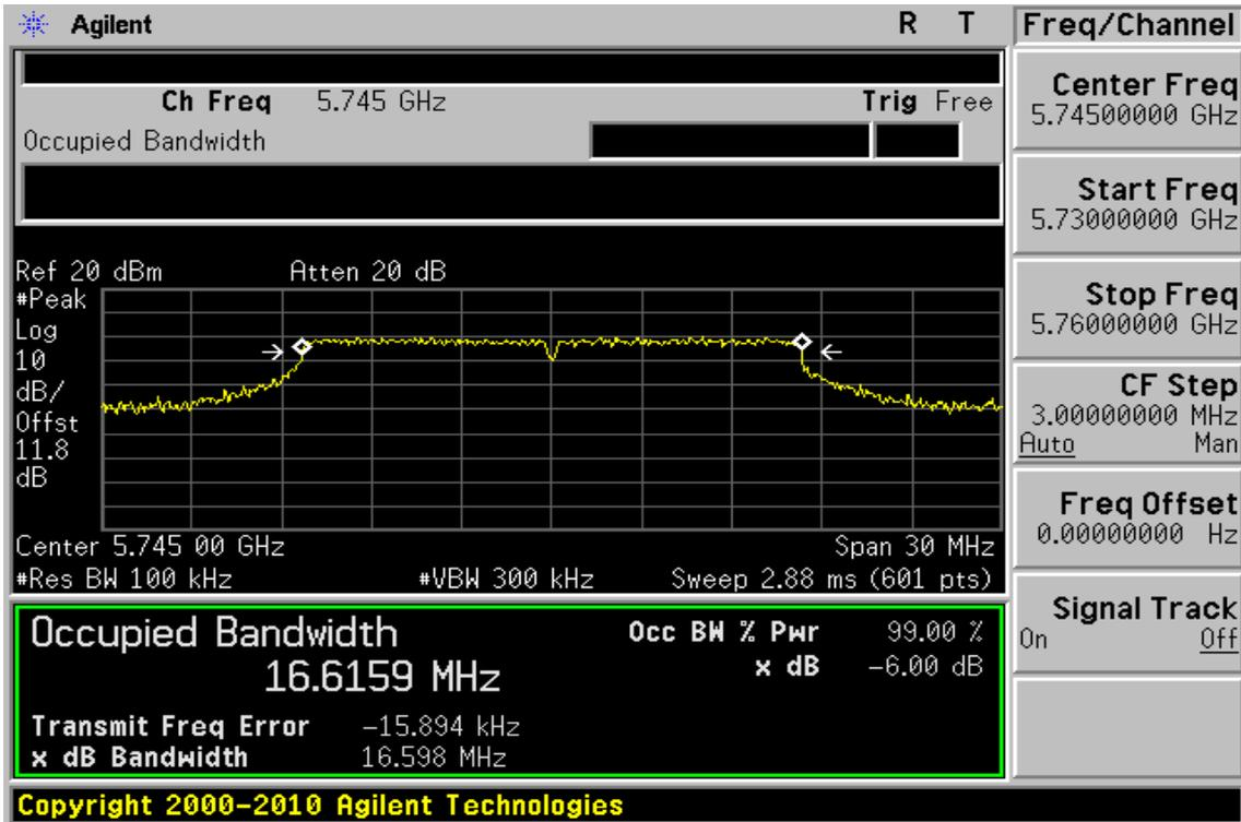
6dB Band Width Test Data CH-Mid
