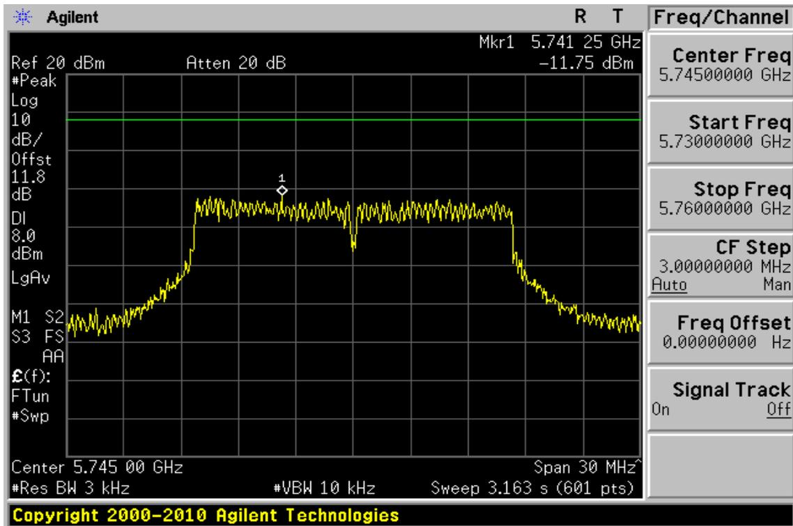
Power Spectral Density Test Plot (CH-Mid)
