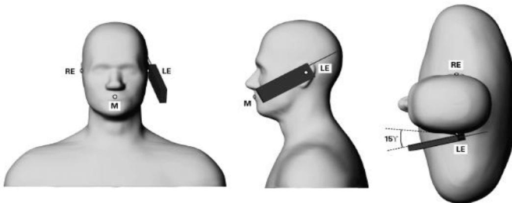
Phone position 2, "tilted position." The reference points for the right ear (RE), left ear (LE) and mouth (M), which define the reference plane for phone positioning.
