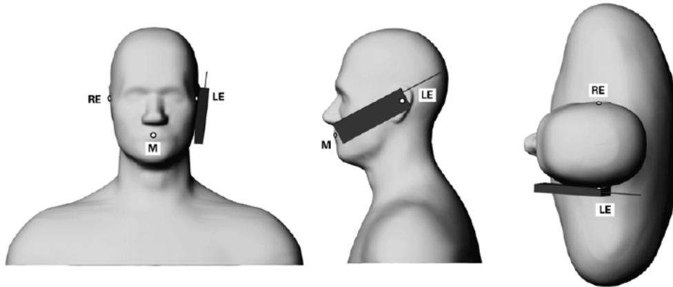
Phone position 1, "cheek" or "touch" position. The reference points for the right ear (RE), left ear (LE) and mouth (M), which define the reference plane for phone positioning.
