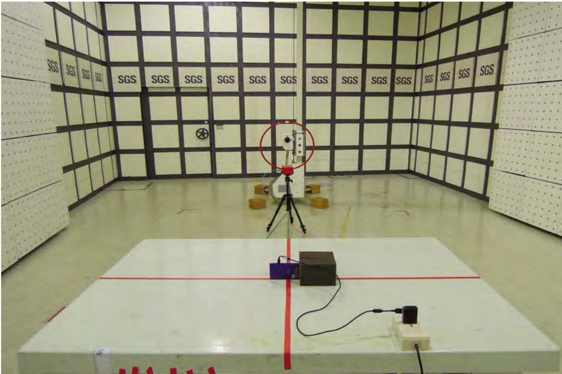
**Antenna with V polarization**
