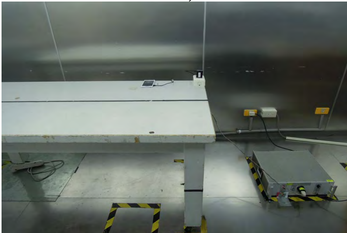
AC Power-line Conducted Emission Set up Photo (Adapter Model number: EP880)
