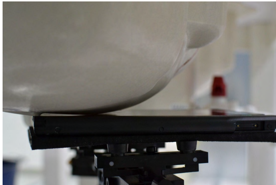
SAR Test Setup Photo 2 – Right Cheek with L-Battery Cover
