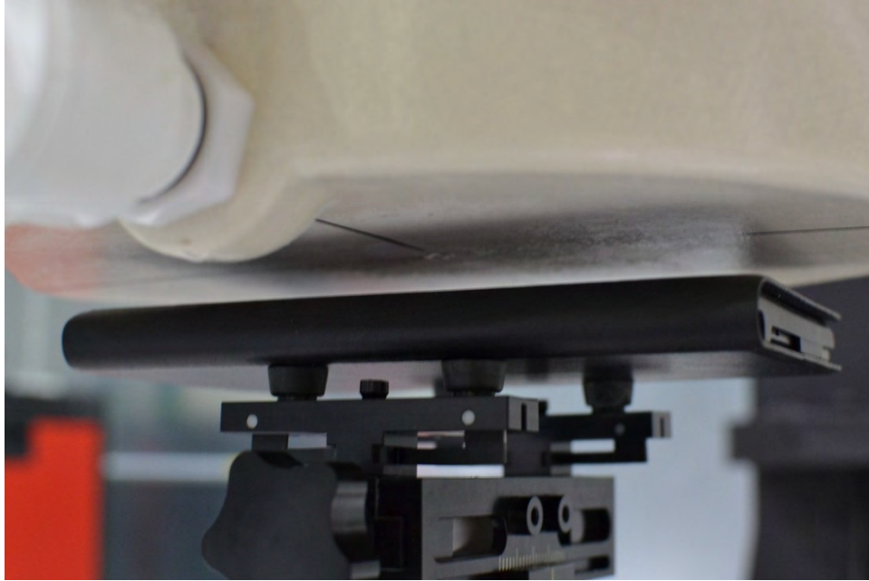
SAR Test Setup Photo 11 – Back Side at 1.5 cm with L-Battery Cover
