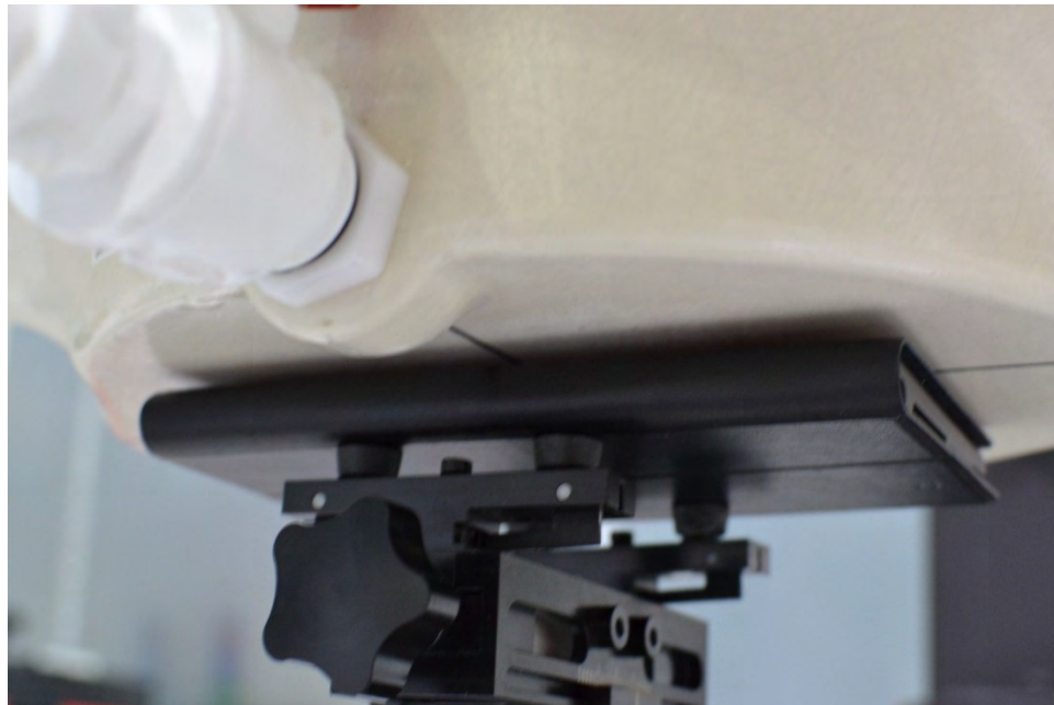
SAR Test Setup Photo 20 – Back Side at 0.3 cm with L-Battery Cover
