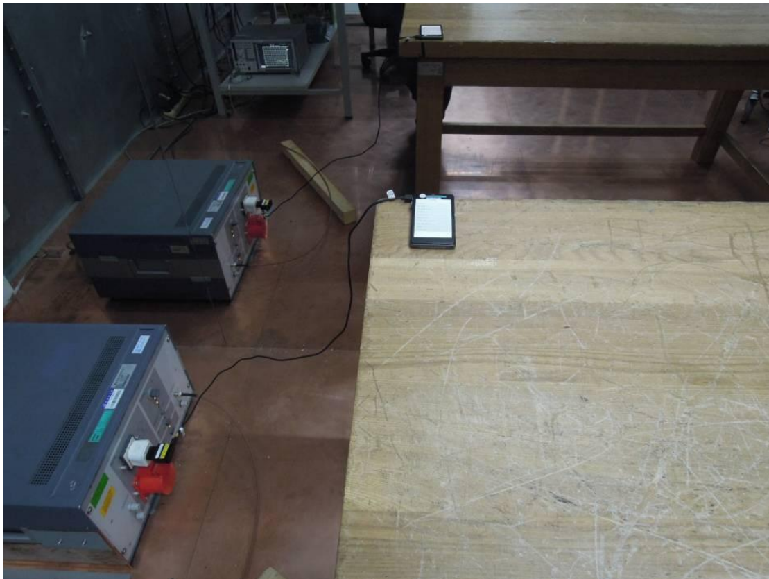
Layout of AC Powerline Conducted Emission – FCC 2.4G/5G
