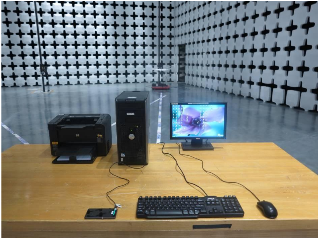
Layout of AC Radiated Spurious Emission Test
