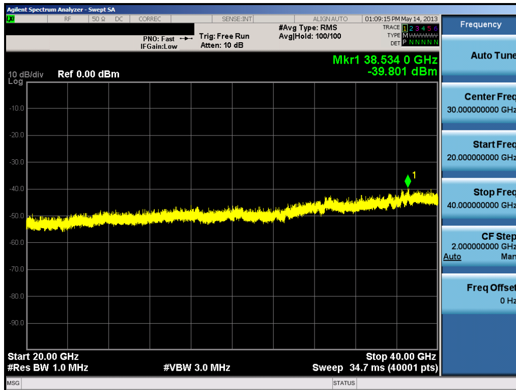
Plot 6-60. Conducted Spurious Plot (802.11a – Ch. 157)
