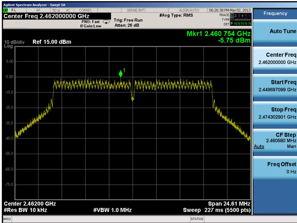
Plot 6-24. Power Spectral Density Plot (802.11g – Ch. 11)
