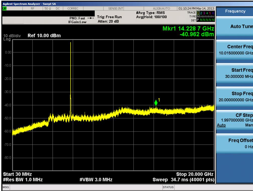
Plot 6-59. Conducted Spurious Plot (802.11a – Ch. 157)
