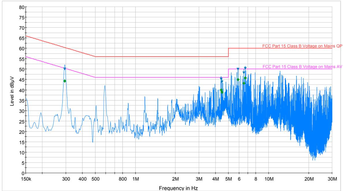
— FCC Part 15 Class B Voltage on Mains QP.LimitLine — FCC Part 15 Class B Voltage on Mains AV.LimitLine — Preview Result 1-PK+
