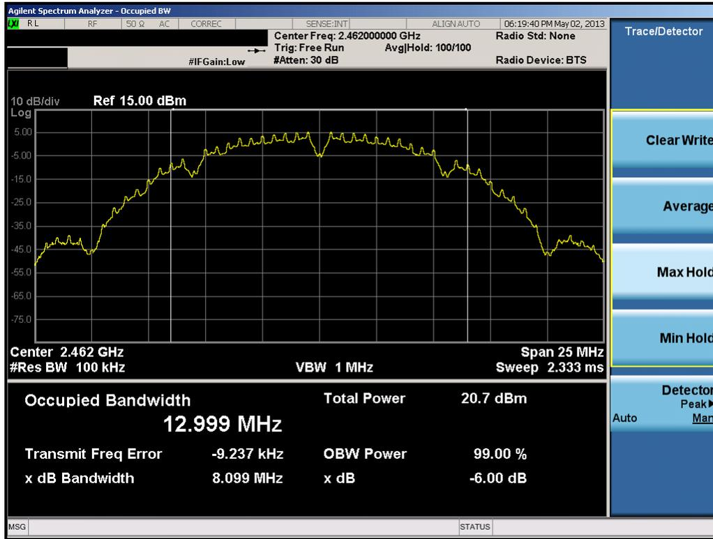
Plot 6-3. 6dB Bandwidth Plot (802.11b – Ch. 11)
