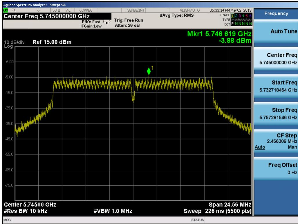
Plot 6-28. Power Spectral Density Plot (802.11a – Ch. 149)
