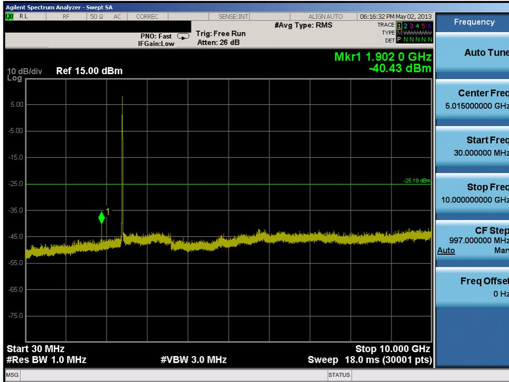
Plot 6-51. Conducted Spurious Plot (802.11b – Ch. 1)
