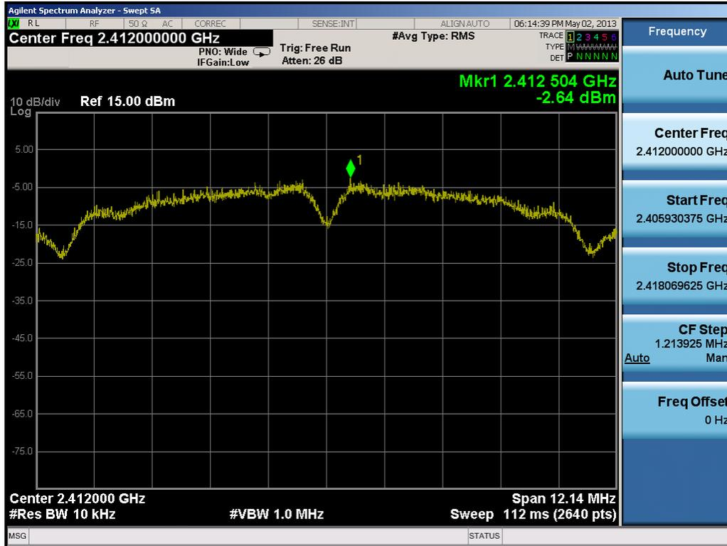
Plot 6-19. Power Spectral Density Plot (802.11b – Ch. 1)
