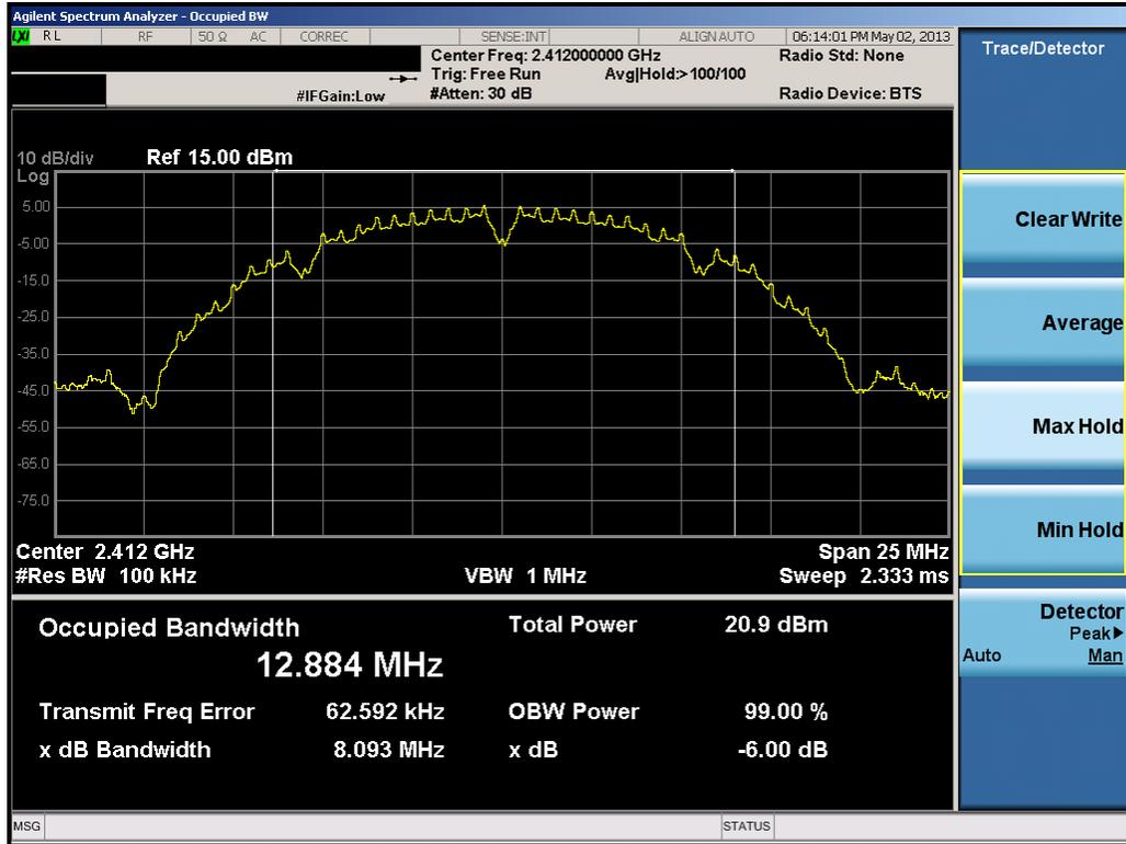
Plot 6-1. 6dB Bandwidth Plot (802.11b – Ch. 1)
