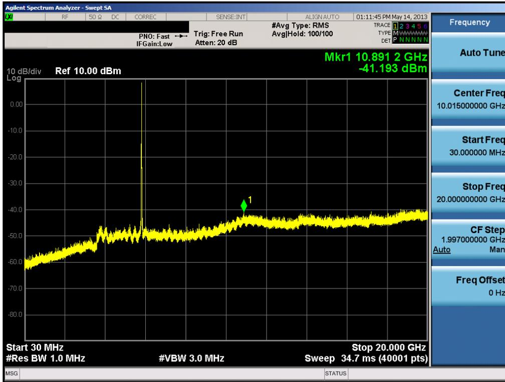
Plot 6-61. Conducted Spurious Plot (802.11a – Ch. 165)
