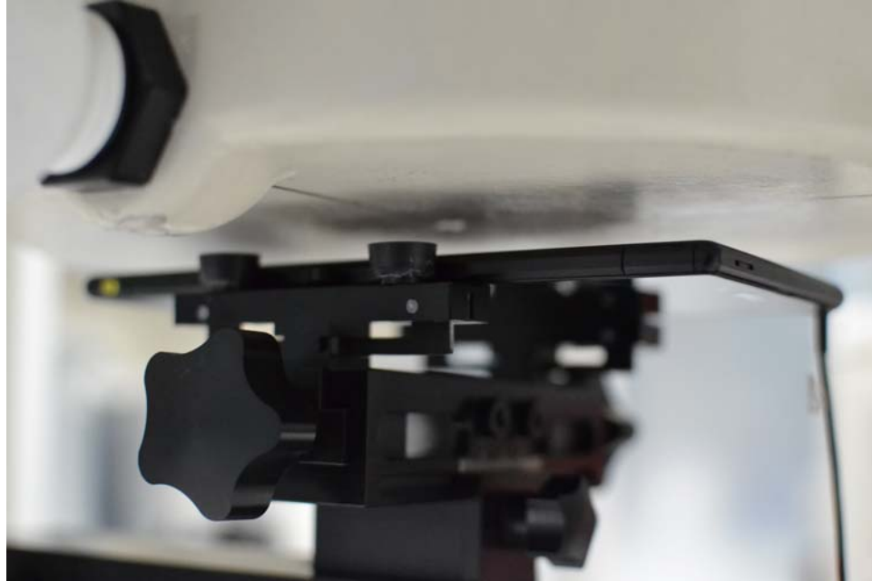
SAR Test Setup Photo 13 – Back Side with Headset at 1.5 cm
