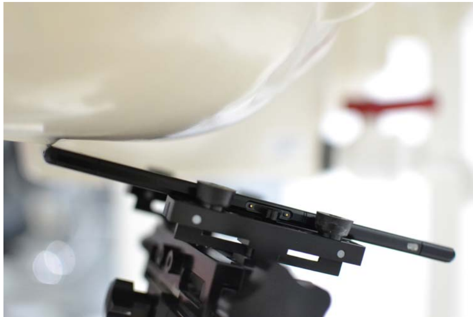
SAR Test Setup Photo 2 – Right Tilt
