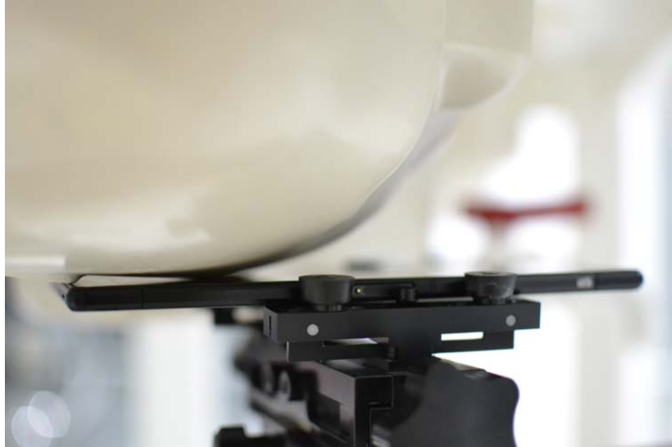
SAR Test Setup Photo 1 – Right Cheek
