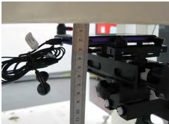
Fig.7 EUT front side with headset (MH410C) to flat phantom
