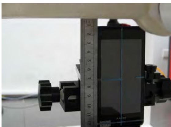
Fig.13 EUT bottom to flat phantom
