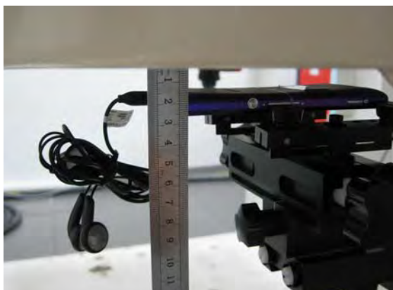
Fig.8 EUT back side with headset (MH410C) to flat phantom
