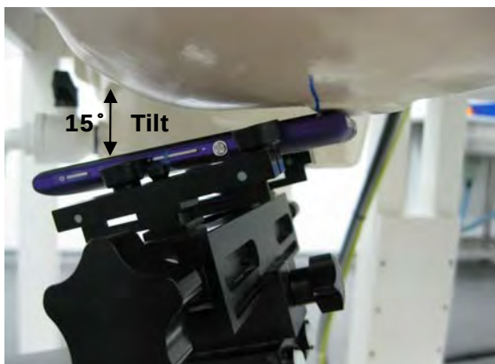
Fig.6 Left Head Section / Ear-Tilt Position(15°)
