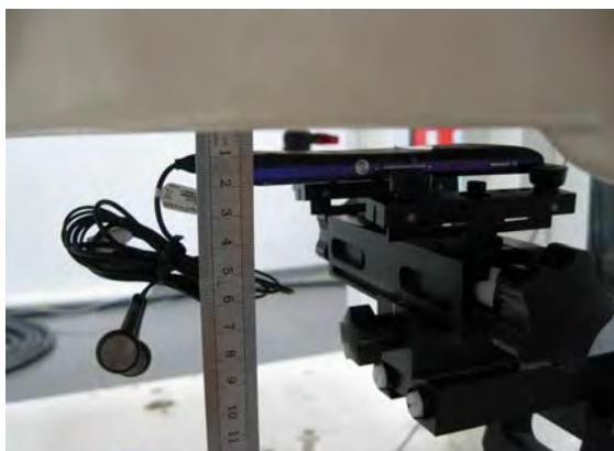
Fig.11 EUT back with headset (MH410C) to flat phantom
