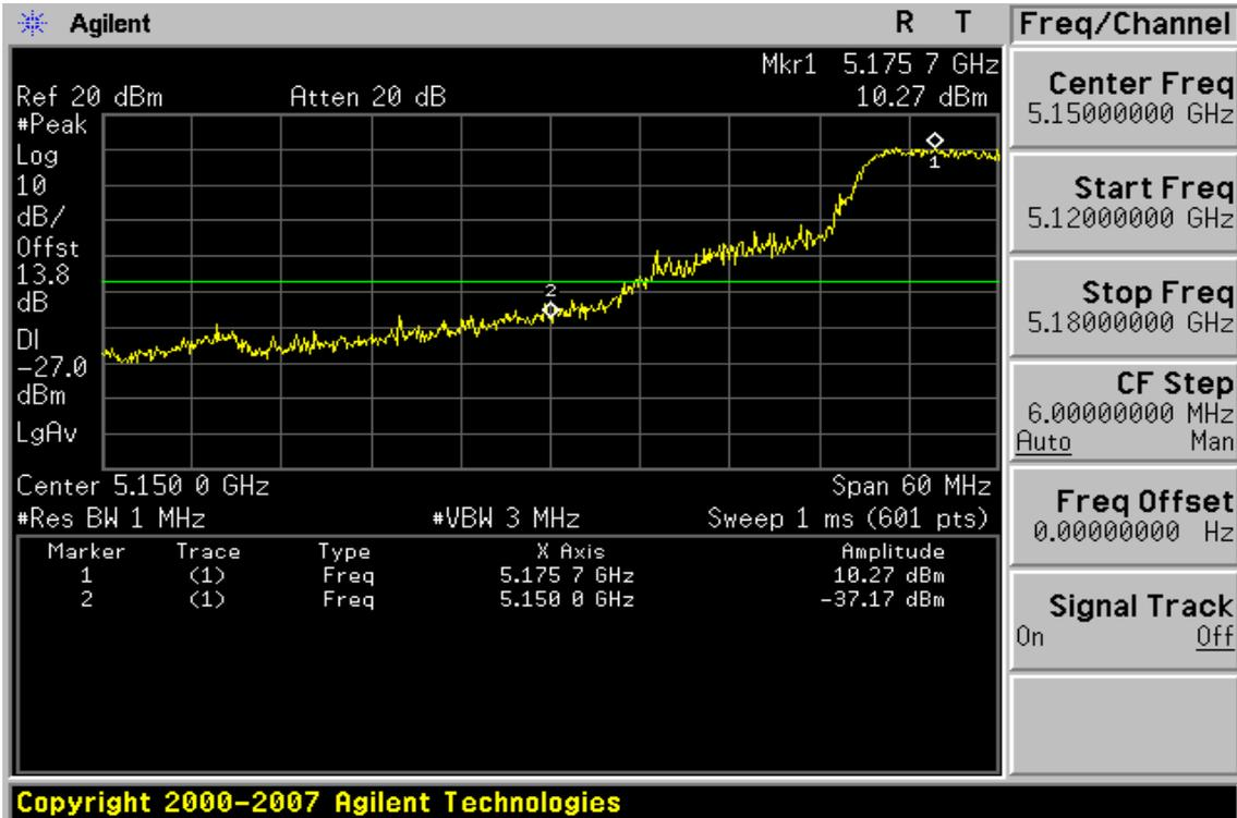
**Band Edges Test Data CH 5350**
