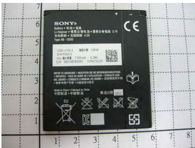
Fig.20 Back view of battery (Model No.: BA900, Supplier: SONY, Type No.: AB-0500)
