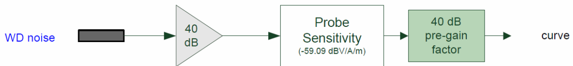
Figure 6-2 Audio Band Magnetic Curve Measurement Block Diagram
