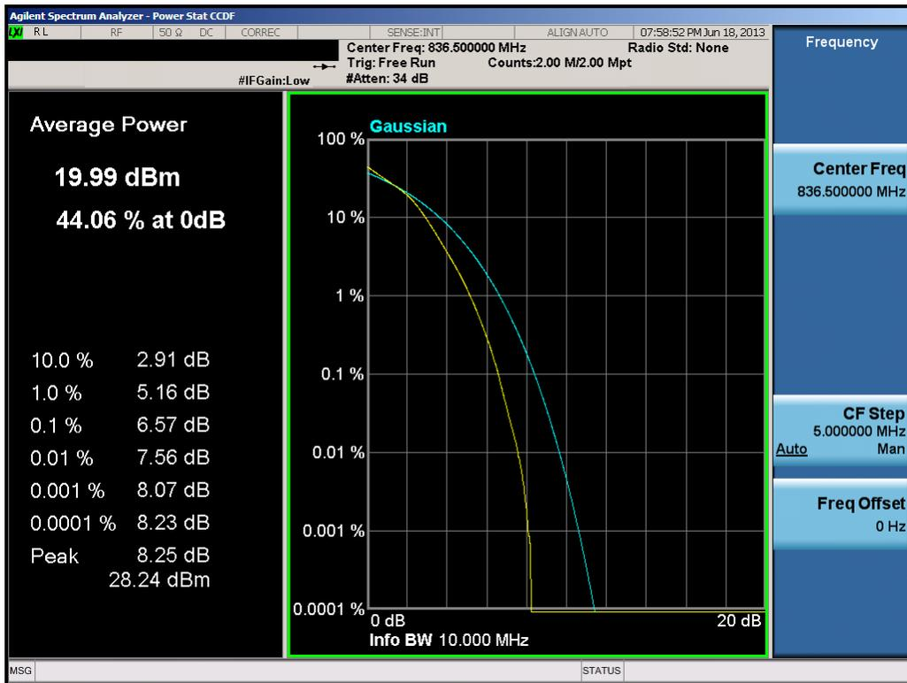
**Plot 7-38. PAR Plot (10.0MHz 16-QAM – RB Size 50)**
