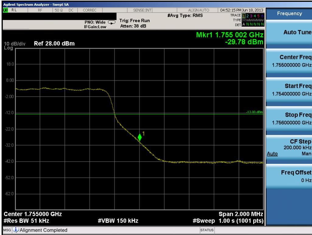
Plot 8-27. Upper Band Edge Plot (5.0MHz QPSK – RB Size 25)
