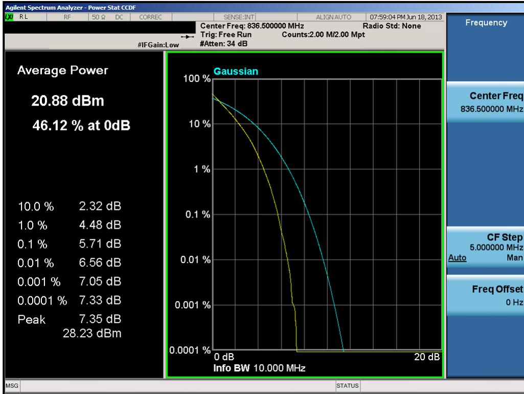
**Plot 7-37. PAR Plot (10.0MHz QPSK – RB Size 50)**
