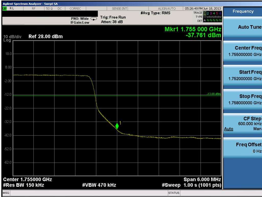
Plot 8-43. Upper Band Edge Plot (15.0MHz QPSK – RB Size 75)
