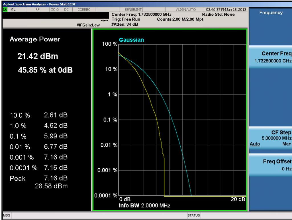
Plot 8-7. PAR Plot (1.4MHz QPSK – RB Size 6)
