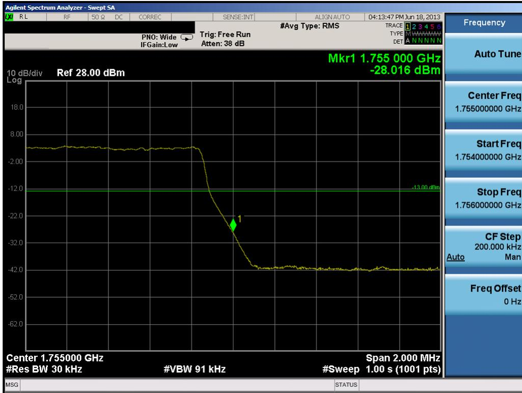
Plot 8-13. Upper Band Edge Plot (3.0MHz QPSK – RB Size 15)
