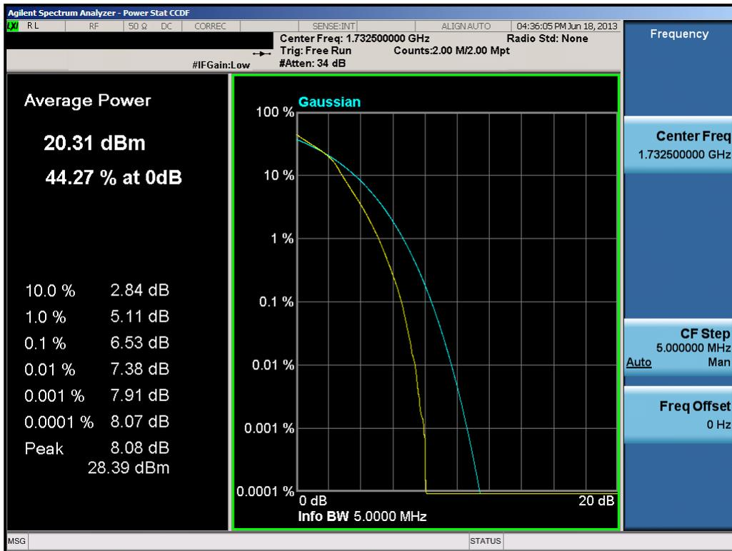
Plot 8-30. PAR Plot (5.0MHz 16-QAM – RB Size 25)
