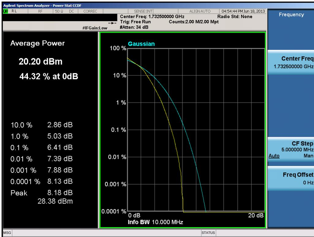
**Plot 8-38. PAR Plot (10.0MHz 16-QAM – RB Size 50)**
