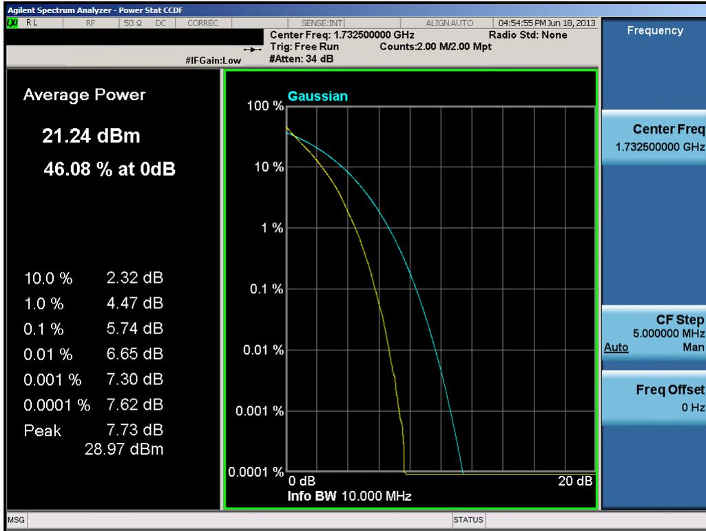
**Plot 8-37. PAR Plot (10.0MHz QPSK – RB Size 50)**
