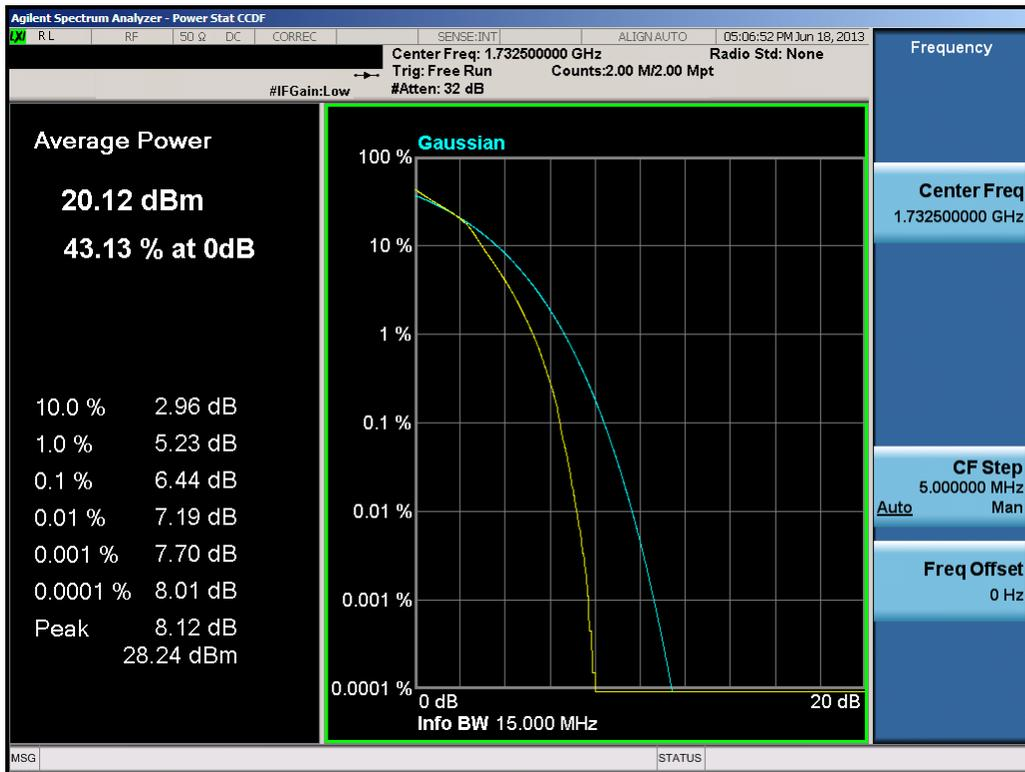
**Plot 8-46. PAR Plot (15.0MHz 16-QAM – RB Size 75)**
