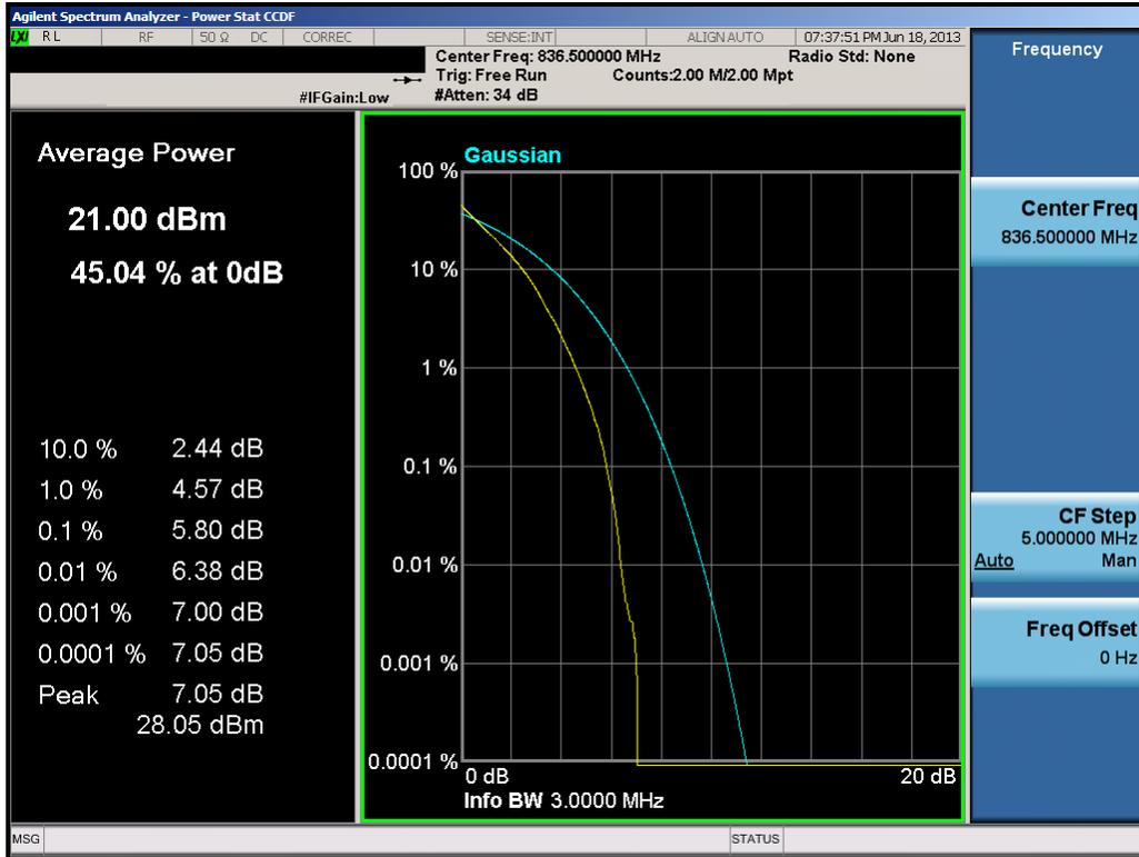
Plot 7-15. PAR Plot (3.0MHz QPSK – RB Size 15)
