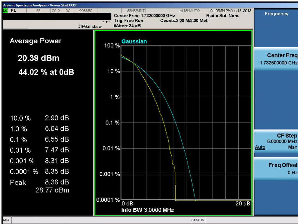
**Plot 8-16. PAR Plot (3.0MHz 16-QAM – RB Size 15)**
