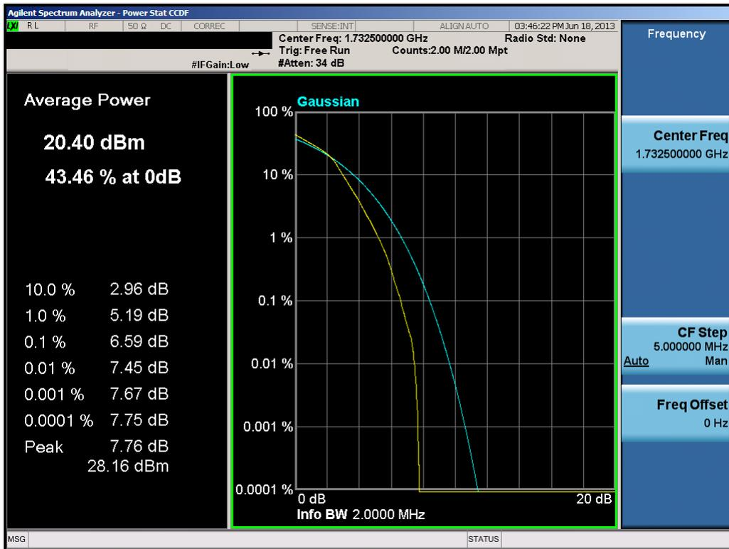
Plot 8-8. PAR Plot (1.4MHz 16-QAM – RB Size 6)
