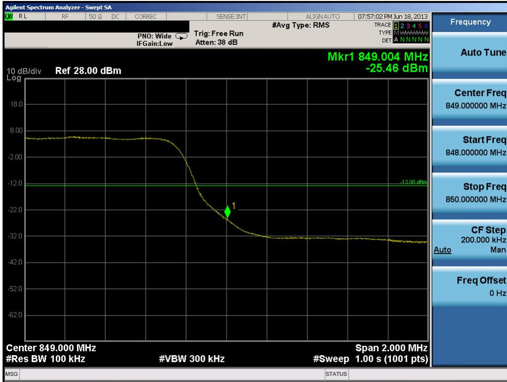
Plot 7-27. Upper Band Edge Plot (5.0MHz QPSK – RB Size 25)
