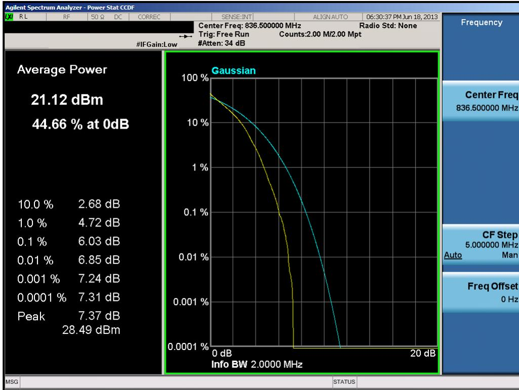
Plot 7-7. PAR Plot (1.4MHz QPSK – RB Size 6)
