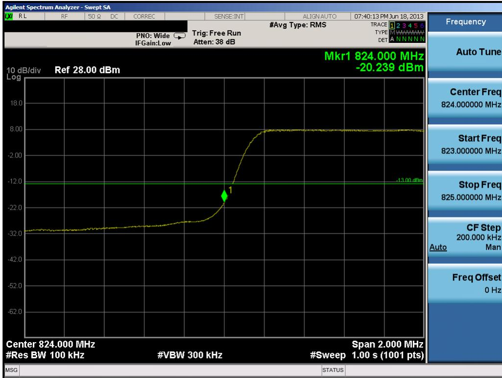
Plot 7-9. Lower Band Edge Plot (3.0MHz QPSK – RB Size 15)
