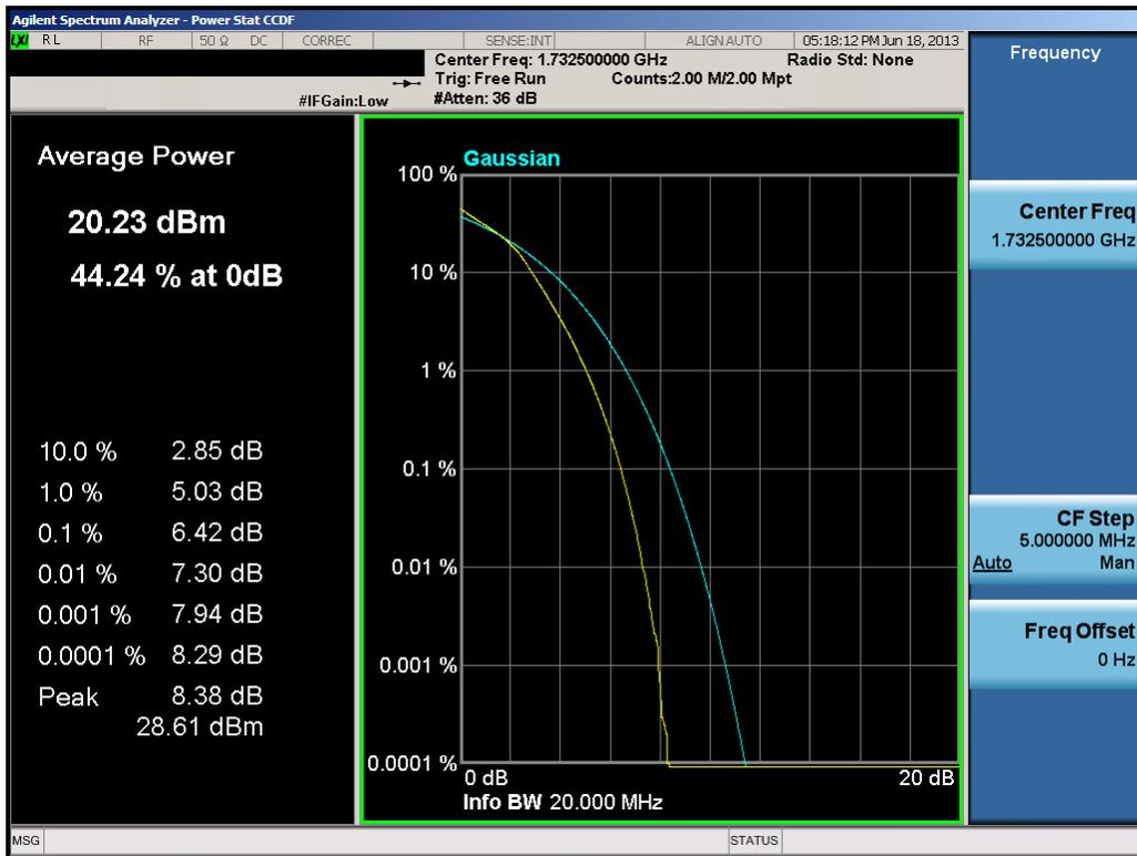
**Plot 8-54. PAR Plot (20.0MHz 16-QAM – RB Size 100)**
