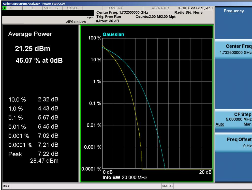
**Plot 8-53. PAR Plot (20.0MHz QPSK – RB Size 100)**
