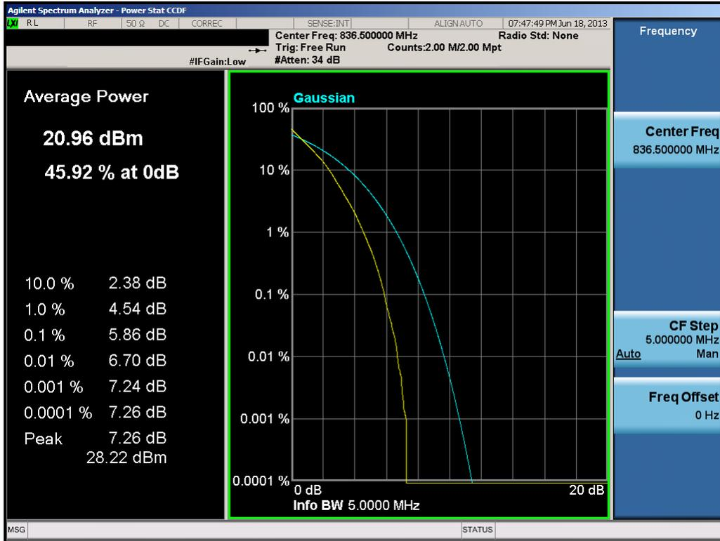
**Plot 7-29. PAR Plot (5.0MHz QPSK – RB Size 25)**
