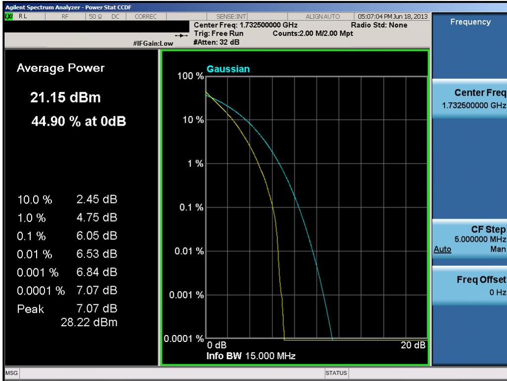
**Plot 8-45. PAR Plot (15.0MHz QPSK – RB Size 75)**
