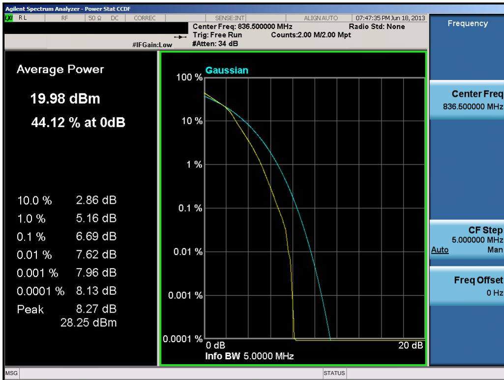
**Plot 7-30. PAR Plot (5.0MHz 16-QAM – RB Size 25)**
