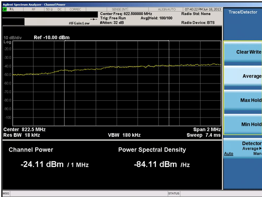
Plot 7-10. Lower Extended Band Edge Plot (3.0MHz QPSK – RB Size 15)
