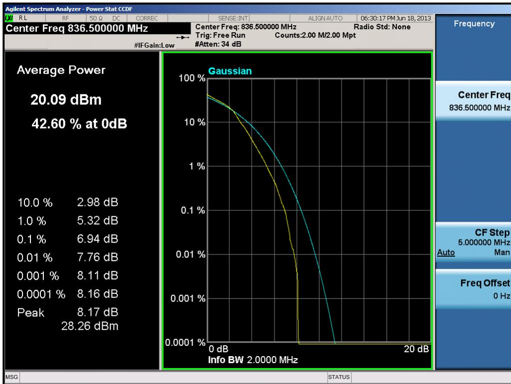
Plot 7-8. PAR Plot (1.4MHz 16-QAM – RB Size 6)
