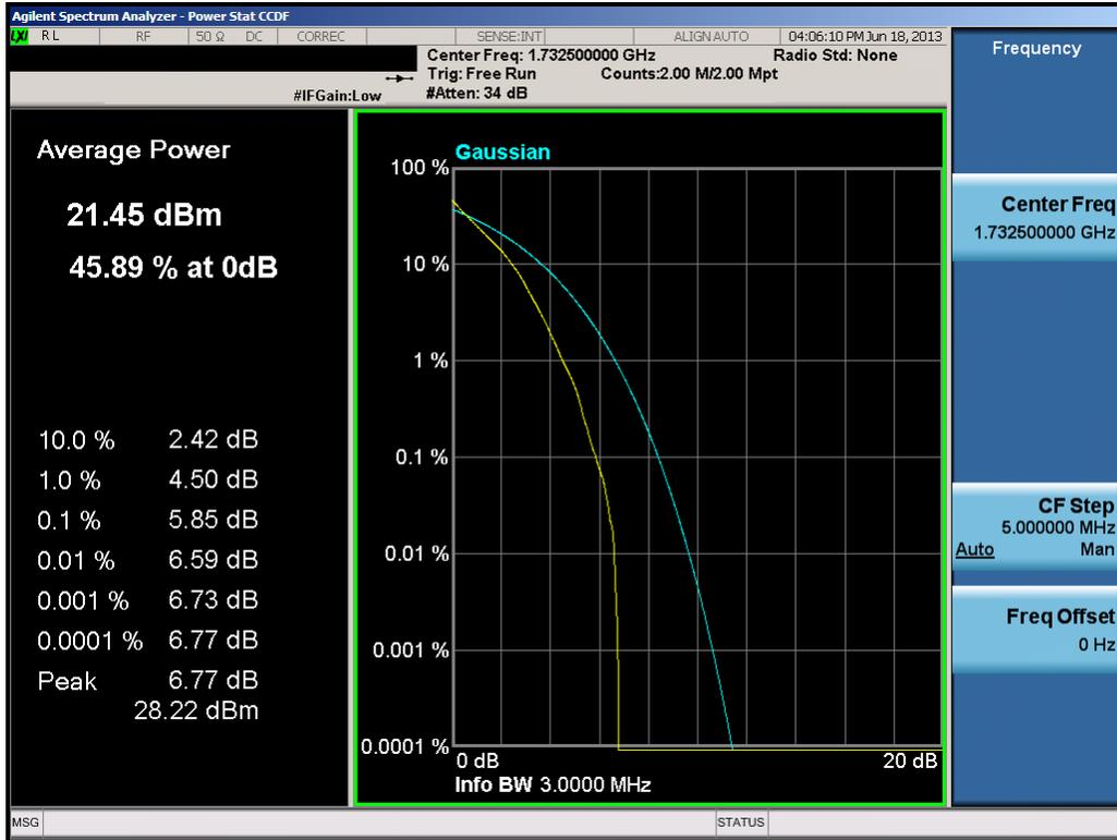
**Plot 8-15. PAR Plot (3.0MHz QPSK – RB Size 15)**
