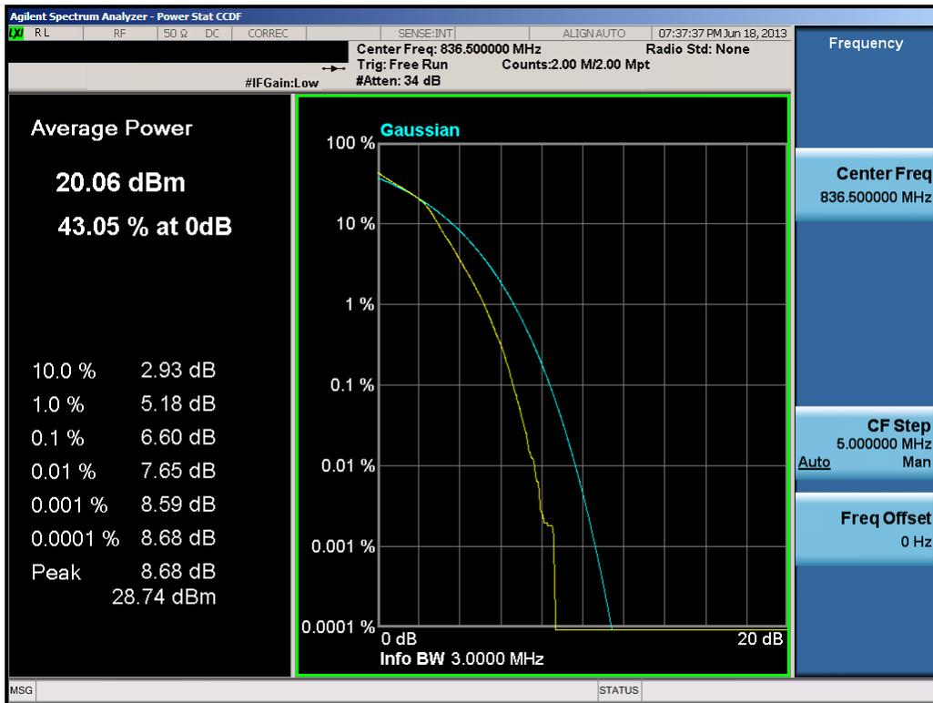
Plot 7-16. PAR Plot (3.0MHz 16-QAM – RB Size 15)
