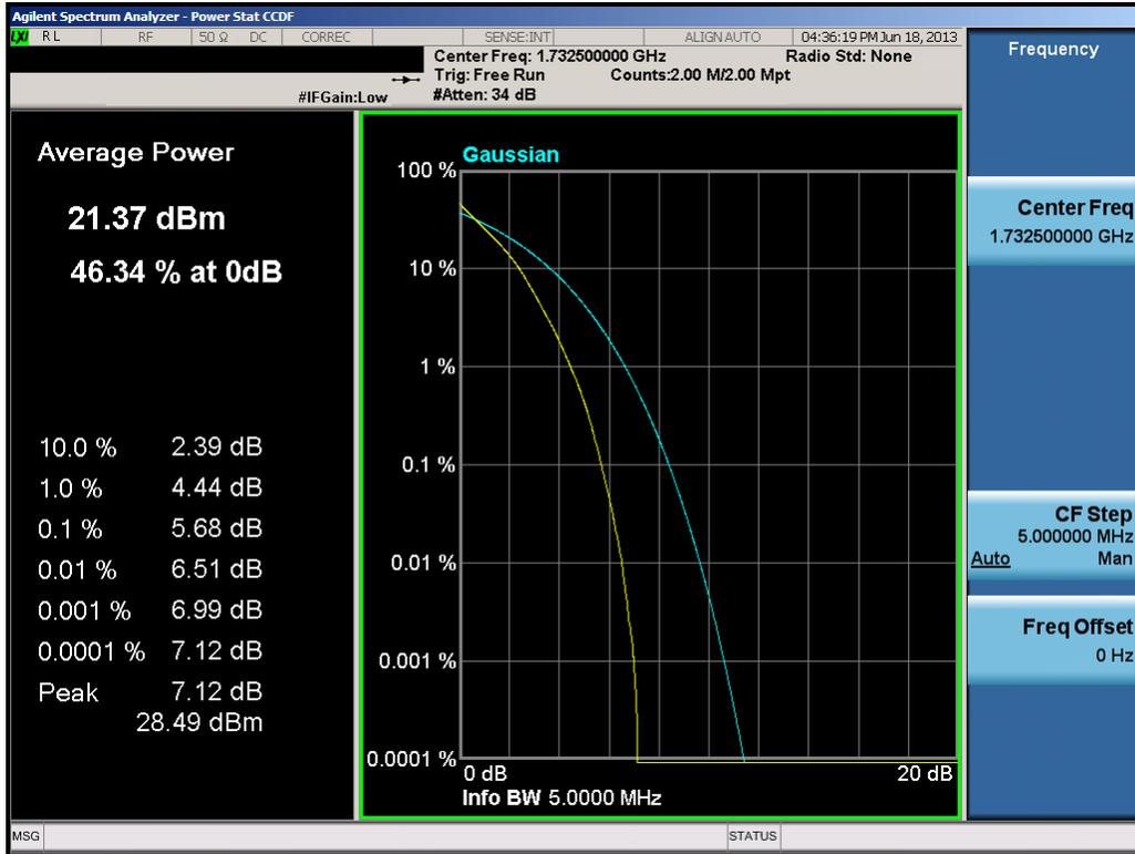
Plot 8-29. PAR Plot (5.0MHz QPSK – RB Size 25)
