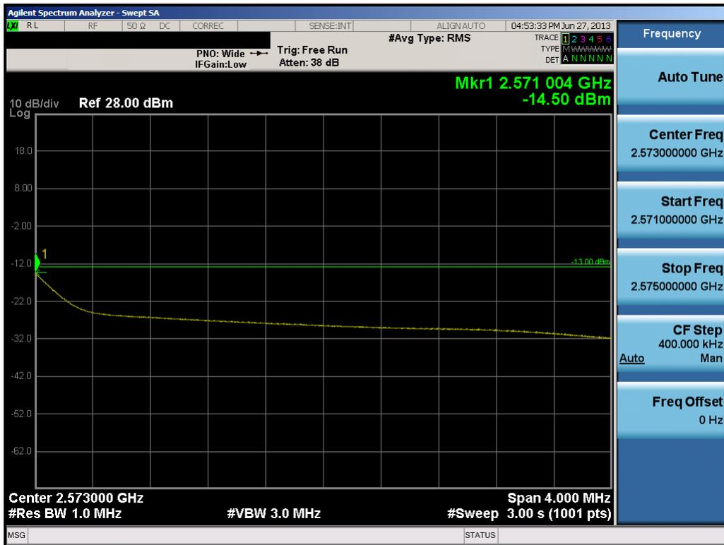
Plot 10-10. Upper Extended Band Edge Plot (5.0MHz QPSK – RB Size 25)
