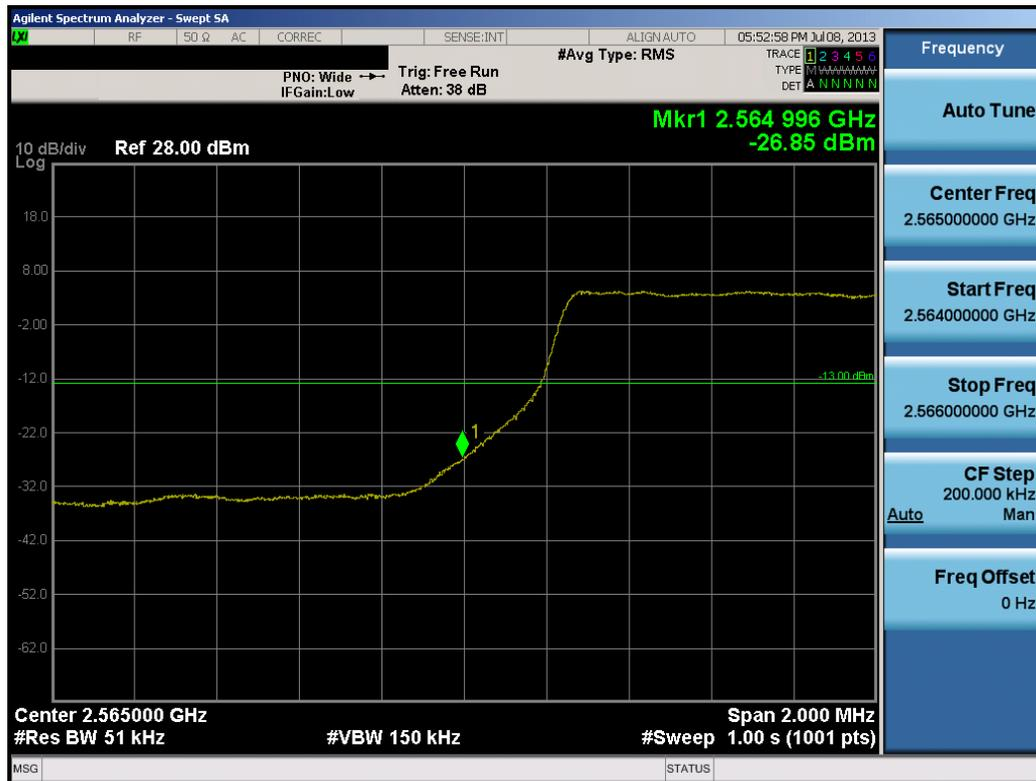
Plot 10-8. High Channel Lower Channel Edge Plot (5.0MHz QPSK – RB Size 25)
