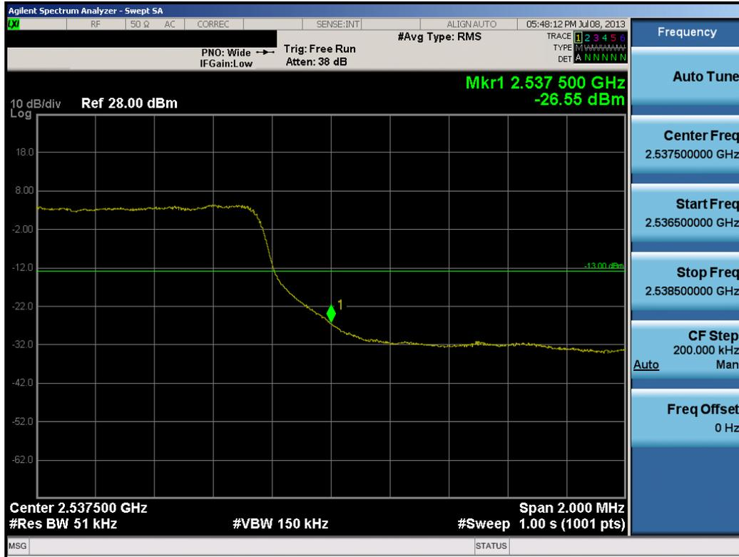
Plot 10-7. Mid Channel Upper Channel Edge Plot (5.0MHz QPSK – RB Size 25)
