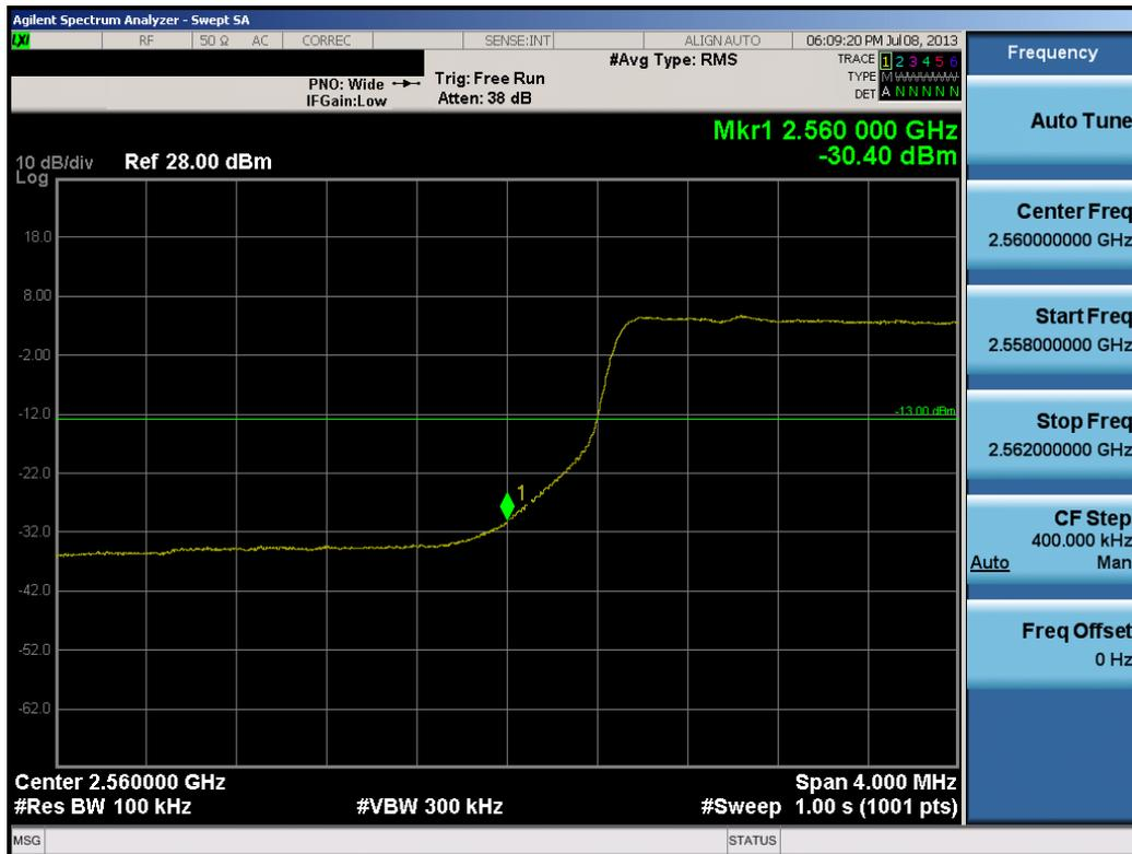
Plot 10-26. Low Channel Lower Channel Edge Plot (10.0MHz QPSK – RB Size 50)
