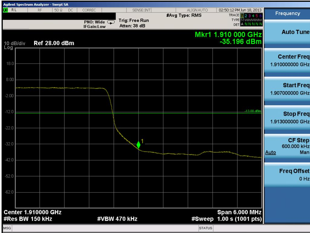
Plot 9-43. Upper Band Edge Plot (15.0MHz QPSK – RB Size 75)
