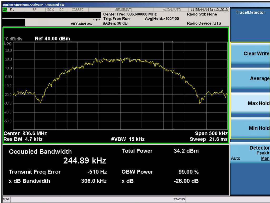
Plot 7-14. Occupied Bandwidth Plot (EDGE850 Mode – Ch. 190)
