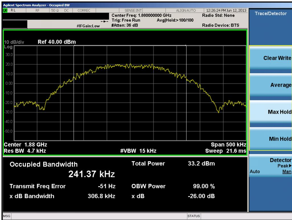
Plot 7-26. Occupied Bandwidth Plot (EDGE1900 Mode – Ch. 661)
