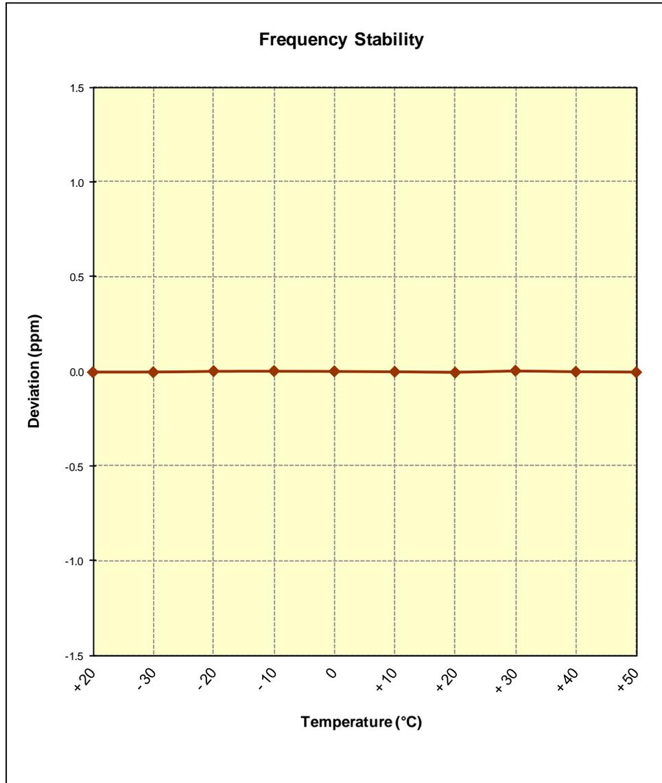
**Figure 6-5. Frequency Stability Graph (PCS WCDMA Mode – Ch. 9400)**
