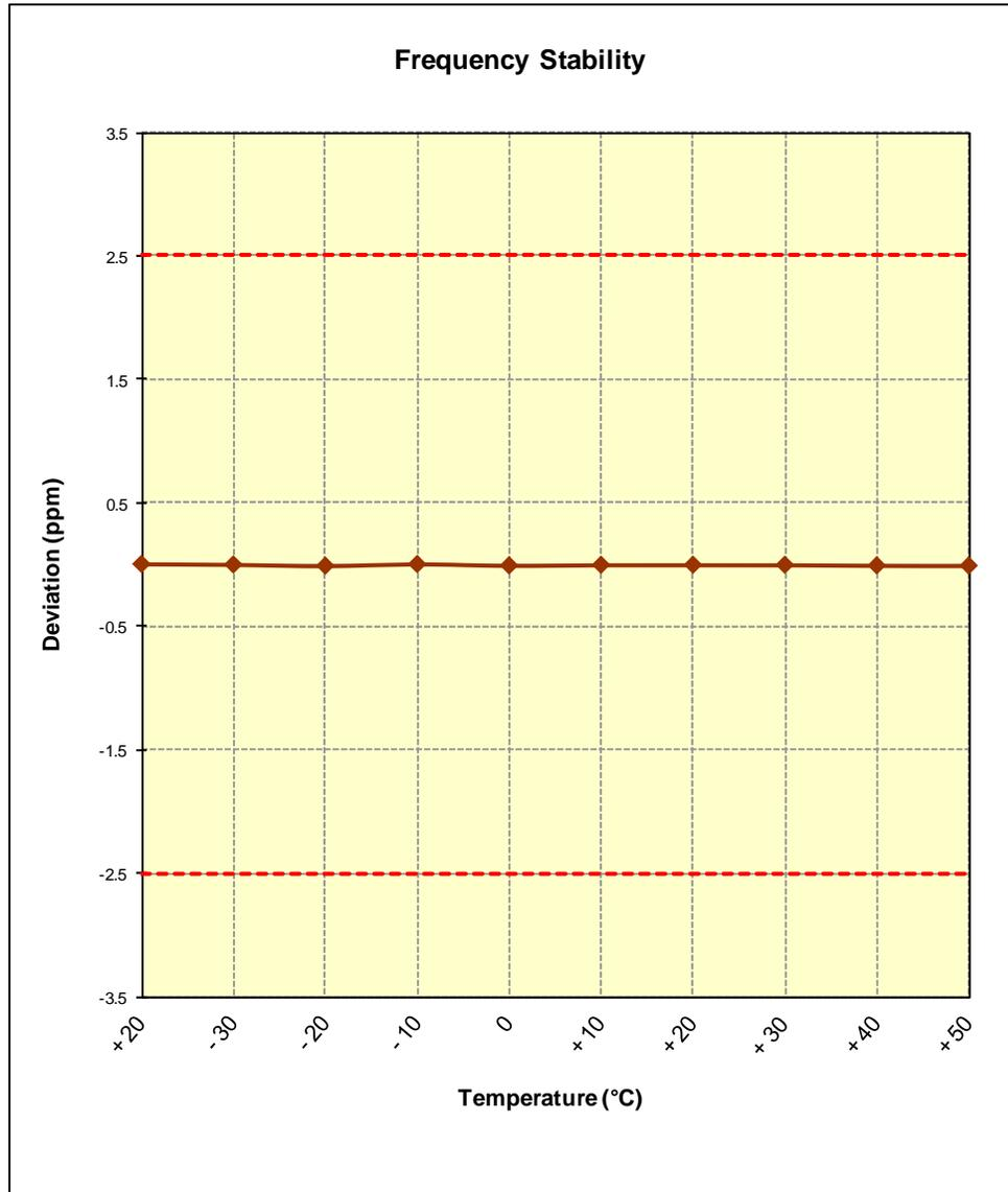
Figure 6-2. Frequency Stability Graph (Cellular WCDMA Mode – Ch. 4183)
