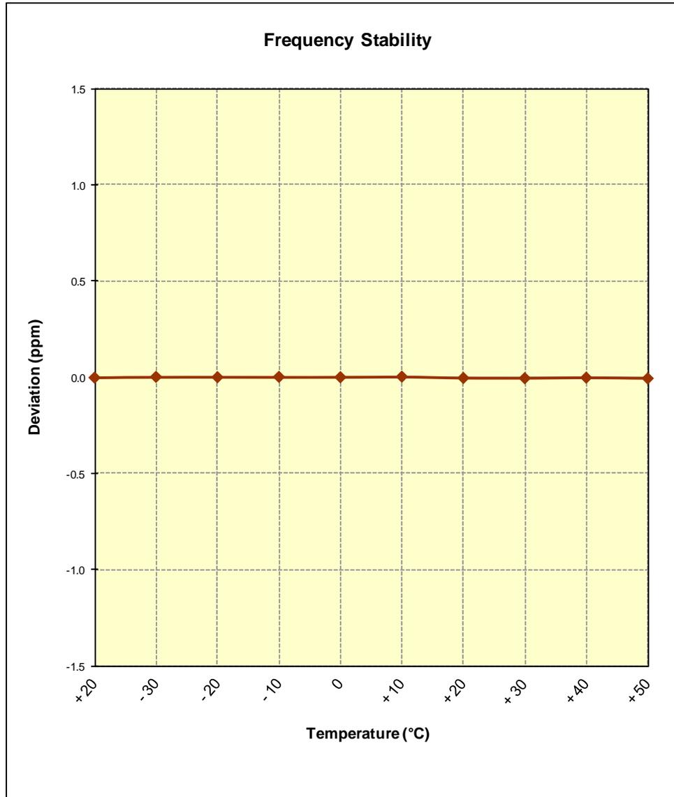
**Figure 6-3. Frequency Stability Graph (AWS WCDMA Mode – Ch. 1413)**
