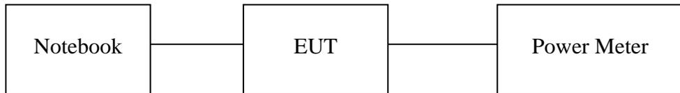
**Fig. 2-2 Configuration of Tested System (Fixed Channel-Radiated)**
