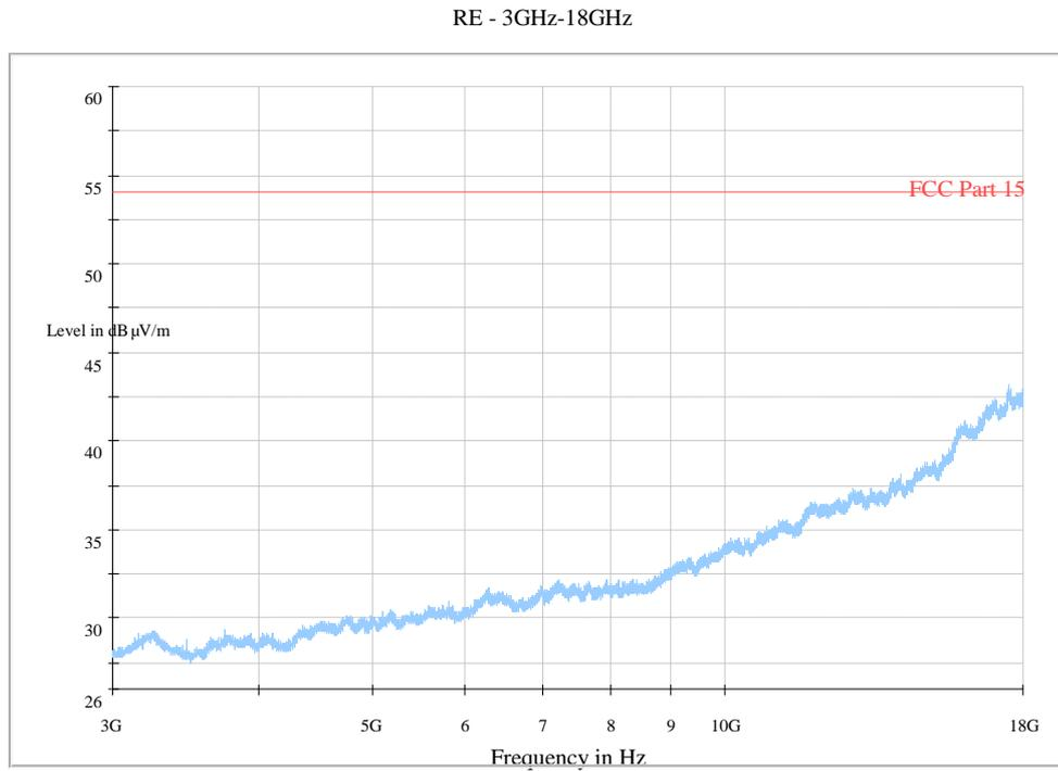
**Fig. 75 Radiated Spurious Emission (802.11n-HT20, Ch11, 3 GHz-18 GHz)**
