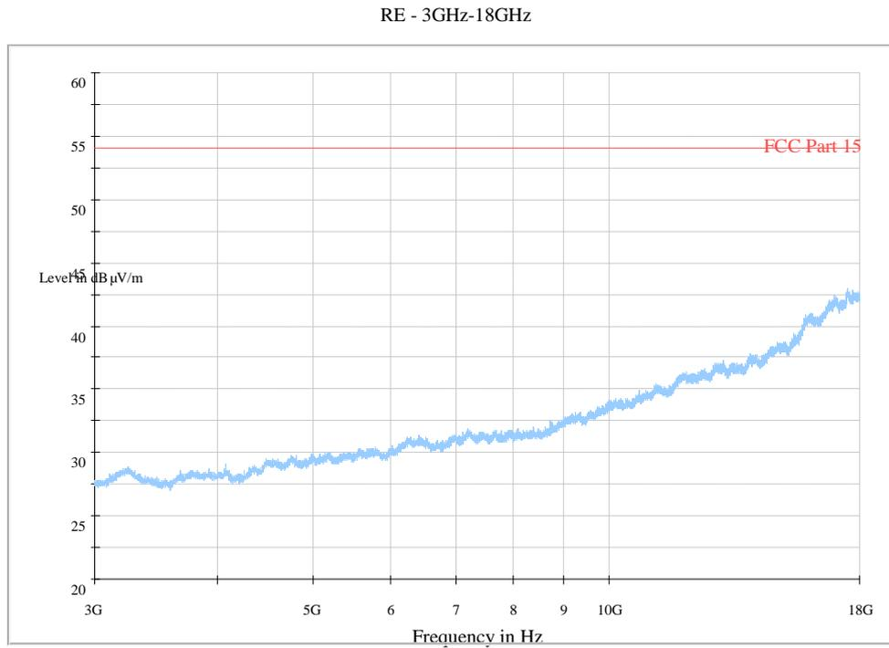
**Fig. 71 Radiated Spurious Emission (802.11n-HT20, Ch6, 3 GHz-18 GHz)**
