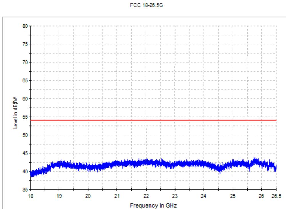
**Fig. 76 Radiated emission: 18 GHz - 26 GHz**
