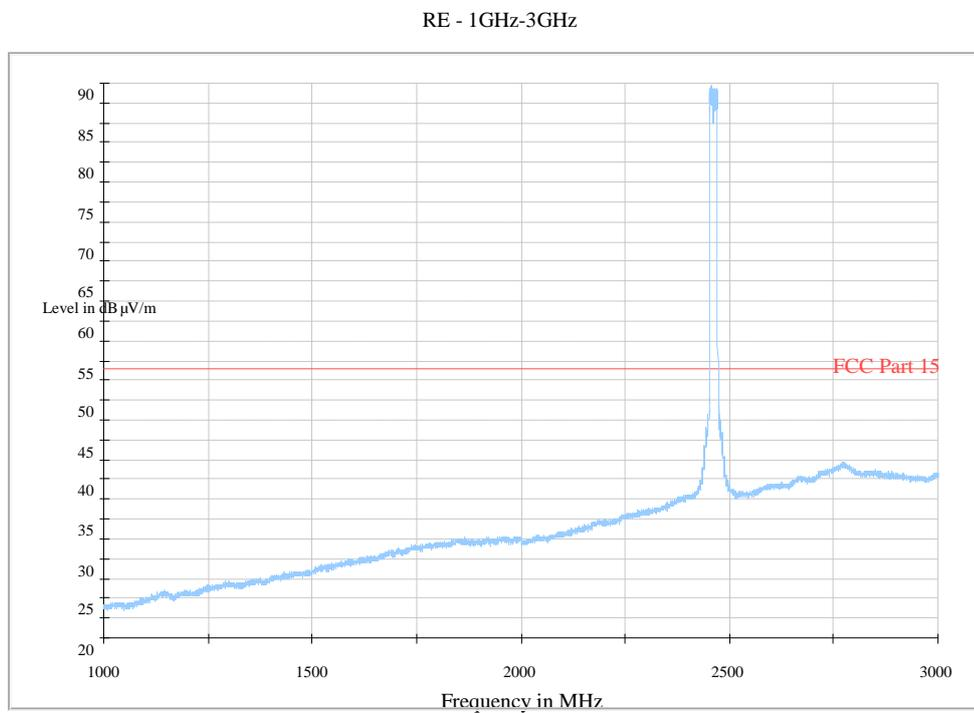
**Fig. 74 Radiated Spurious Emission (802.11n-HT20, Ch11, 1 GHz-3 GHz)**
