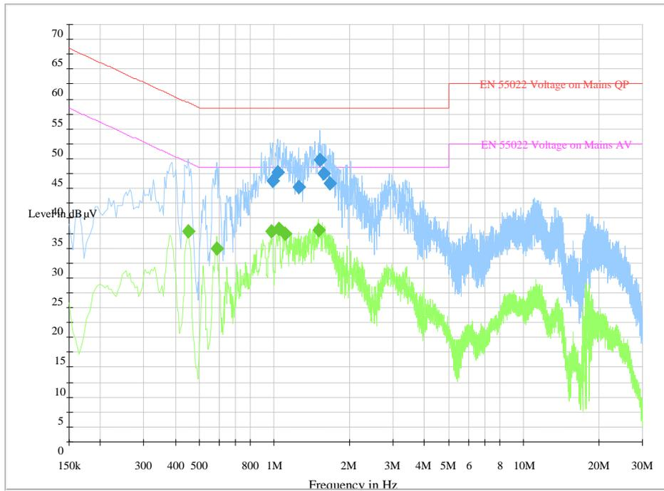
Fig. 77 AC Powerline Conducted Emission
