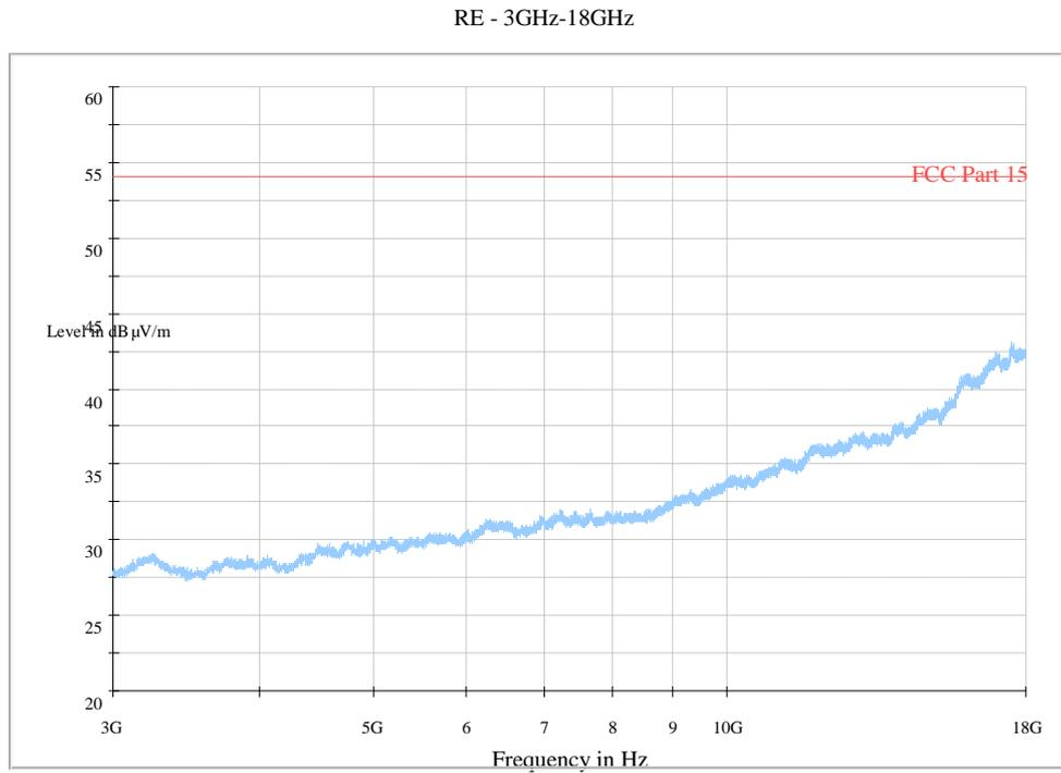
**Fig. 53 Radiated Spurious Emission (802.11b, Ch11, 3 GHz-18 GHz)**
