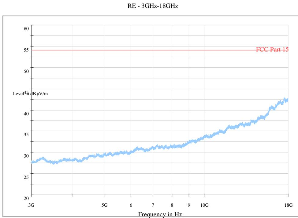
**Fig. 64 Radiated Spurious Emission (802.11g, Ch11, 3 GHz-18 GHz)**
