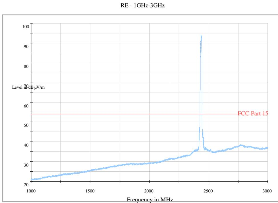
**Fig. 48 Radiated Spurious Emission (802.11b, Ch6, 1 GHz-3 GHz)**
