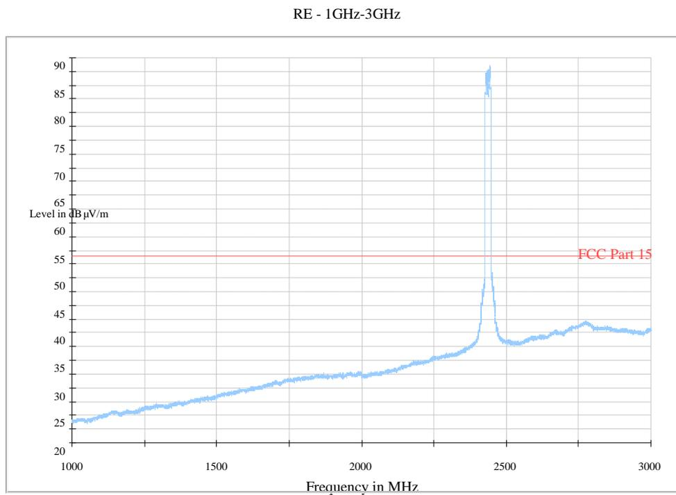
**Fig. 70 Radiated Spurious Emission (802.11n-HT20, Ch6, 1 GHz-3 GHz)**
