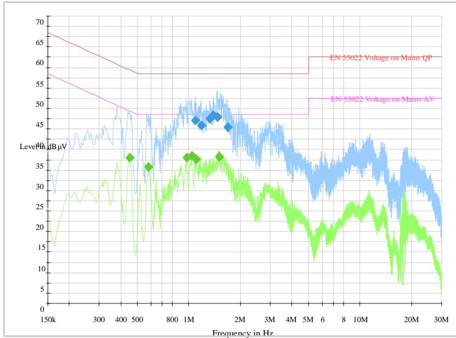
**Fig. 78 AC Powerline Conducted Emission**
