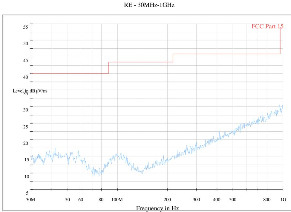
**Fig. 47 Radiated Spurious Emission (802.11b, Ch6, 30 MHz-1 GHz)**
