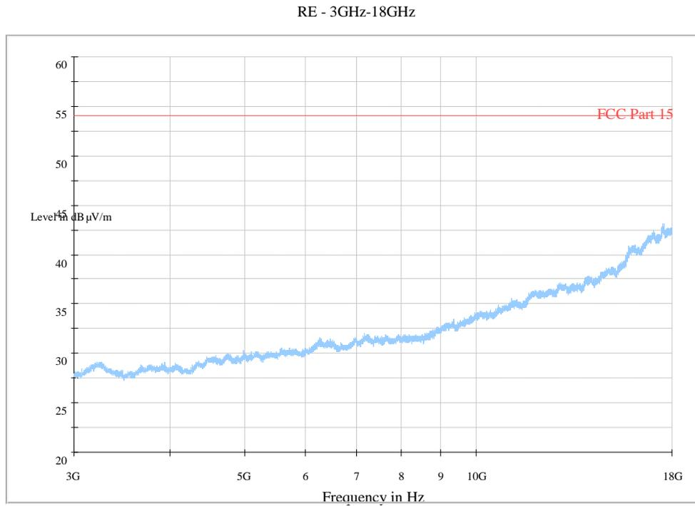
**Fig. 49 Radiated Spurious Emission (802.11b, Ch6, 3 GHz-18 GHz)**
