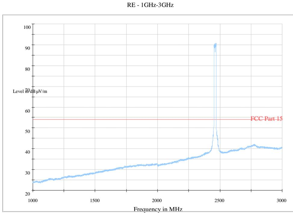
**Fig. 63 Radiated Spurious Emission (802.11g, Ch11, 1 GHz-3 GHz)**
