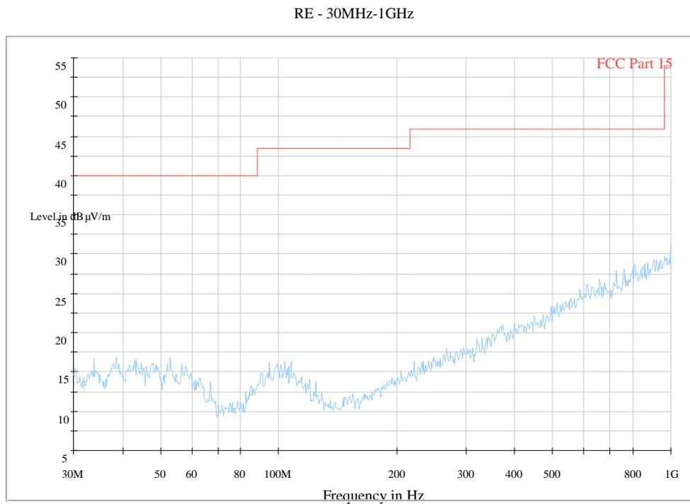
**Fig. 66 Radiated Spurious Emission (802.11n-HT20, Ch1, 30 MHz-1 GHz)**
