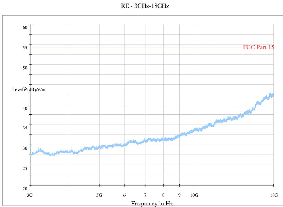
**Fig. 60 Radiated Spurious Emission (802.11g, Ch6, 3 GHz-18 GHz)**
