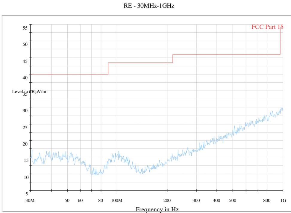
**Fig. 58 Radiated Spurious Emission (802.11g, Ch6, 30 MHz-1 GHz)**
