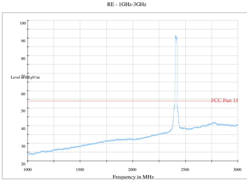
**Fig. 56 Radiated Spurious Emission (802.11g, Ch1, 1 GHz-3 GHz)**
