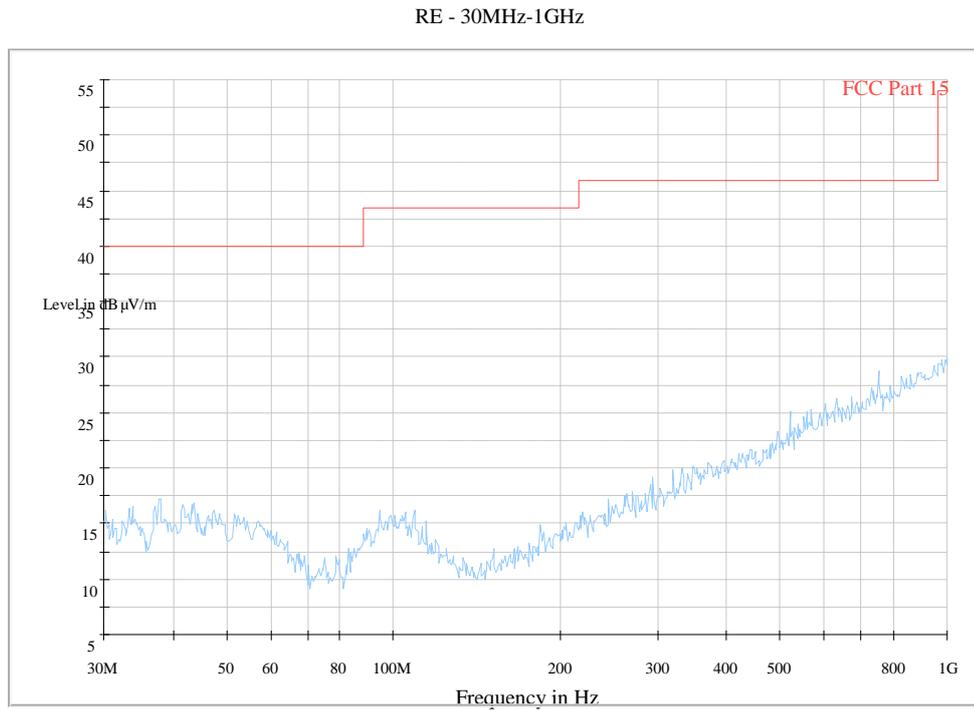
**Fig. 69 Radiated Spurious Emission (802.11n-HT20, Ch6, 30 MHz-1 GHz)**
