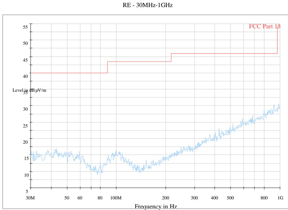
**Fig. 44 Radiated Spurious Emission (802.11b, Ch1, 30 MHz-1 GHz)**
