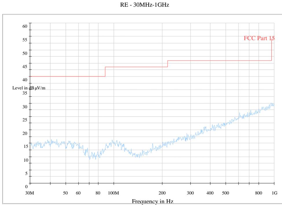
**Fig. 55 Radiated Spurious Emission (802.11g, Ch1, 30 MHz-1 GHz)**
