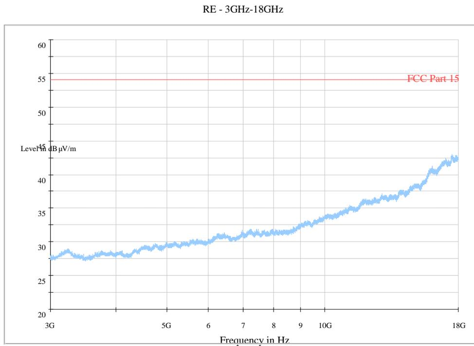
**Fig. 68 Radiated Spurious Emission (802.11n-HT20, Ch1, 3 GHz-18 GHz)**
