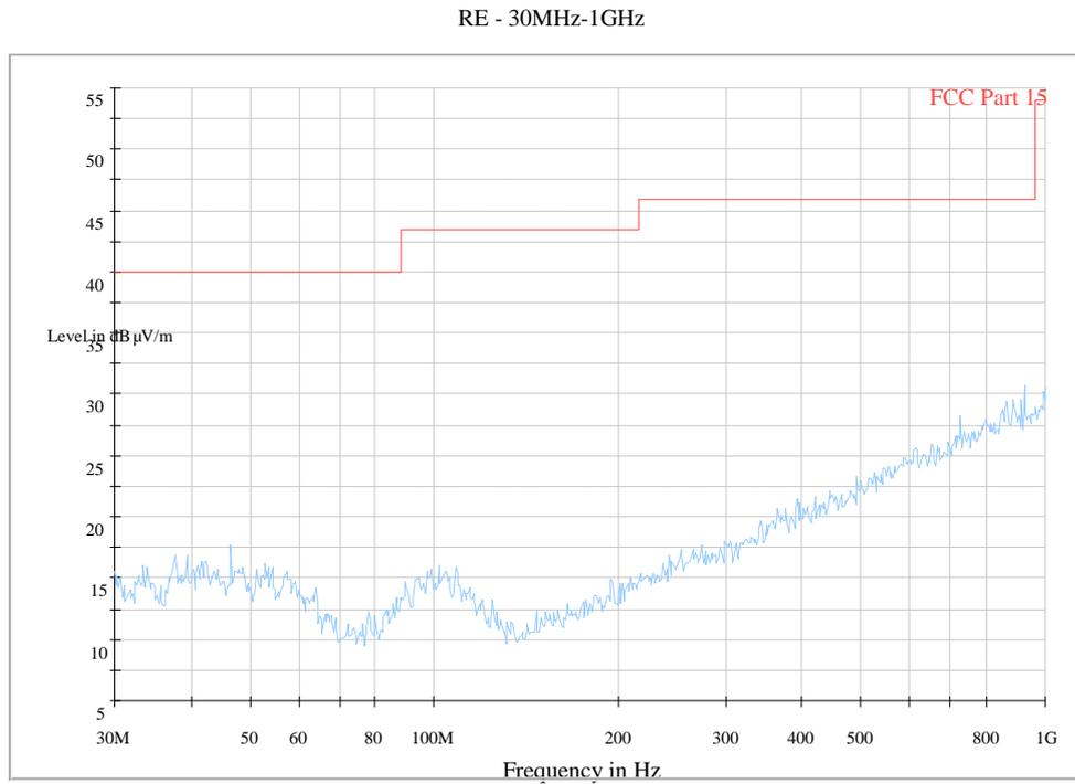
**Fig. 51 Radiated Spurious Emission (802.11b, Ch11, 30 MHz-1 GHz)**
