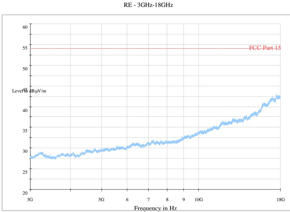
**Fig. 57 Radiated Spurious Emission (802.11g, Ch1, 3 GHz-18 GHz)**
