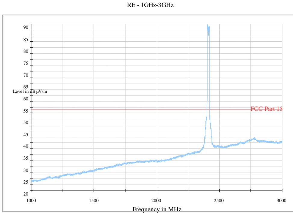
**Fig. 67 Radiated Spurious Emission (802.11n-HT20, Ch1, 1 GHz-3 GHz)**
