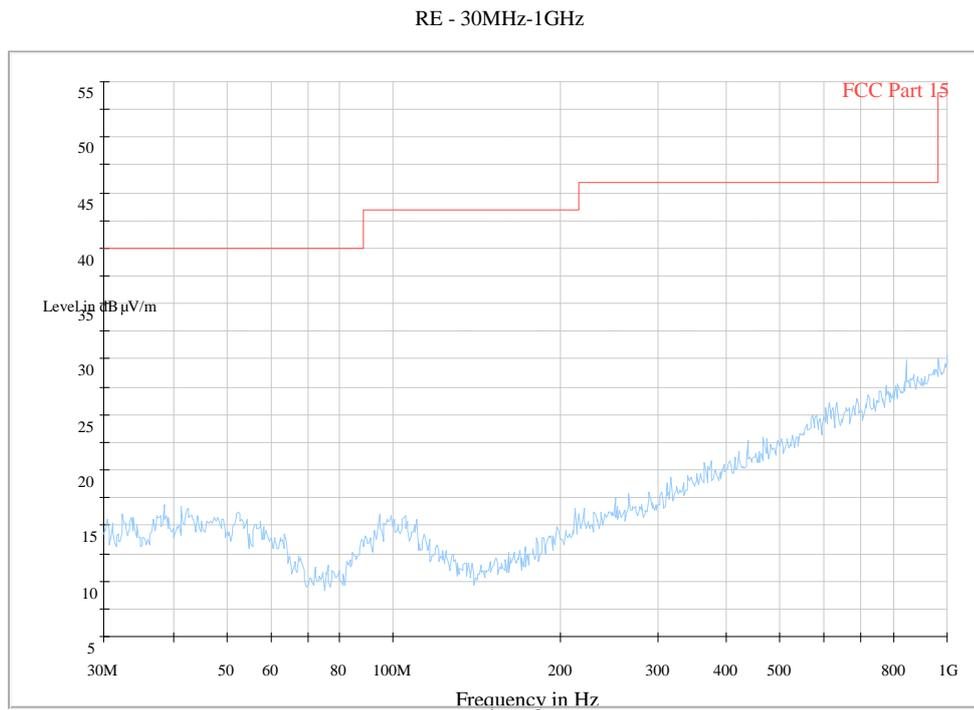
**Fig. 73 Radiated Spurious Emission (802.11n-HT20, Ch11, 30 MHz-1 GHz)**
