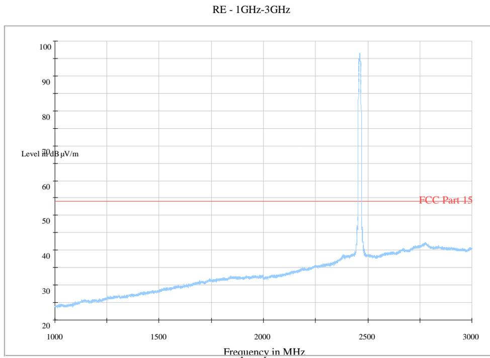
**Fig. 52 Radiated Spurious Emission (802.11b, Ch11, 1 GHz-3 GHz)**
