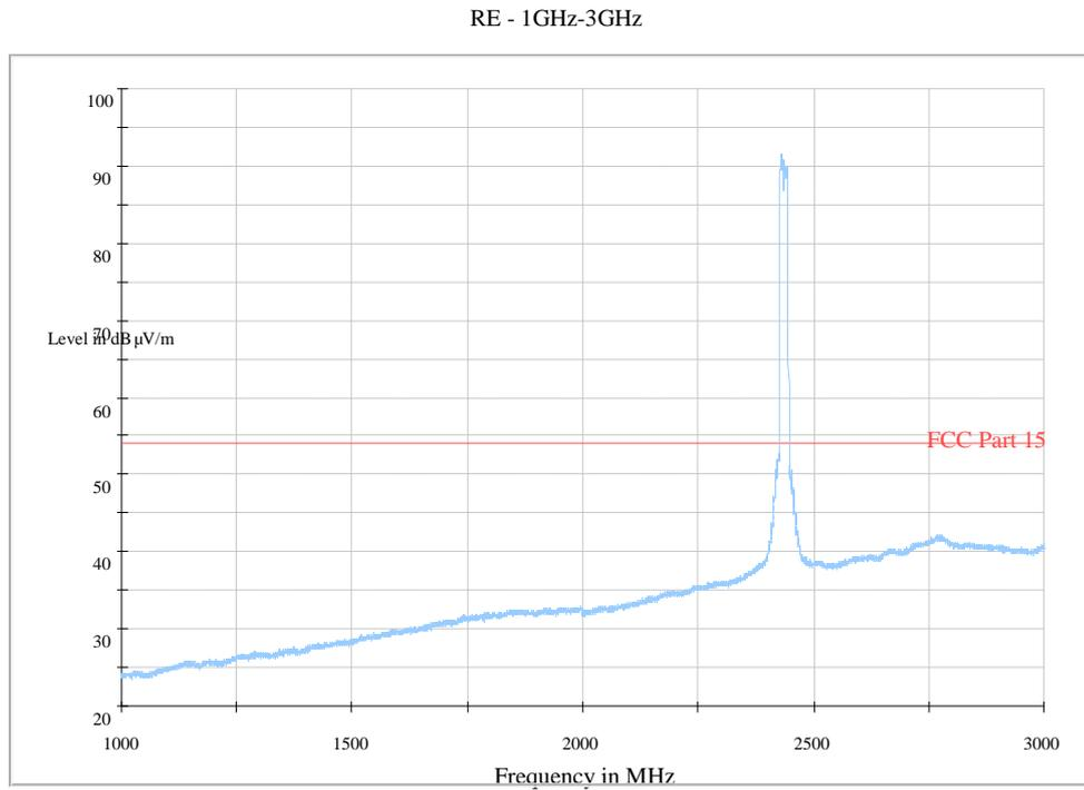
**Fig. 59 Radiated Spurious Emission (802.11g, Ch6, 1 GHz-3 GHz)**
