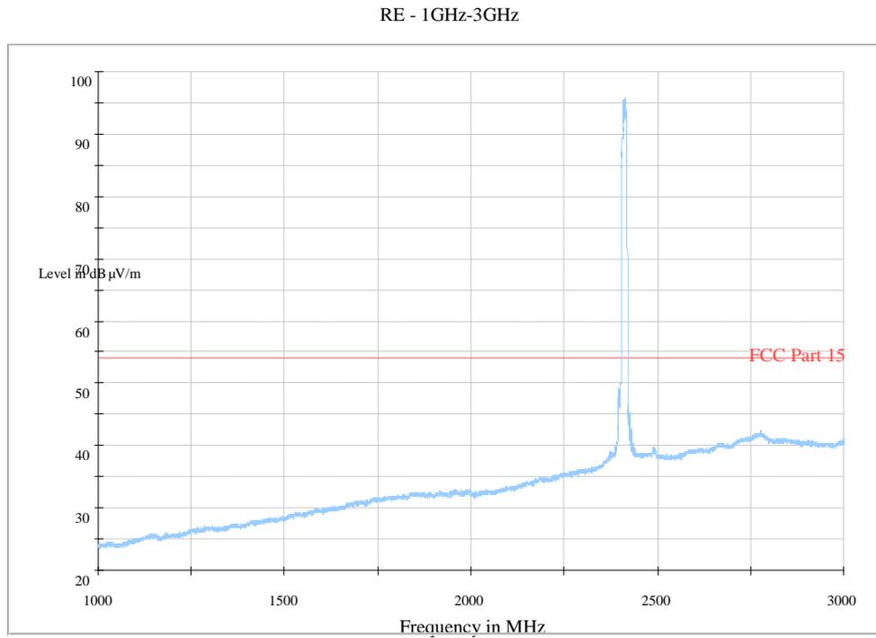
**Fig. 45 Radiated Spurious Emission (802.11b, Ch1, 1 GHz-3 GHz)**
