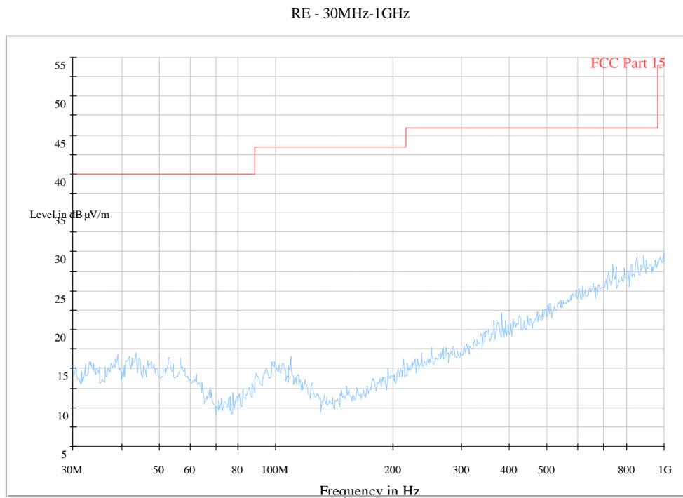
**Fig. 62 Radiated Spurious Emission (802.11g, Ch11, 30 MHz-1 GHz)**
