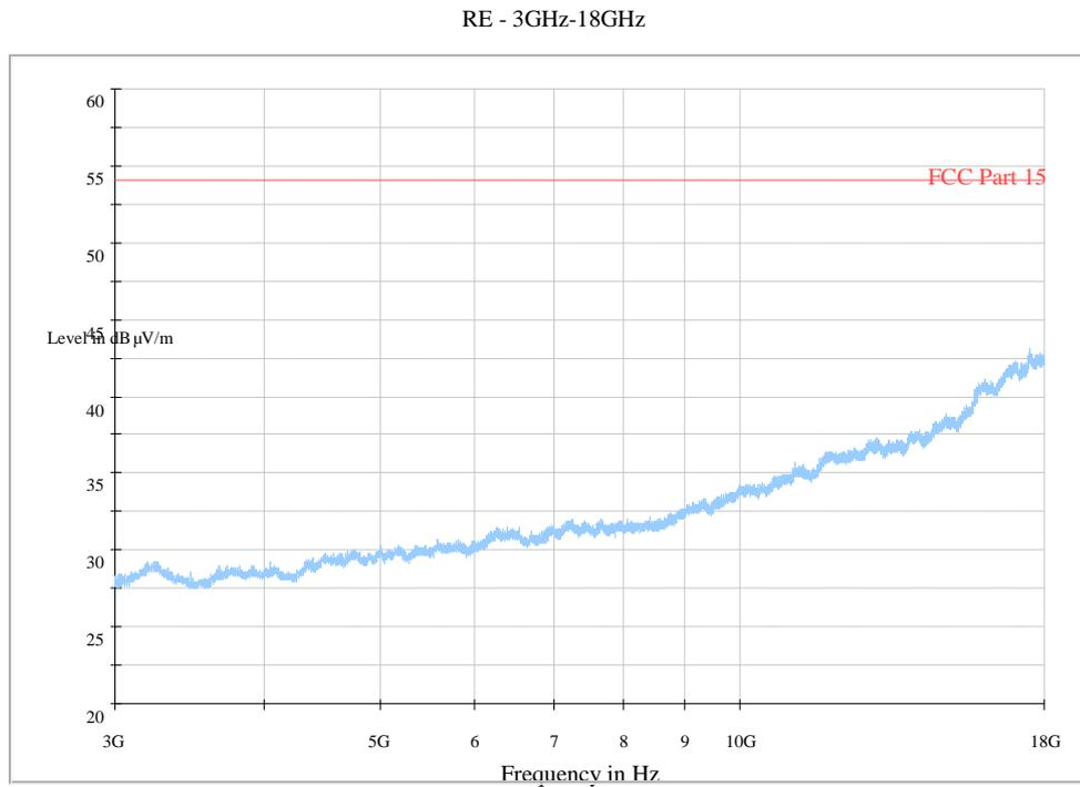
**Fig. 46 Radiated Spurious Emission (802.11b, Ch1, 3 GHz-18 GHz)**
