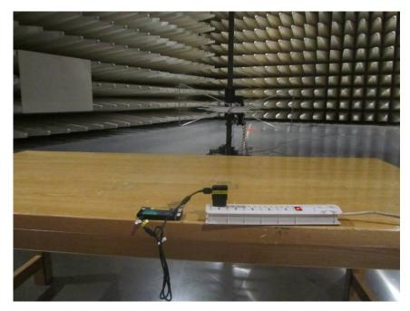
**Layout of AC Powerline Conducted Emission**
