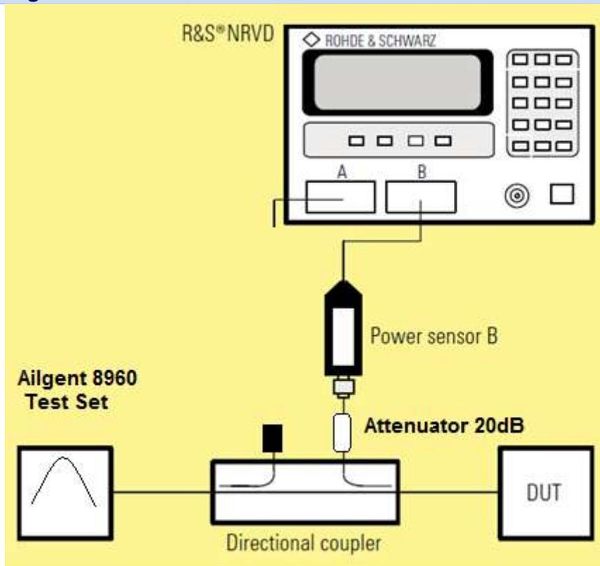
**A.8.1. Establish a DC-HSDPA RB Test Mode Connection with DL 42Mbps**
