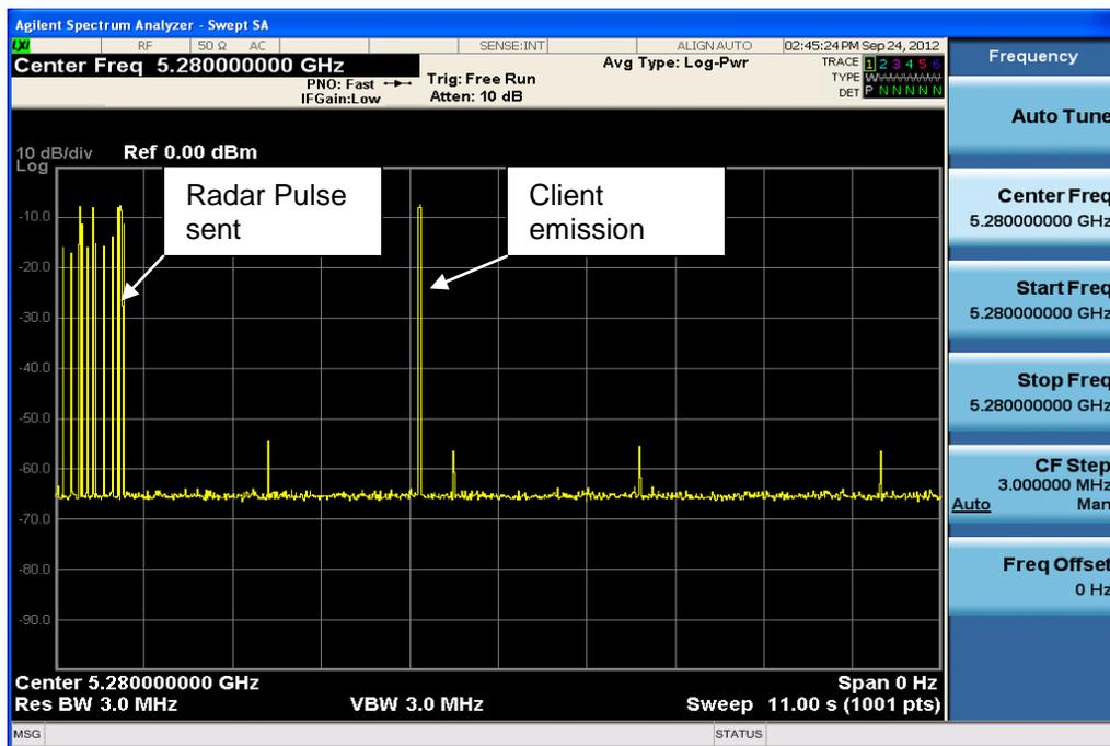
The arrow shows the time of the radar pulse. On the plot you can see that no transmissions occur from the AP after sending the radar burst. The time difference between the recognition of the radar burst by the AP and its last transmission is called as Channel Move Time (Limit: 10 s). The accumulated transmission time of the AP and for the slave device after detection of a radar signal is called channel closing transmission time (Limit: in total 200 ms + 60 ms).
