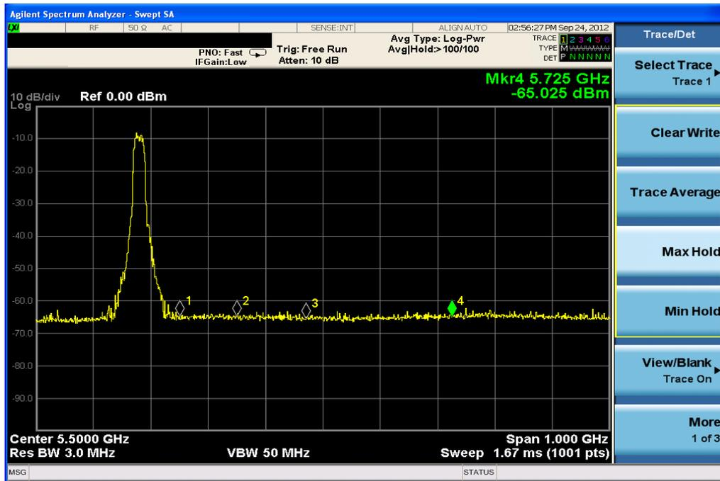
The plot shows that no transmissions over a 30 minutes period occur within the DFS-Bands (between marker 1 and 2 and between Marker 3 and 4). The emissions above are not within the DFS-bands.
