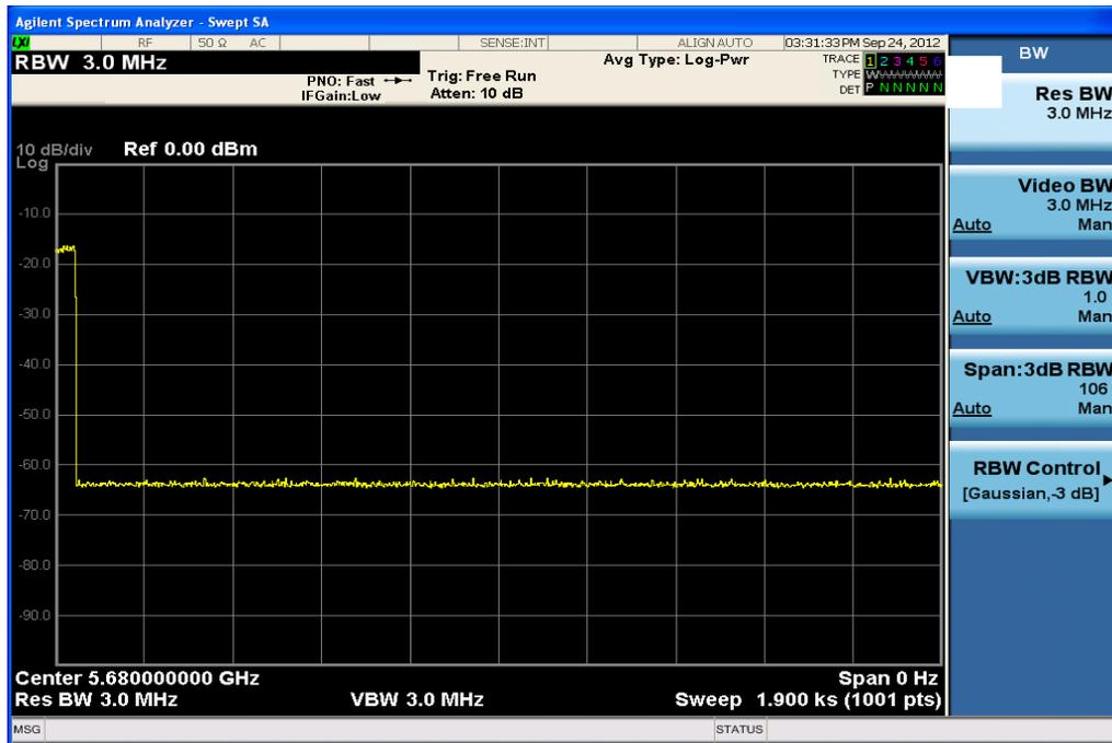
In the plot above you can see, that the client does not transmit any emission within 30 minutes after having received the "stop transmit" order from the Access Point (DFS-Master).
