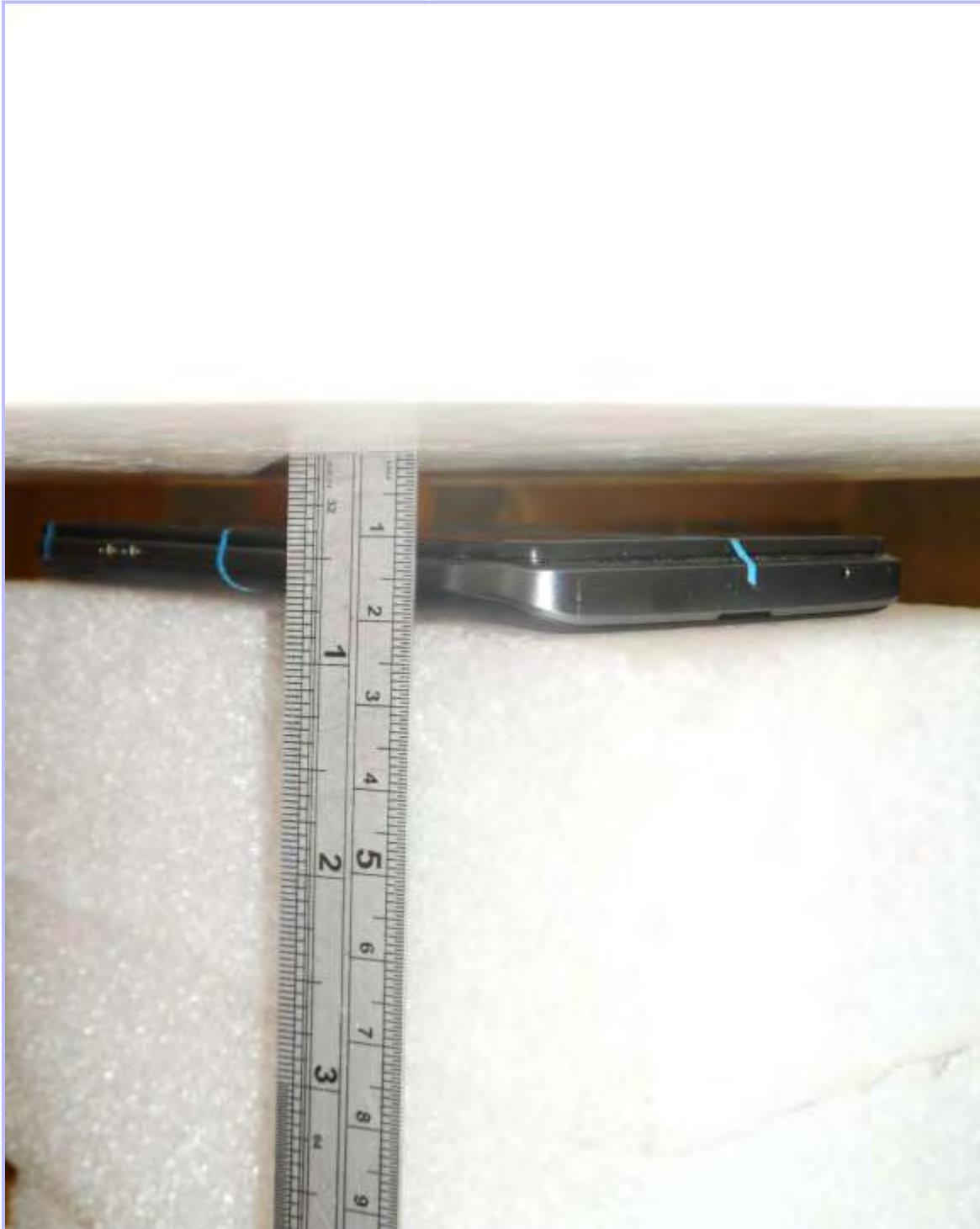
PHT/89439JD001/008: Back of EUT facing Phantom at 10mm
