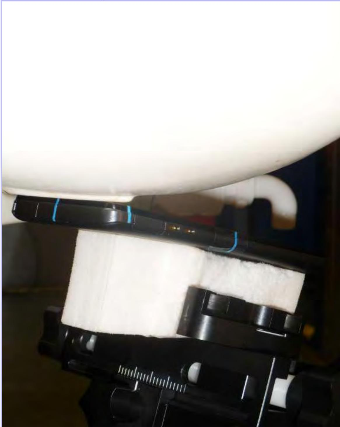
PHT/89439JD02/006: Front of EUT facing Phantom at 10mm
