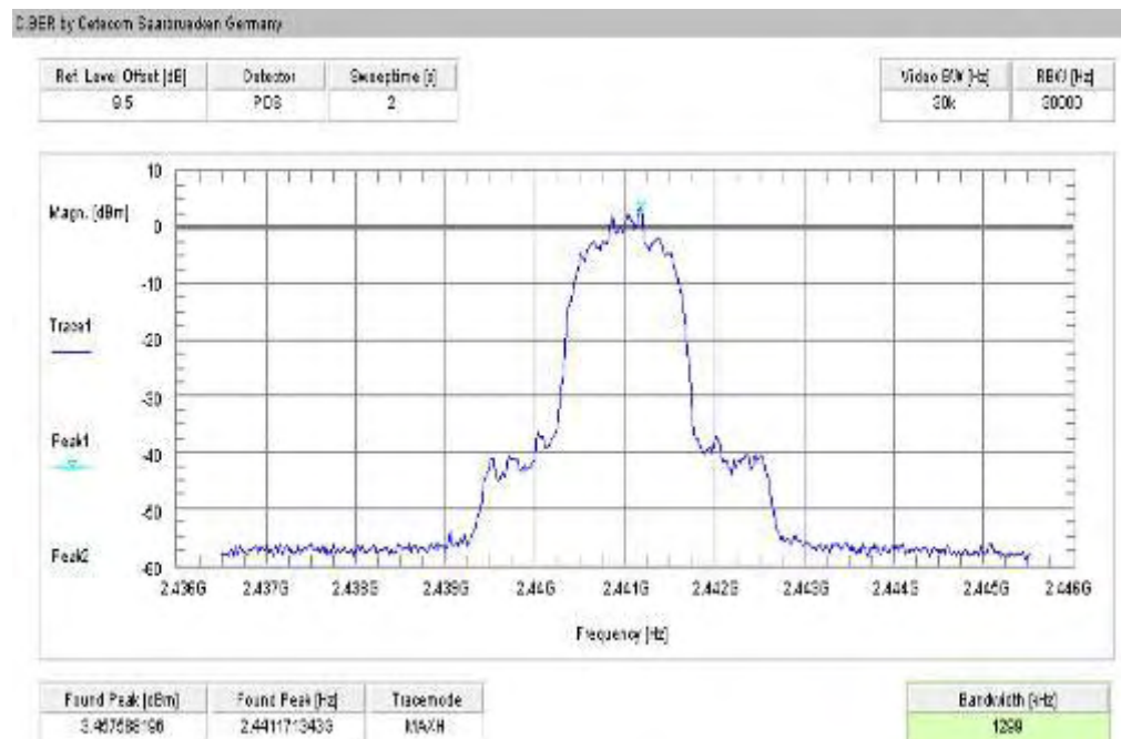
Plot 8: middle channel – 2441 MHz, 8 DPSK modulation
