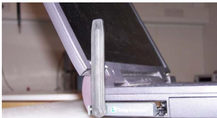
**GC89 with extended antenna connected in DELL Laptop**
