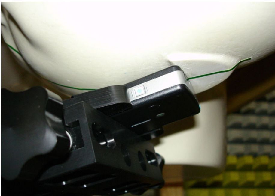
(b) Device on head phantom in the tilt position.
