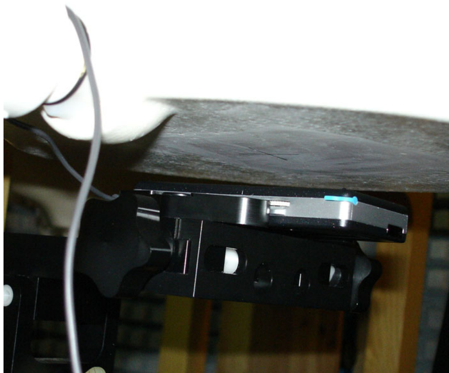
(c) Device on flat section of the phantom. The separation was 15 mm between the device and the flat phantom.
