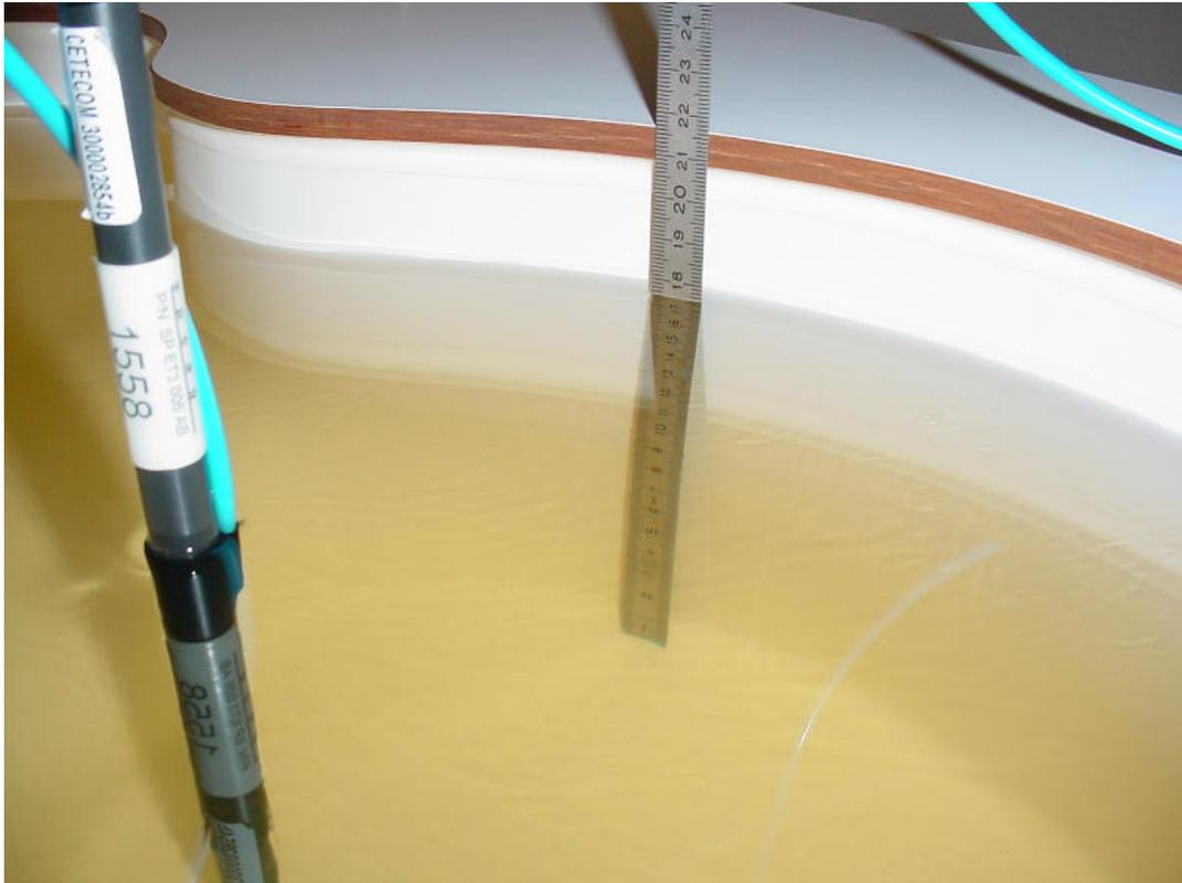
Photo 24: Liquid depth 1900 MHz body tissue simulating liquid
