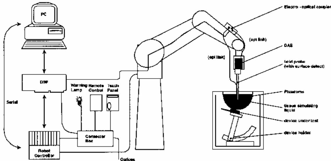
The DAS4 system for performing compliance tests consists of the following items:
