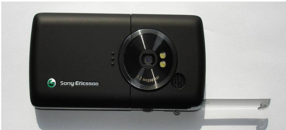
**(b) Back of phone with stylus pen partly pulled out.**
