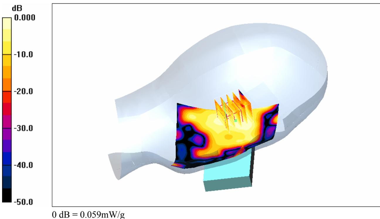
**(j) SAR Distribution for EUT in WLAN mode measured against the left hand side phantom for the tilt phone position.**
