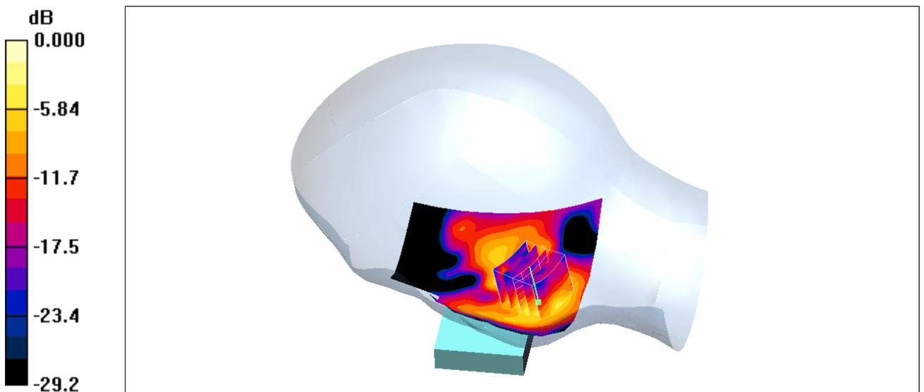
**(g) Maximum SAR Distribution for EUT in WLAN mode measured against the right hand side phantom for the cheek phone position.**
