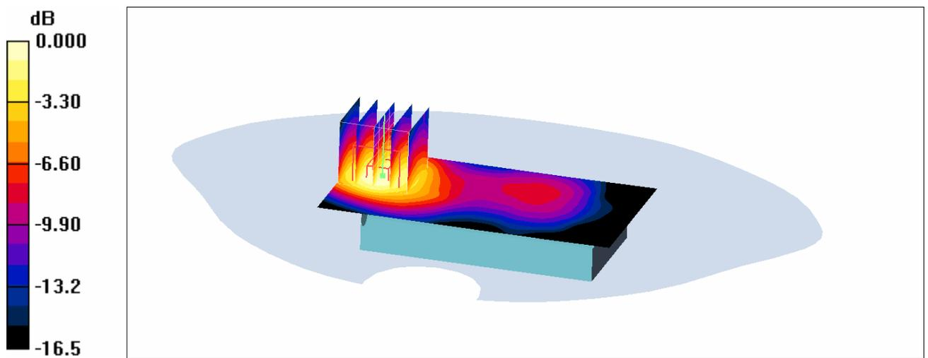
(e) Maximum SAR Distribution for EUT in GSM1900 mode measured with the back of the phone facing the flat section of phantom.
