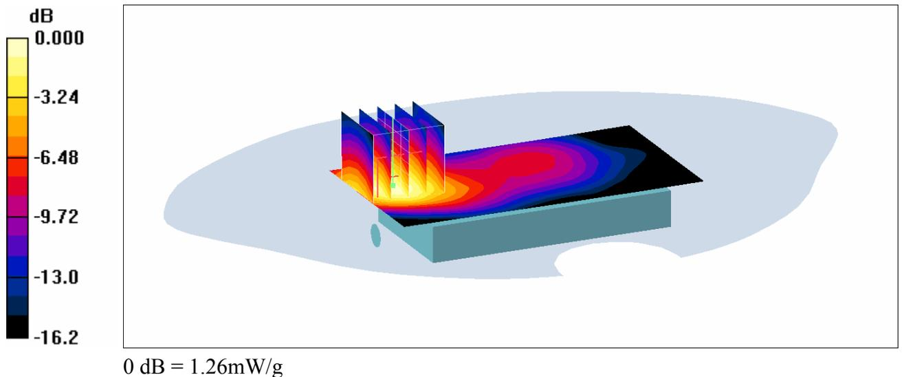
(f) Maximum SAR Distribution for EUT in GPRS(2Tx)1900 mode measured with the back of the phone facing the flat section of phantom.
