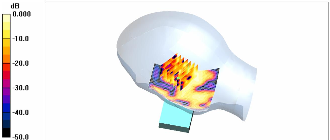
**(h) SAR Distribution for EUT in WLAN mode measured against the right hand side phantom for the tilt phone position.**
