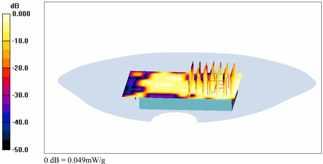
(k) Maximum SAR Distribution for EUT in WLAN mode measured with the back of the phone facing the flat section of phantom.
