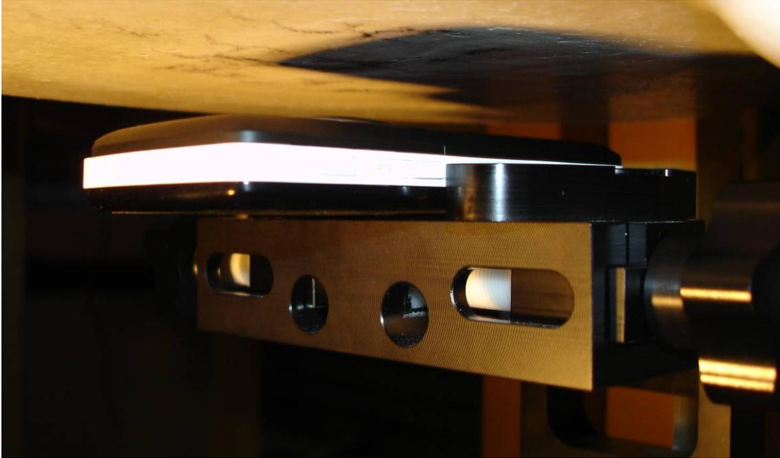
(c) Device on flat section of the phantom. The separation was 15 mm between the device and the flat phantom.
