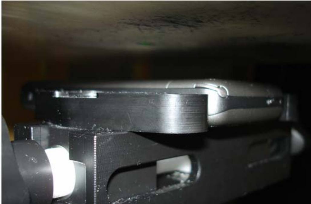
(c) Device on flat section of the phantom. The separation was 15 mm between the device and the flat phantom.
