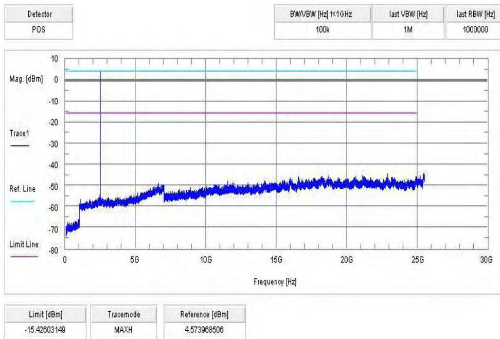
**Plot 7:** lowest channel – 2402 MHz, 8 DPSK modulation
