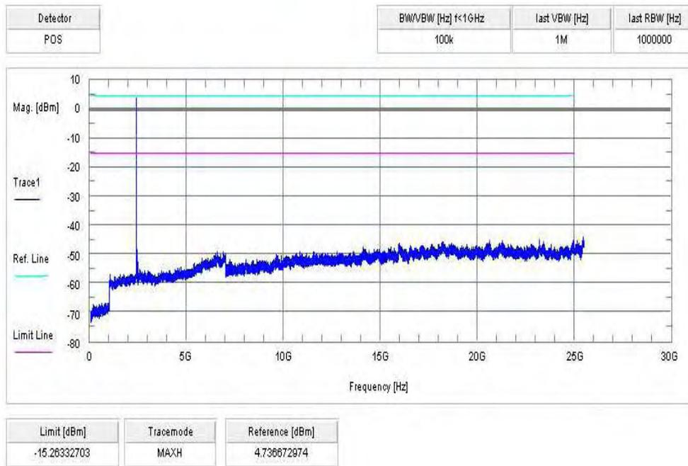
**Plot 8:** middle channel – 2441 MHz, 8 DPSK modulation
