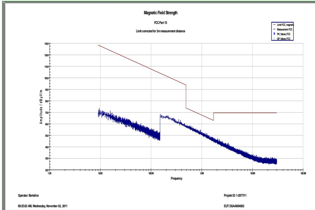
**Plot 2:** 9 kHz to 30 MHz, TX mode, channel 39
