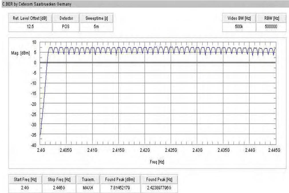
**Plot 2: Number of hopping channels (GFSK modulation)**
