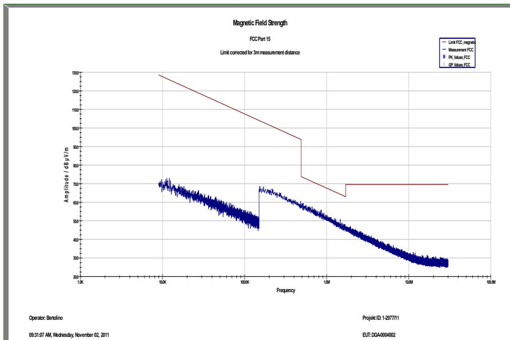
Plot 3: 9 kHz to 30 MHz, TX mode, channel 78
