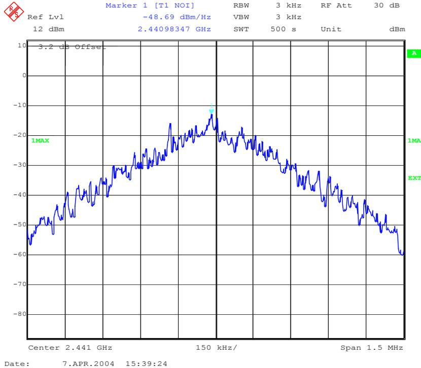
Result: Power density : - 48,69 dBm/Hz = -13,89 dBm / 3 KHz
