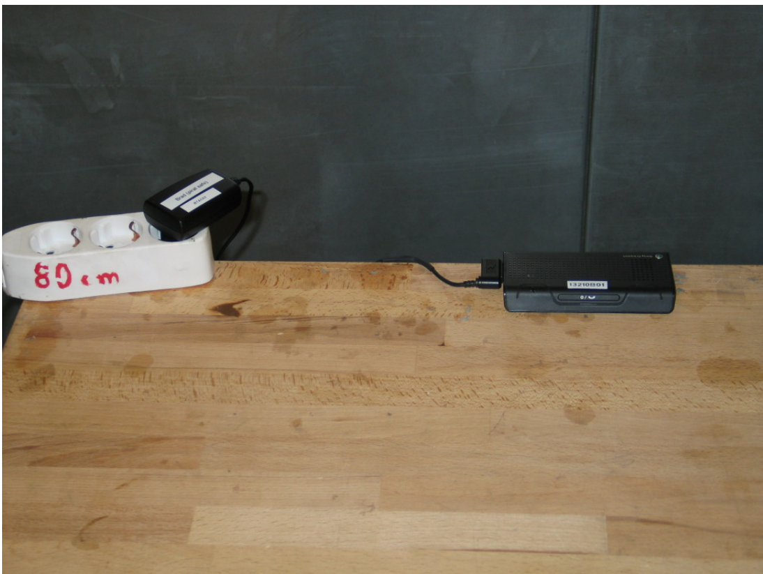
Photo 3: Test setup for conducted measurements (AC Port (power line))
