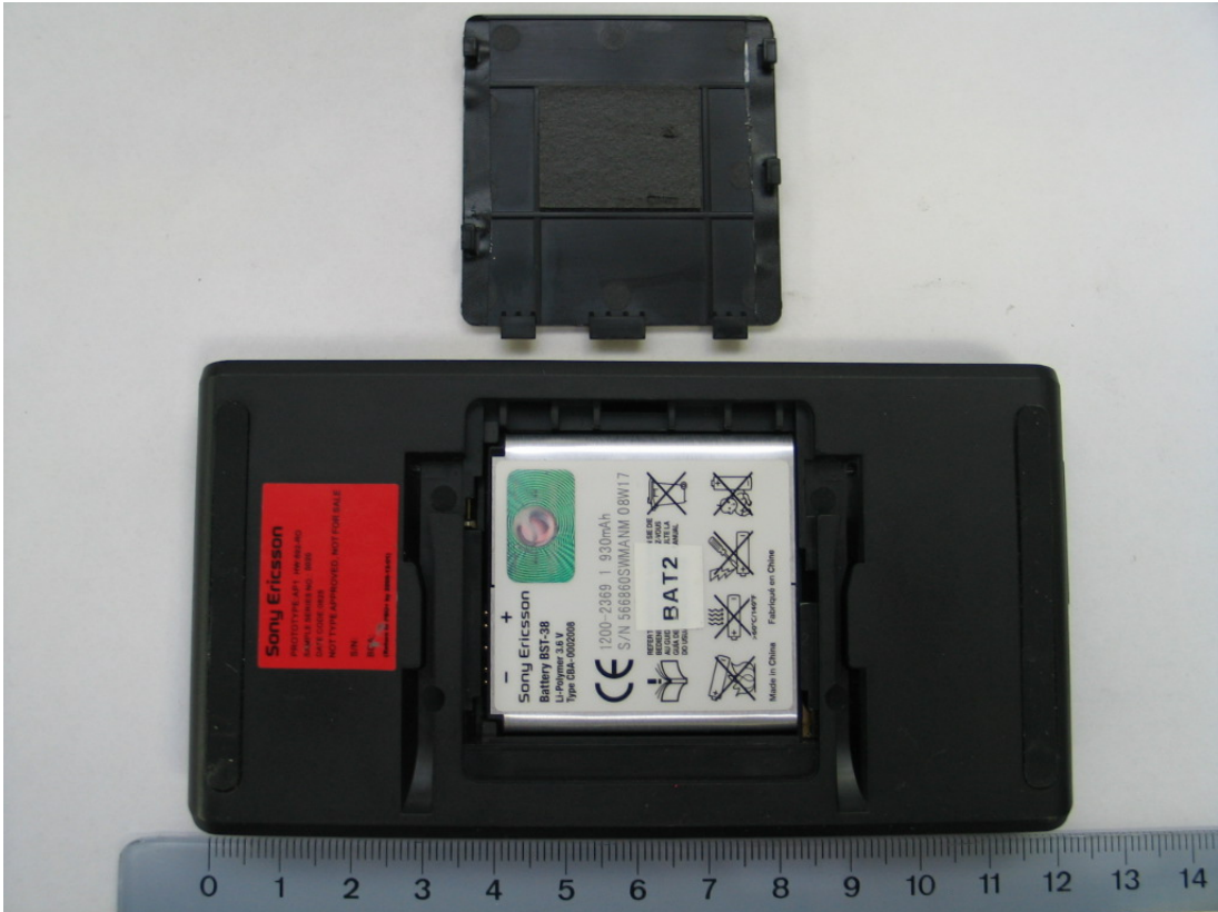
Photo 6: EUT (bottom side, battery cover removed)
