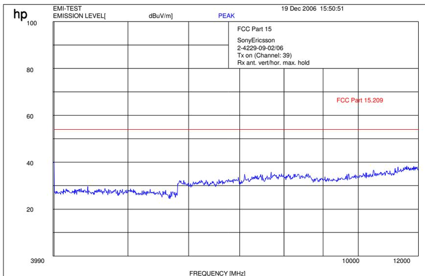
Plot : 0.03 - 4 GHz vertical/horizontal (highest channel)
