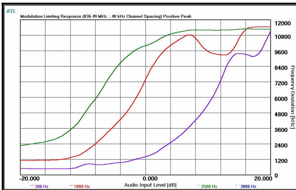
PLOT 12-1: MODULATION CHARACTERISTICS – MODULATION LIMITING: WIDE BAND; POSITIVE PEAK
