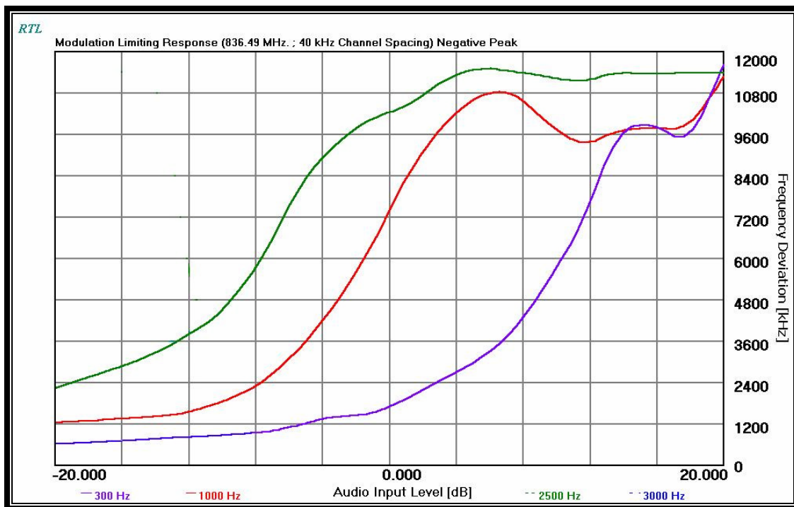
PLOT 12-2: MODULATION CHARACTERISTICS – MODULATION LIMITING: WIDE BAND; NEGATIVE PEAK
