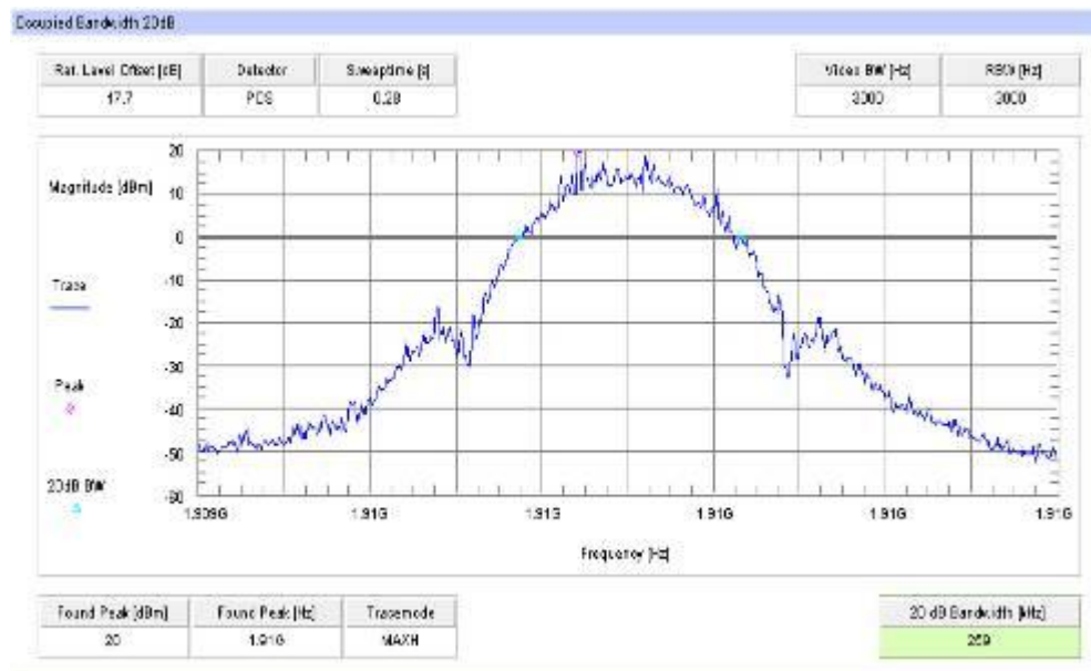
Plot 12: Channel 810 (-26 dBc BW) - EDGE
