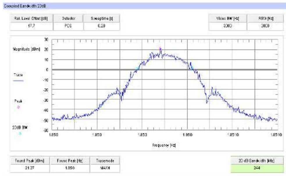
Plot 8: Channel 512 (-26 dBc BW) - EDGE
