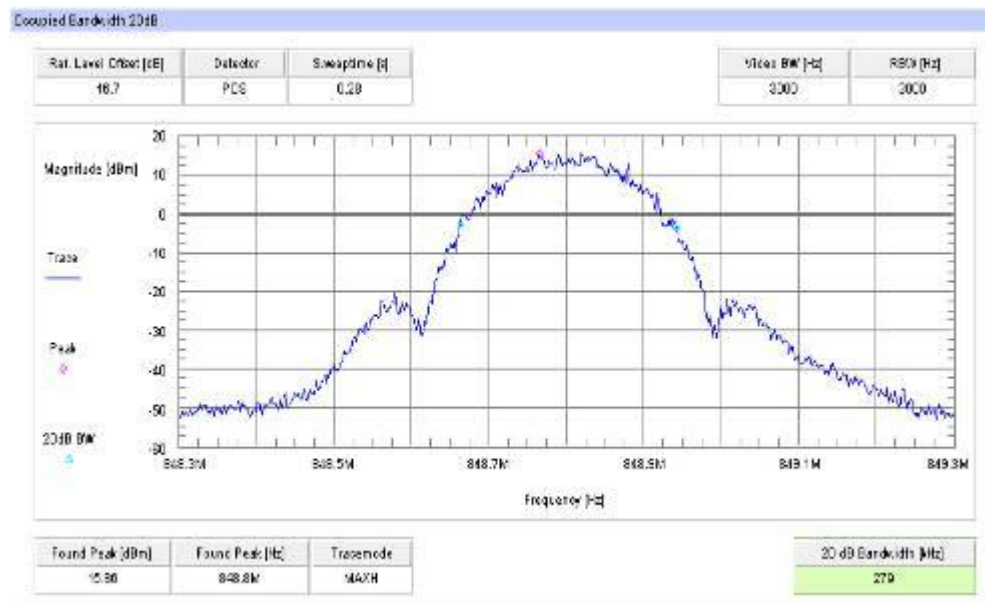
Plot 12: Channel 251 (-26 dBc BW) - EDGE
