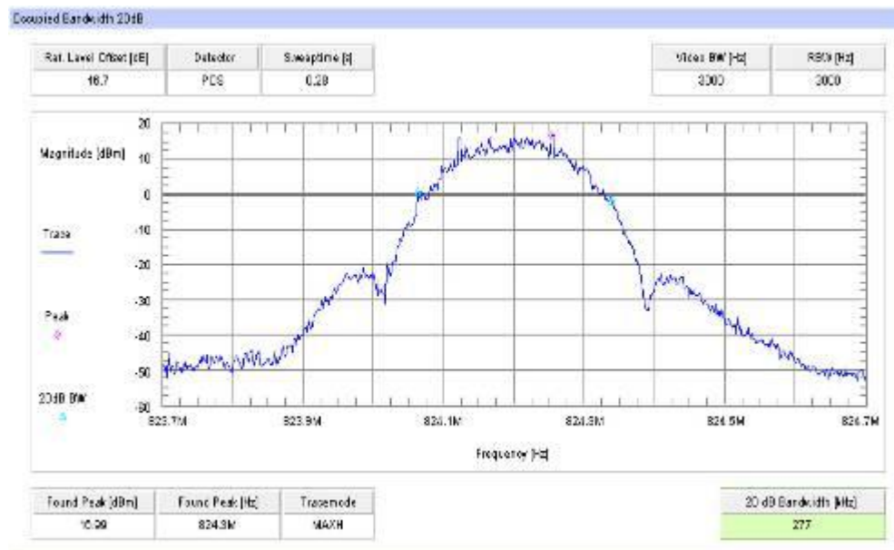
Plot 8: Channel 128 (-26 dBc BW) - EDGE
