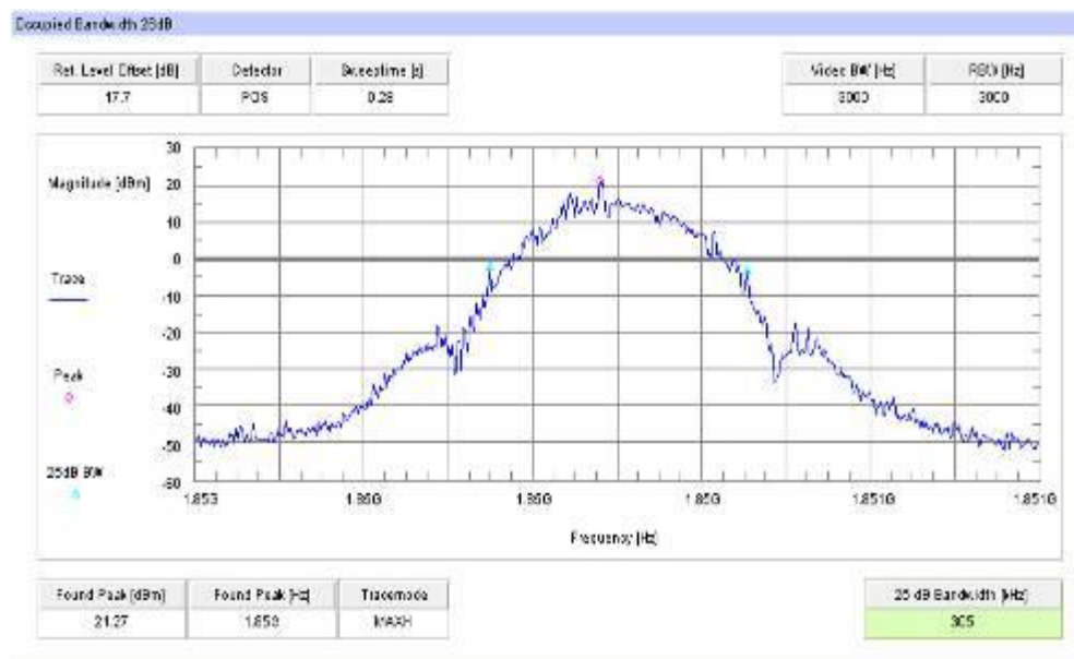
Plot 8: Channel 512 (-26 dBc BW) - EDGE
