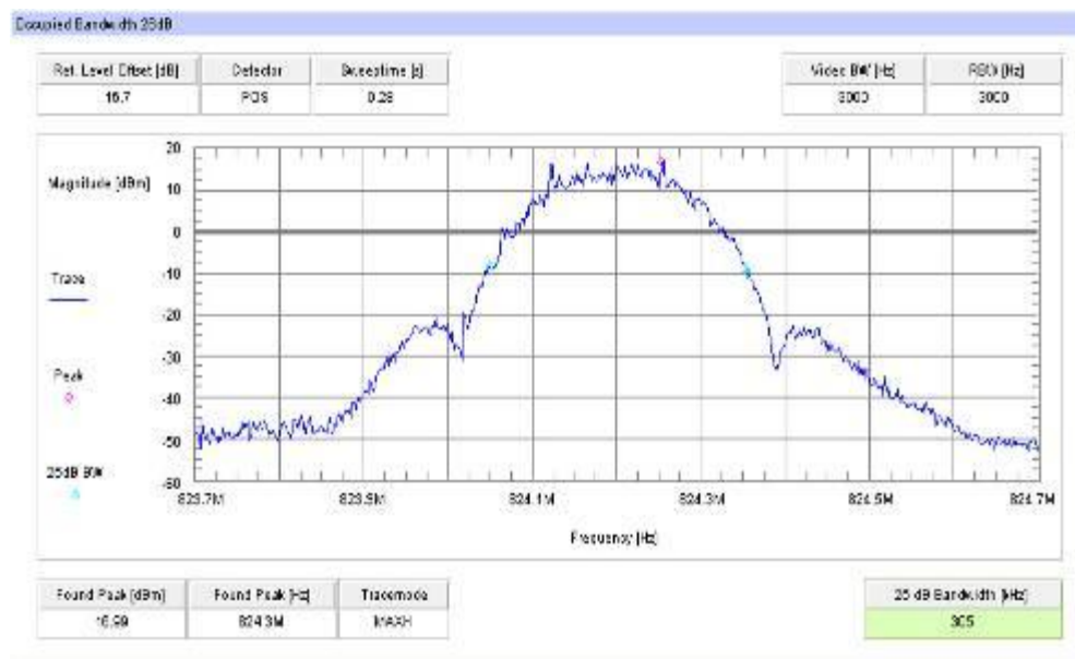
Plot 8: Channel 128 (-26 dBc BW) - EDGE
