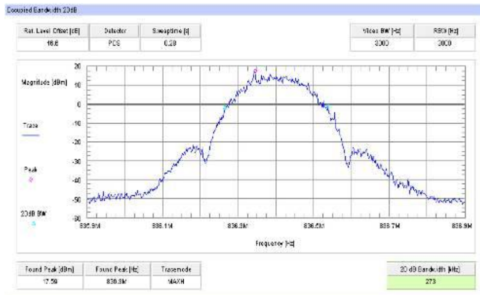
Plot 10: Channel 189 (-26 dBc BW) - EDGE
