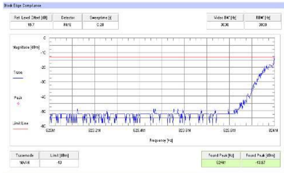
Plot 2: Channel 251 (GSM-mode)
