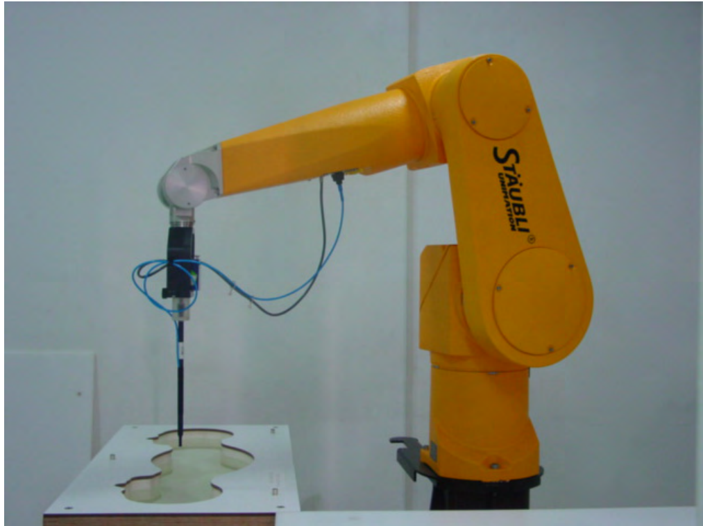
Picture B1: Specific Absorption Rate Test Layout
