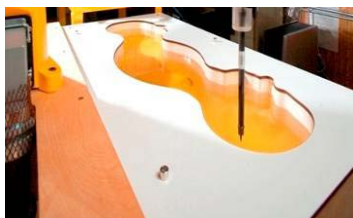
Figure 6-2 SAM Phantom with Simulating Tissue
