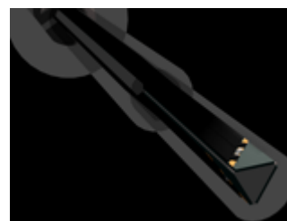
Figure 4-3 Triangular Probe Configuration
