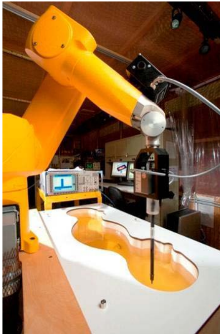
Figure 3-2 SAR Measurement System
