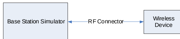
Figure 14-1 Power Measurement Setup
