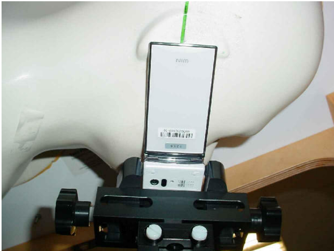
Photo 20: Test position right hand tilted 15°
