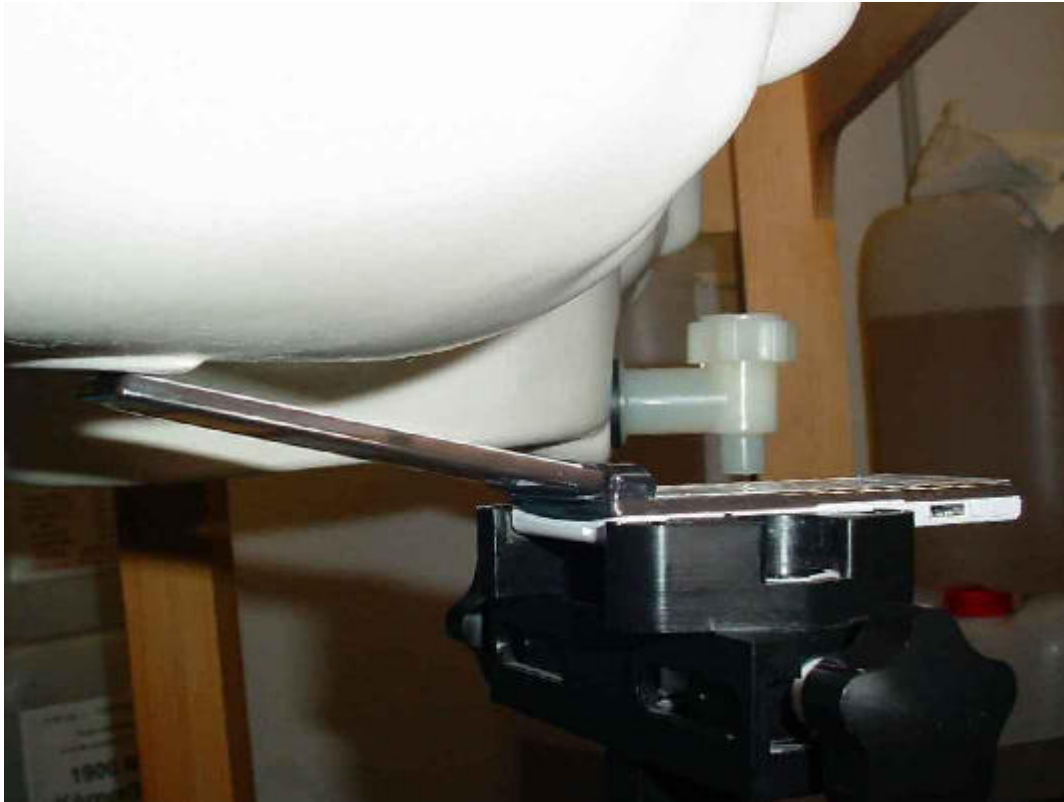
Photo 22: Test position body worn front side (15 mm distance)
