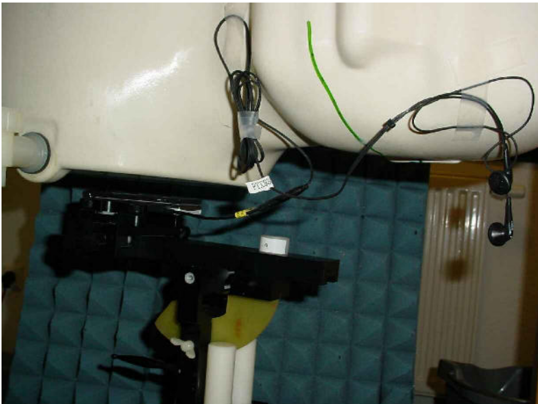
Photo 22: Test position body worn front side (15 mm distance)
