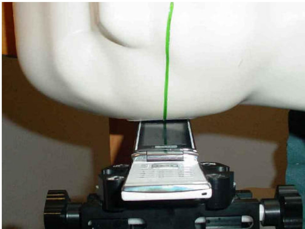
Photo 20: Test position right hand tilted 15°
