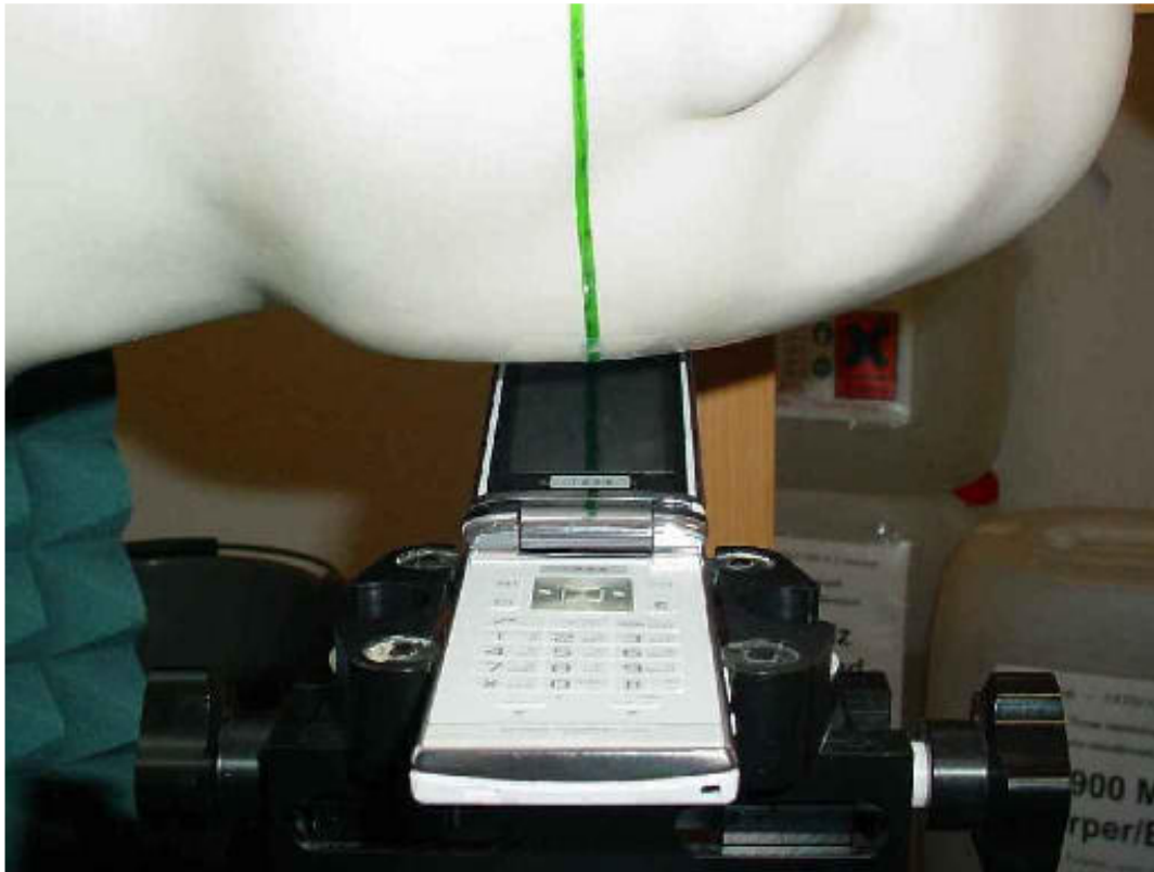
Photo 16: Test position left hand tilted 15°
