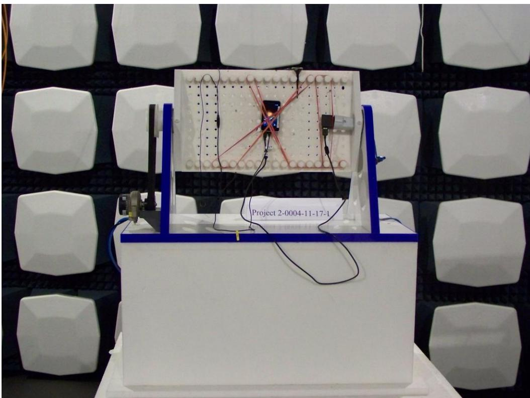
**Photograph 2:** Radiated emission measurements in anechoic chamber
