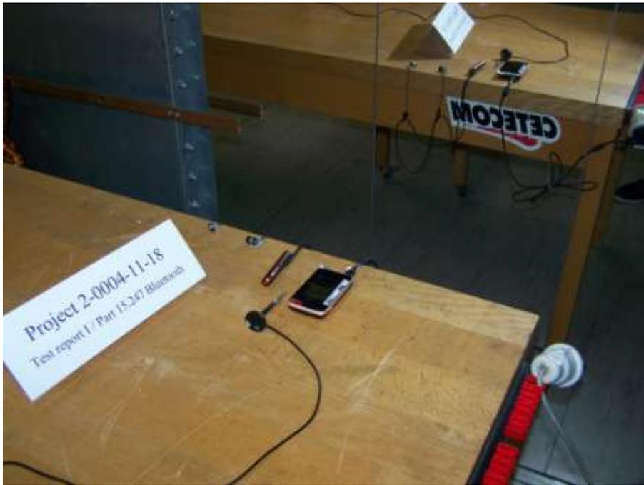
Photograph 3: Conducted test set-up, emissions on AC-mains
