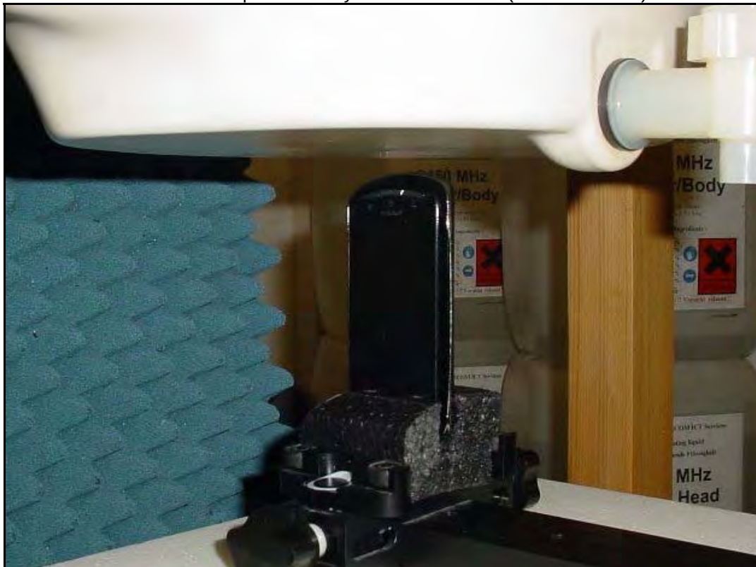
Photo 34: Test position body worn bottom side (10mm distance)
