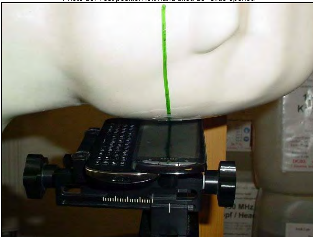
Photo 18: Test position left hand tilted 15° slide opened
