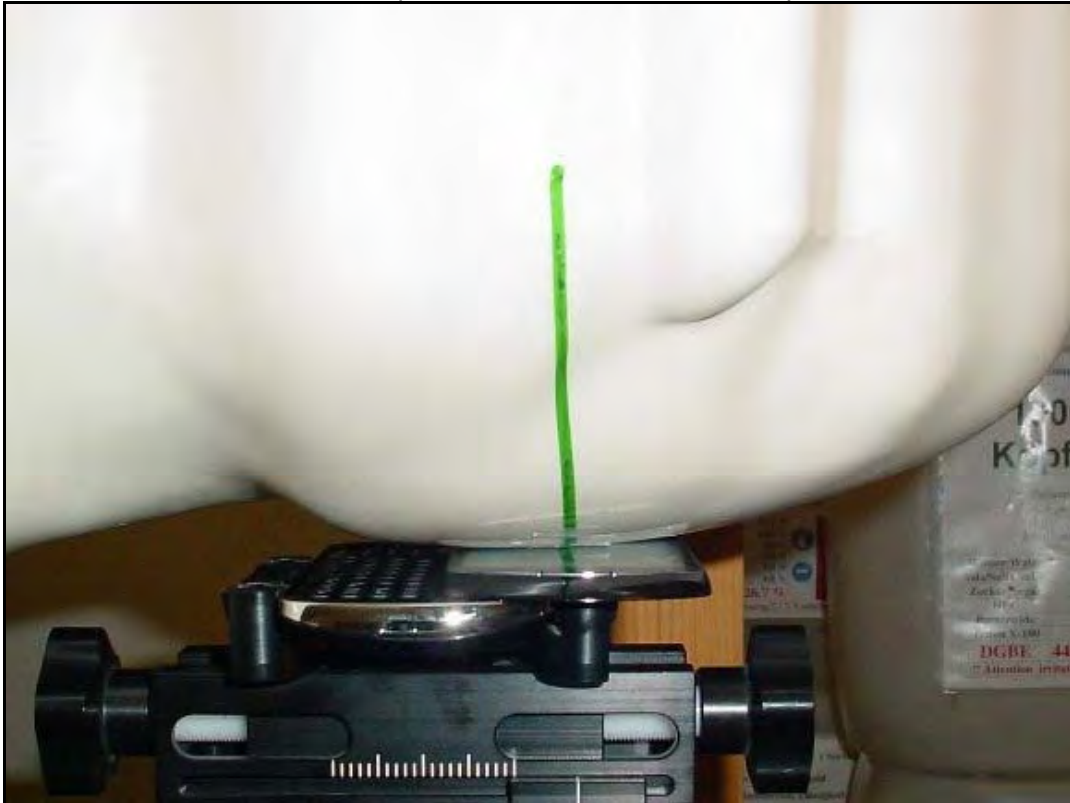
Photo 16: Test position left hand touched slide opened
