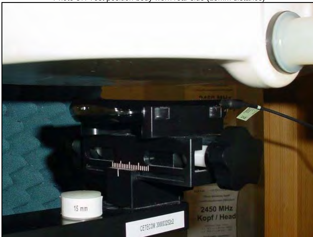
Photo 37: Test position body worn rear side (15mm distance)
