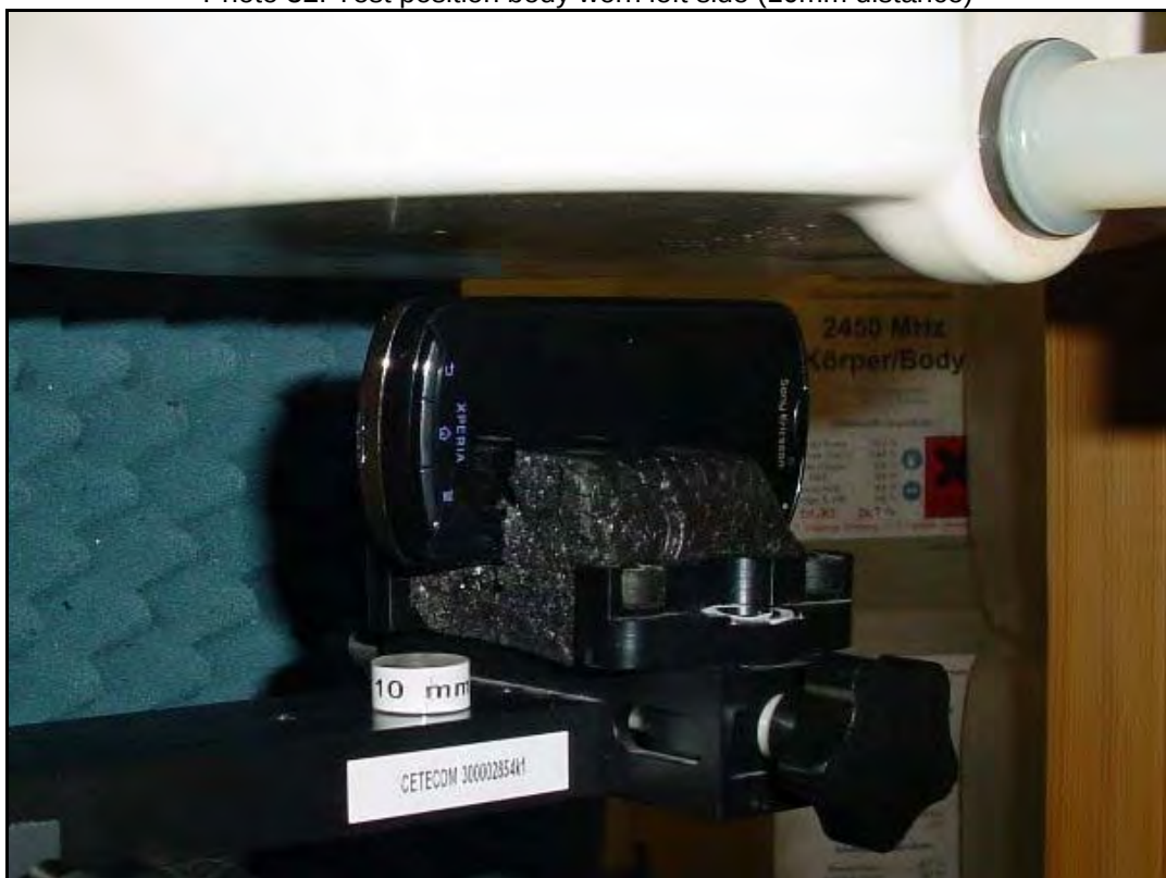
Photo 32: Test position body worn left side (10mm distance)
