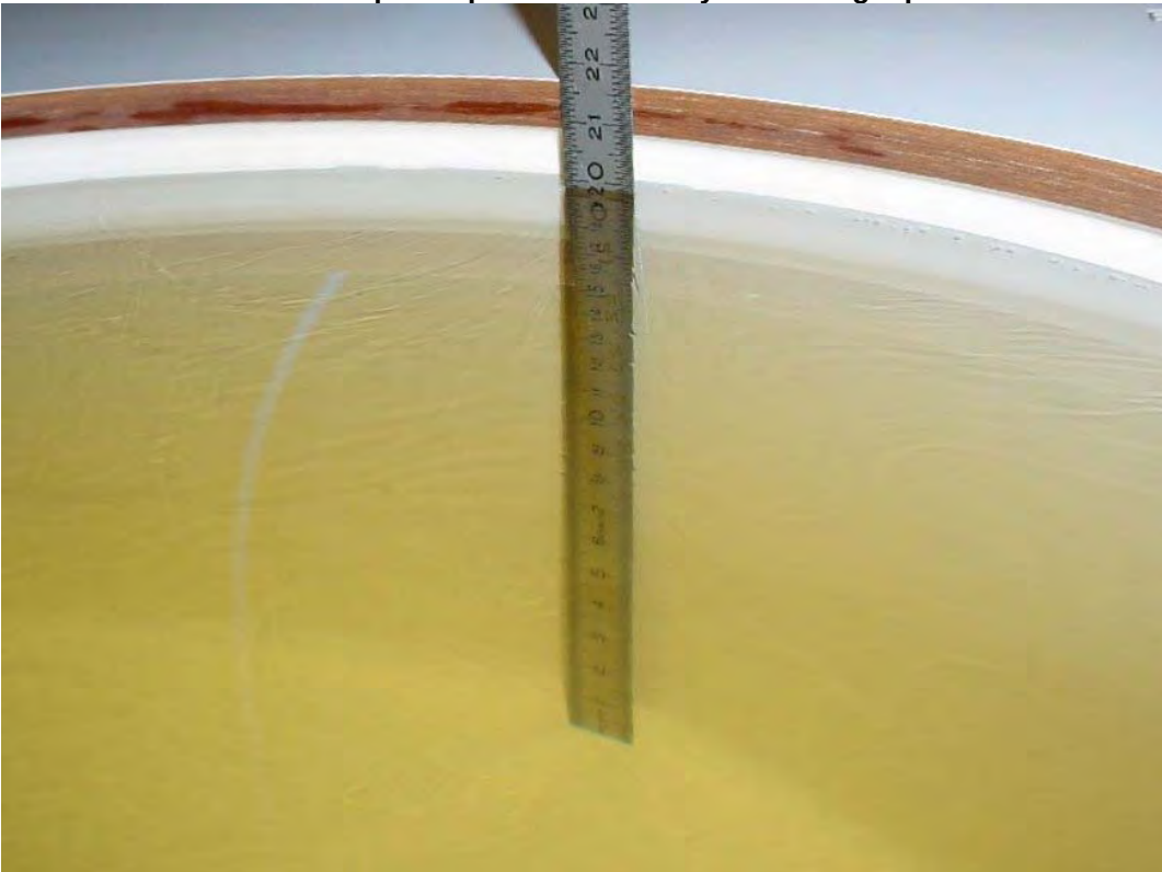
Photo 2: Liquid depth 850 MHz body simulating liquid
