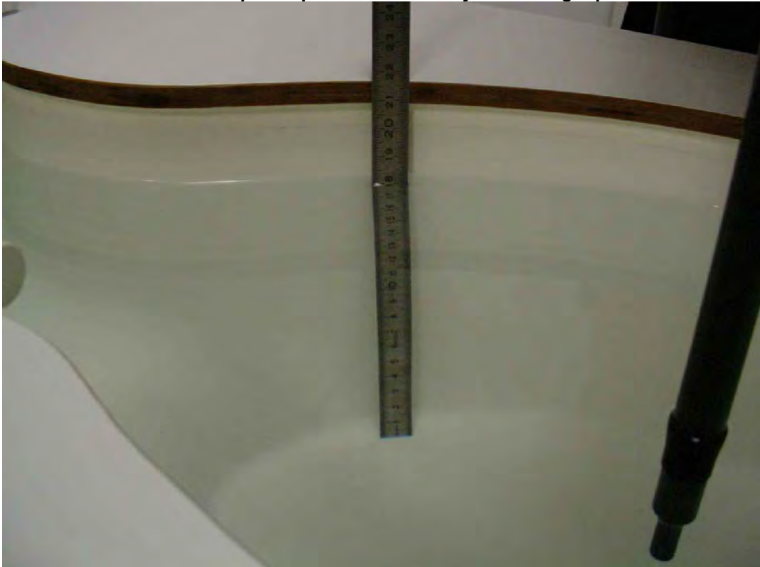
Photo 6: Liquid depth 2450 MHz body simulating liquid
