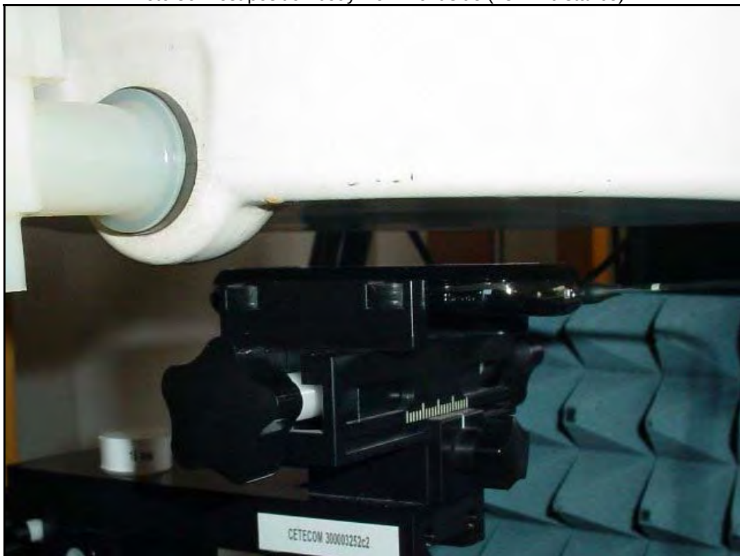
Photo 36: Test position body worn front side (15mm distance)
