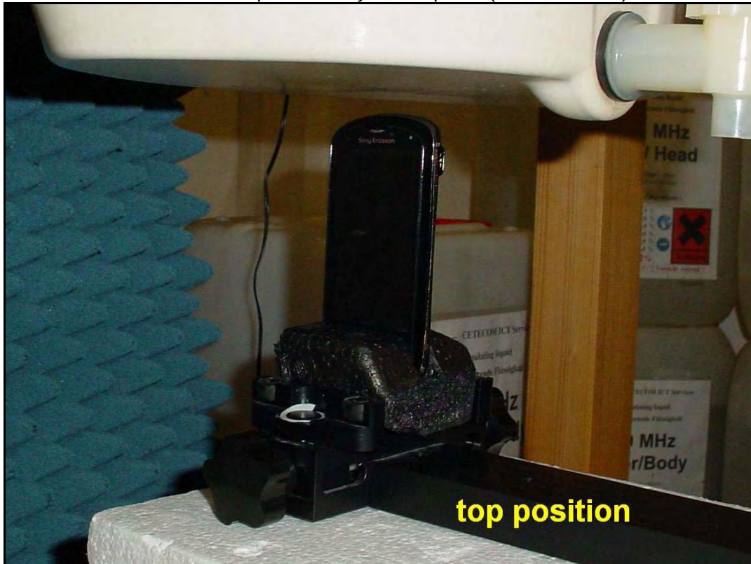
Photo 36: Test position body worn front side (15mm distance)
