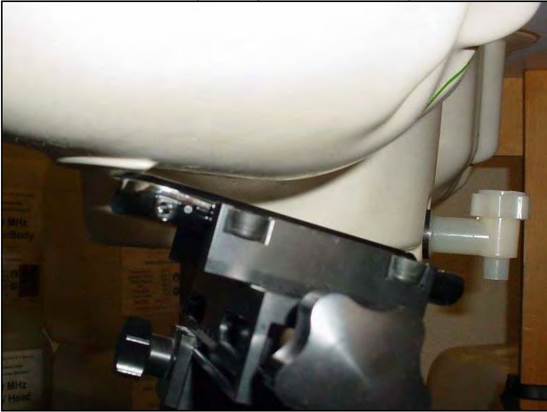
Photo 30: Test position body worn front side (10mm distance)
