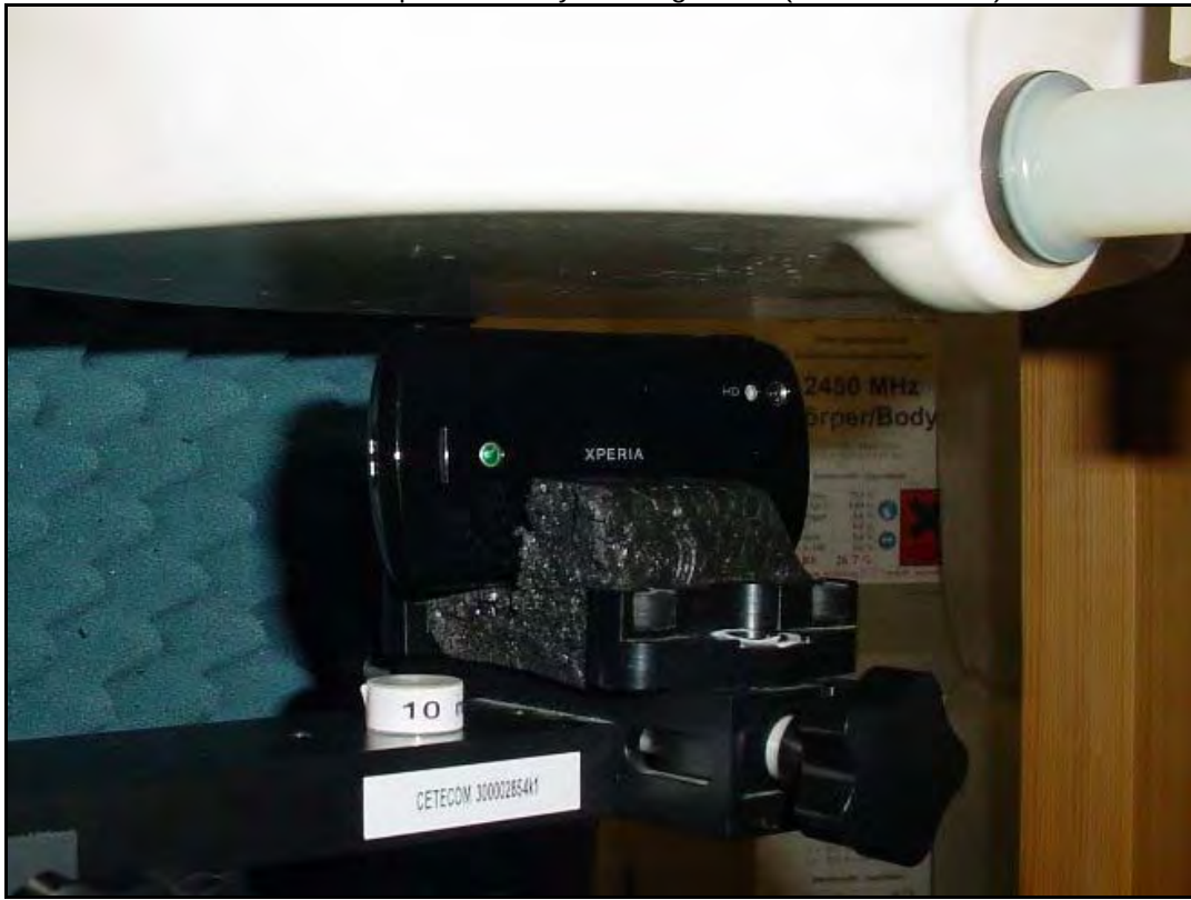
Photo 34: Test position body worn bottom side (10mm distance)
