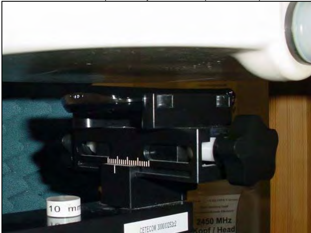
Photo 32: Test position body worn left side (10mm distance)
