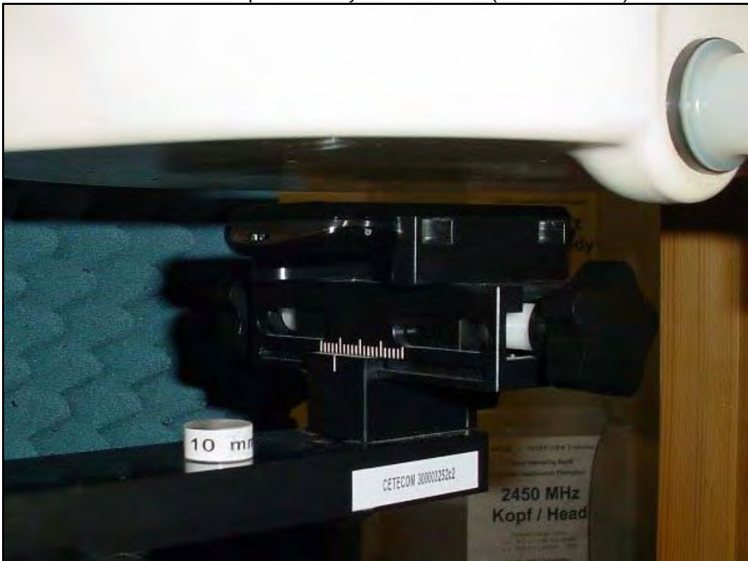
Photo 30: Test position body worn front side (10mm distance)
