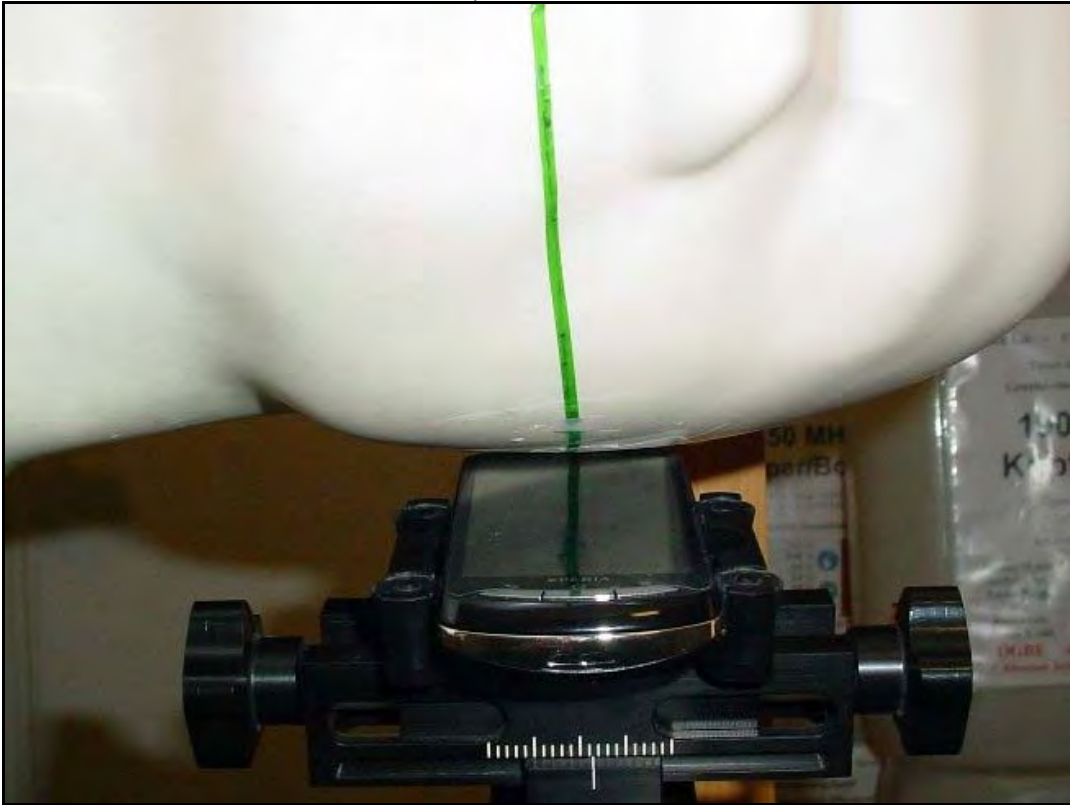
Photo 14: Test position left hand tilted 15°
