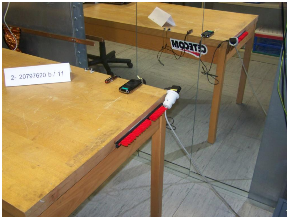
Measurement of conducted emissions on AC-mains
