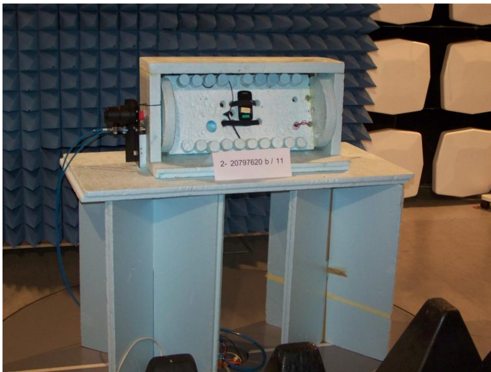
Measurement of radiated field strength
