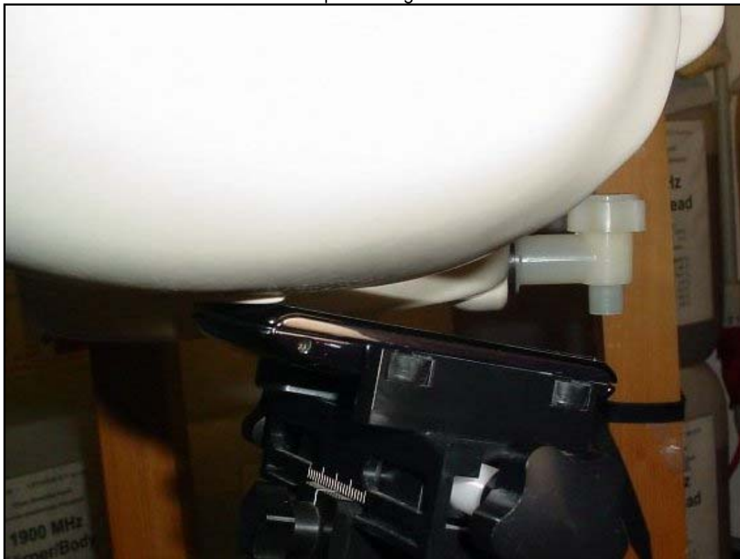
Photo 20: Test position body worn front side (10 mm distance)
