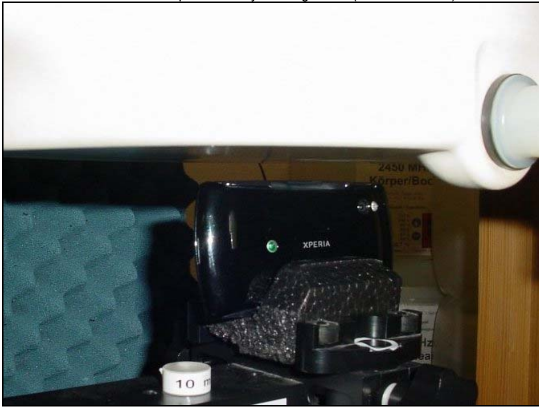
Photo 24: Test position body worn bottom edge side (10 mm distance)
