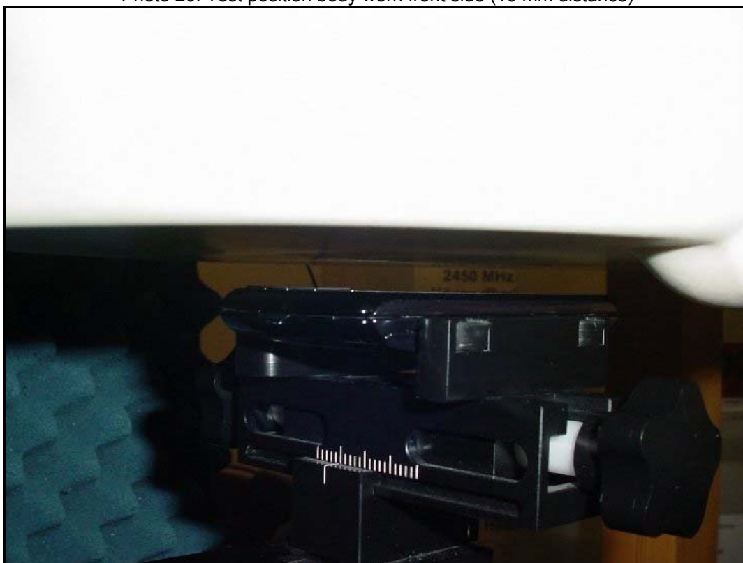
Photo 20: Test position body worn front side (10 mm distance)
