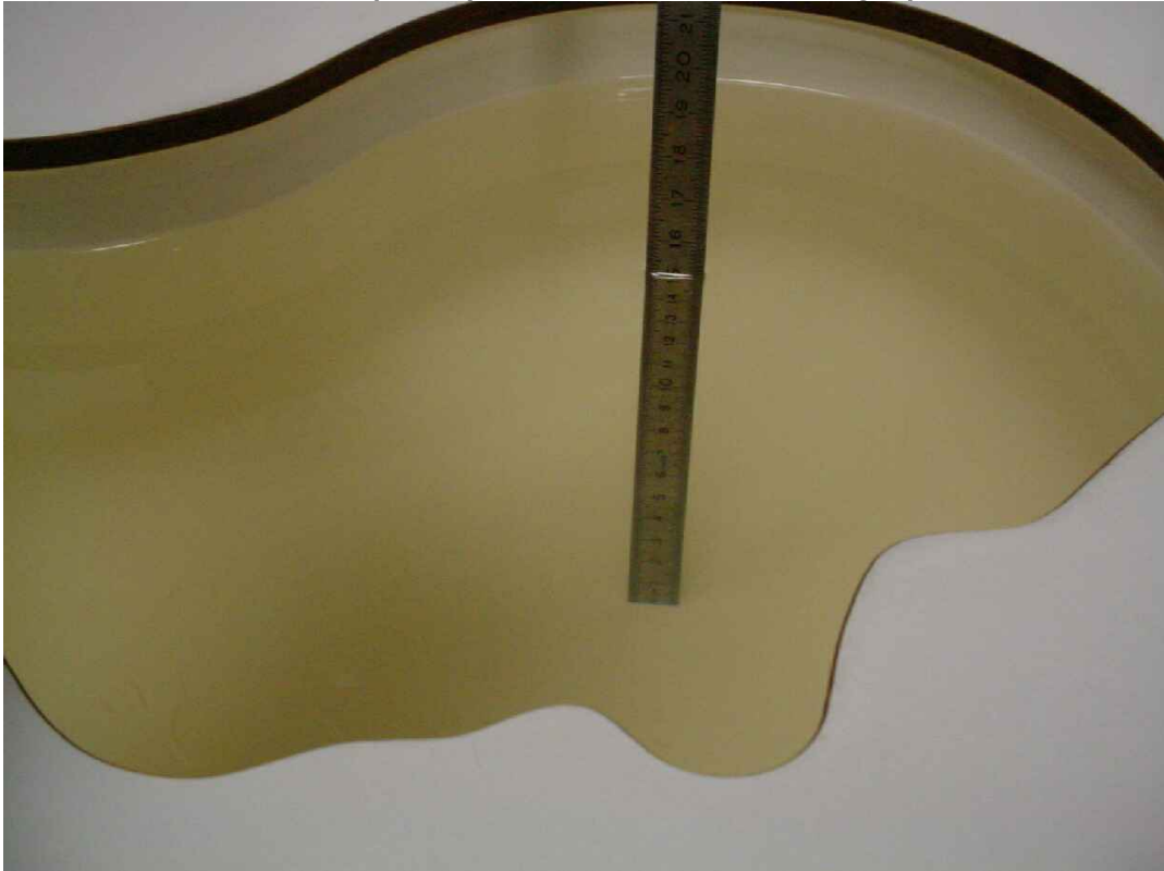
Photo 6: Liquid depth 2450 MHz body simulating liquid
