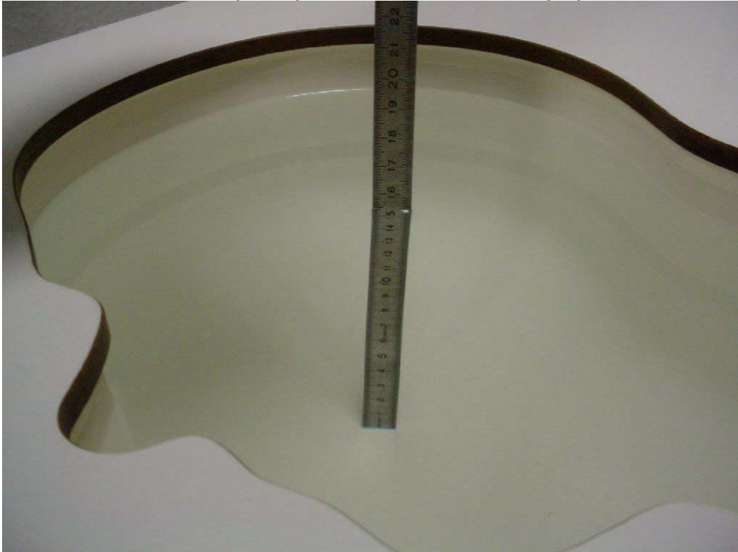
Photo 4: Liquid depth 1900 MHz body simulating liquid
