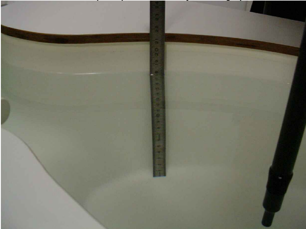
Photo 6: Liquid depth 2450 MHz body simulating liquid
