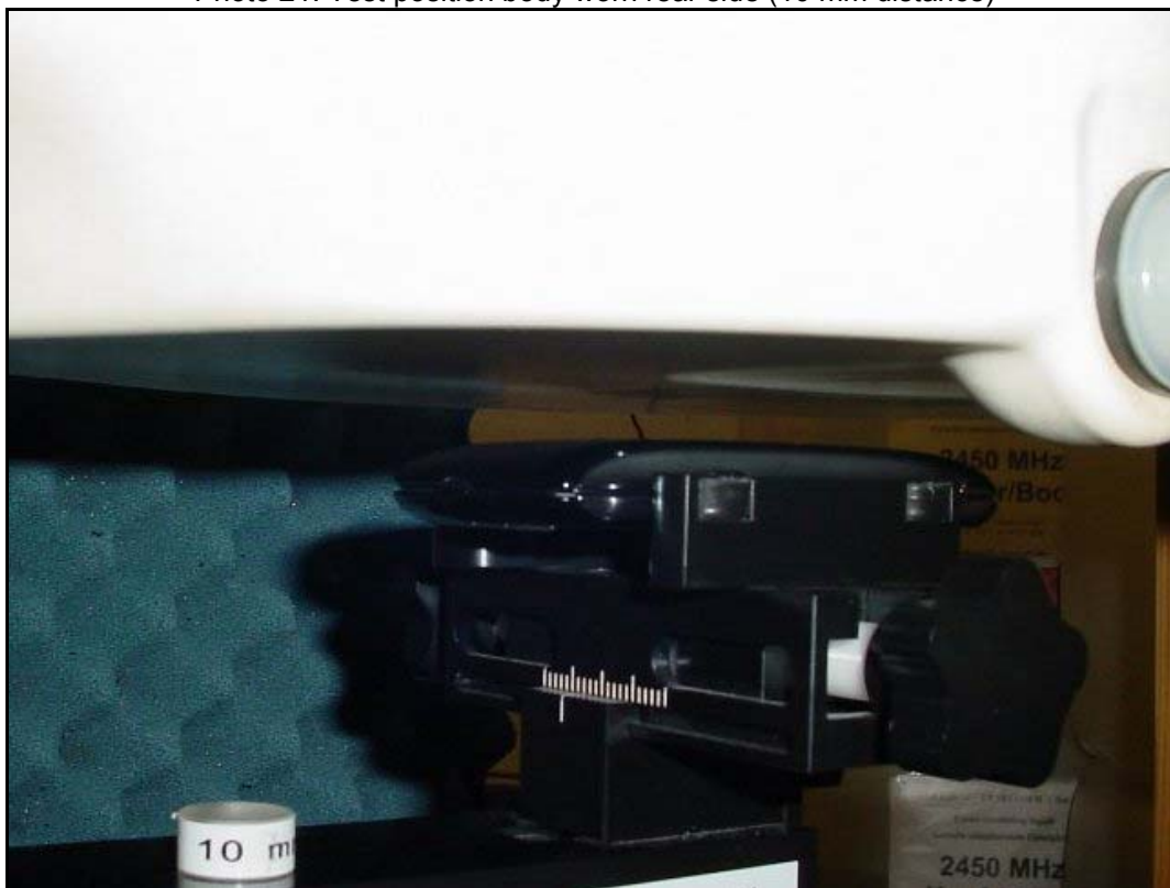
Photo 22: Test position body worn left side (10 mm distance)
