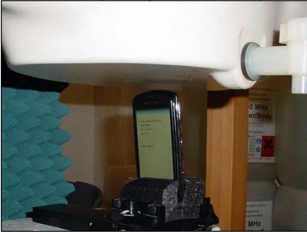
Photo 26: Test position body worn rear side (15 mm distance) with headset
