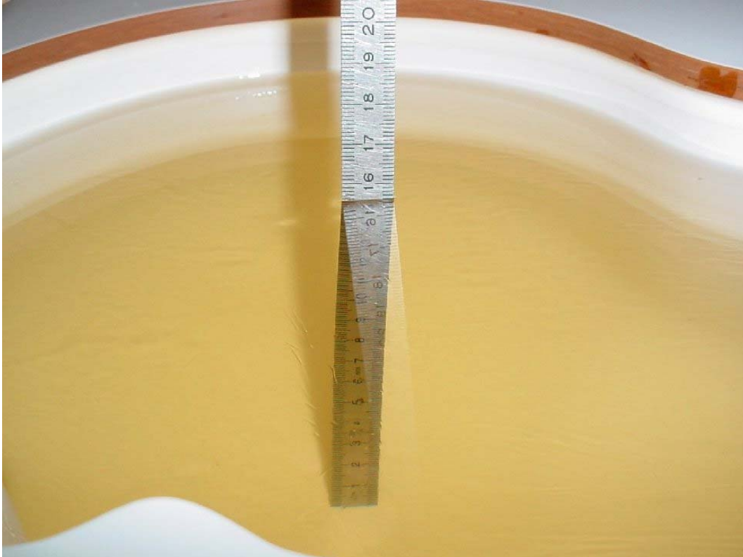
Photo 2: Liquid depth 850 MHz body simulating liquid
