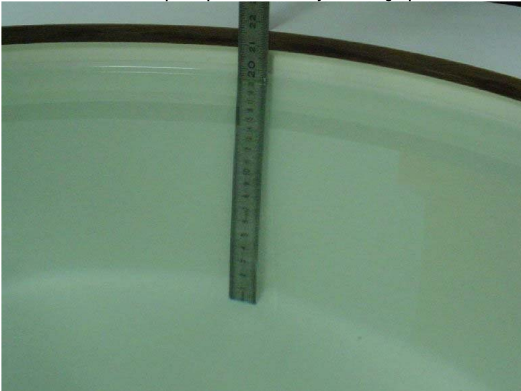
Photo 4: Liquid depth 1900 MHz body simulating liquid
