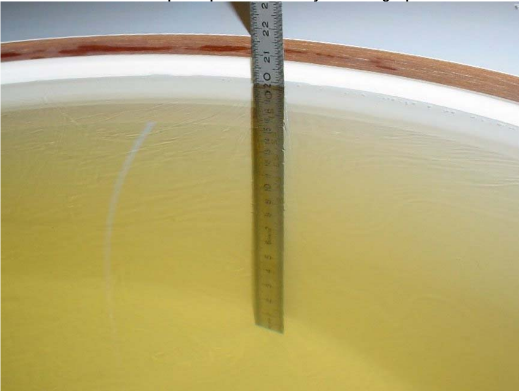
Photo 2: Liquid depth 850 MHz body simulating liquid
