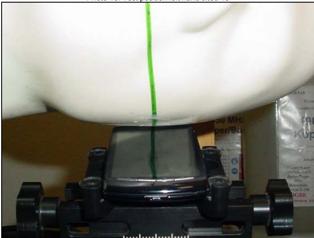
Photo 14: Test position left hand tilted 15°
