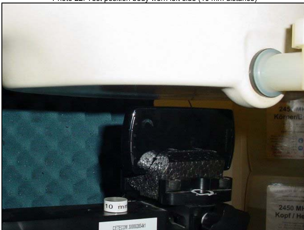
Photo 22: Test position body worn left side (10 mm distance)
