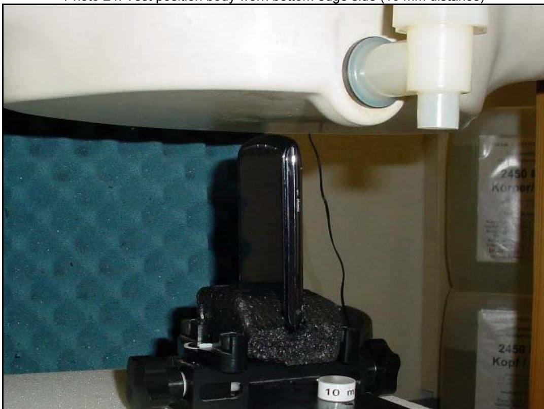
Photo 24: Test position body worn bottom edge side (10 mm distance)
