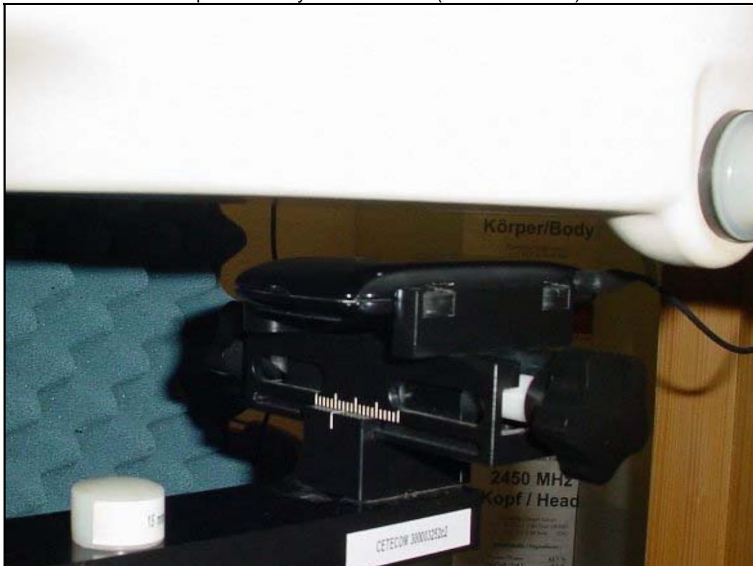
Photo 26: Test position body worn rear side (15 mm distance) with headset
